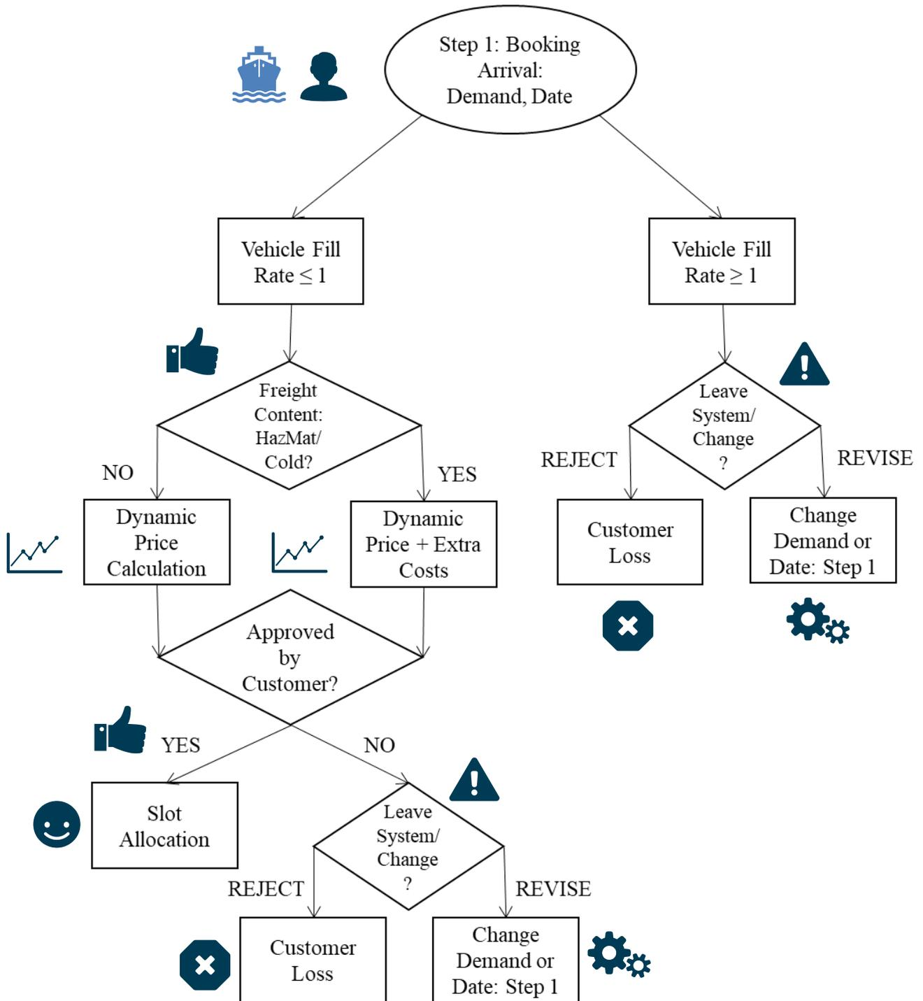
**Figure 4.8:** Flowchart of Dynamic Pricing and Slot Allocation in Multimodal Freight Network
