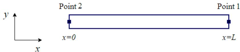
Figure 3.4. A beam element with free-free end conditions
