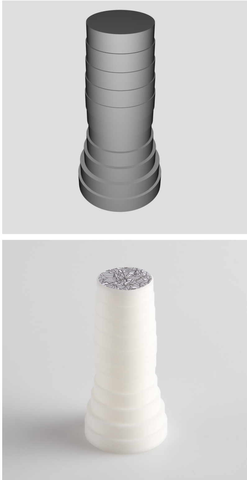
Figure 7.2: Generated 3D mesh and fabricated actual model
