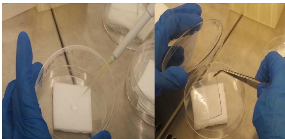
Figure 7: Inoculation of the test specimen with E. coli according to ISO 22196 test procedure
