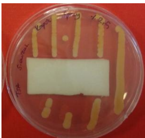
Figure 16: Agar plate showing the inhibition of the bacterial growth in the antimicrobial specimens' surrounding area.
