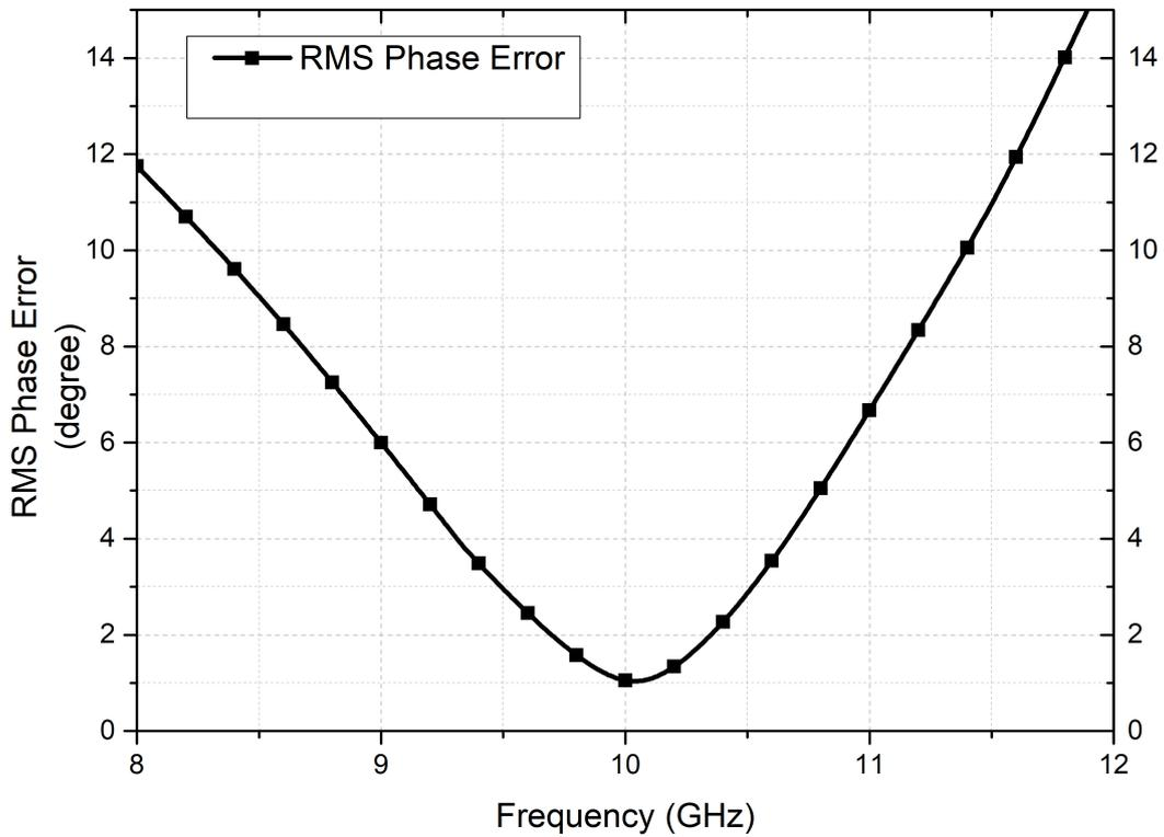
**Figure 46:** Simulation result of the RMS phase error of the designed phase shifter
