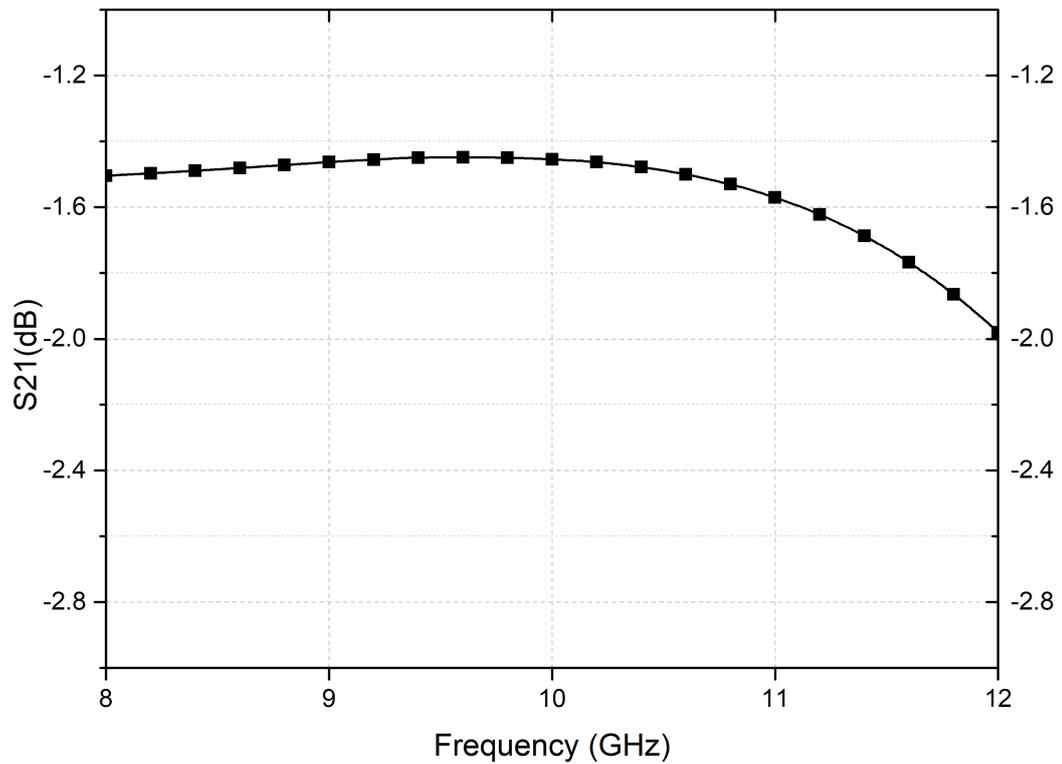
**Figure 30:** Simulation result of the insertion-loss of the SP4T
