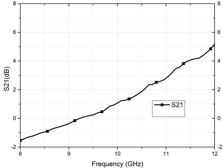
**Figure 67:** S21 measurement results of designed second active gain-equalizer
