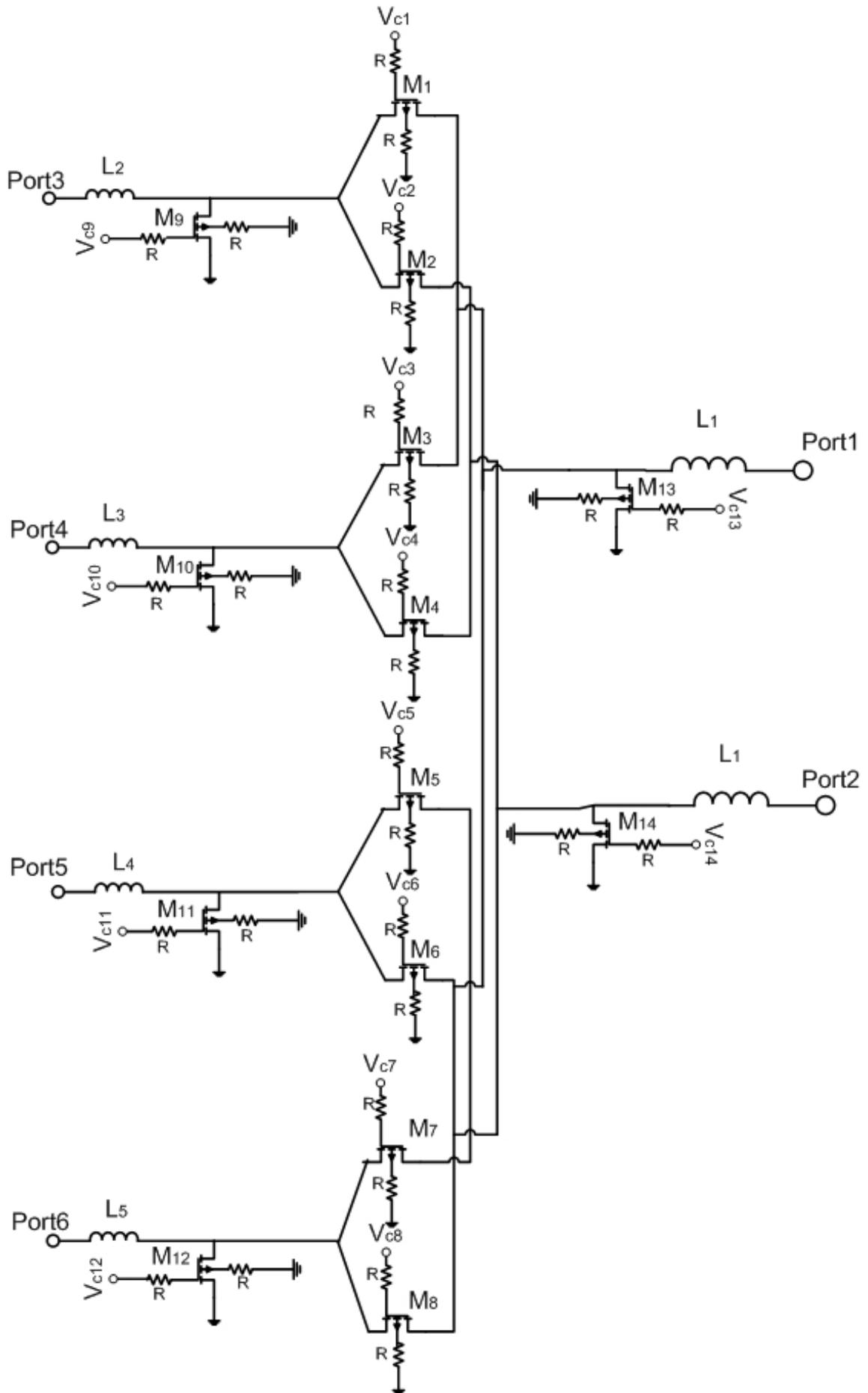
Figure 32: Schematic of the DP4T
