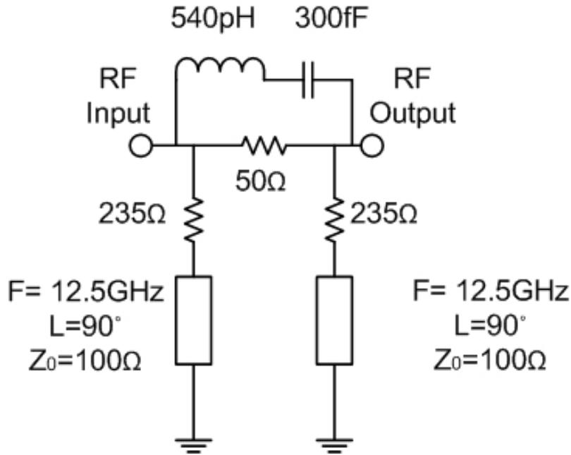
**Figure 53:** The schematic of designed conventional type gain-equalizer
