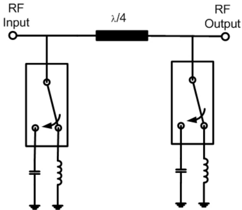
**Figure 16:** General diagram of the bit of the loaded-line phase shifter
