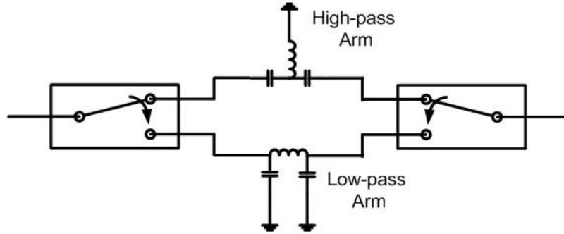
**Figure 22:** Schematic view of high-pass/low pass type phase shifter
