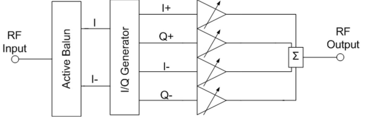
**Figure 20:** Block diagram of a typical vector sum type phase shifter
