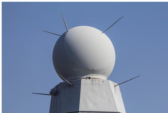
**Figure 7:** Active phased array example: SAMPSON[4]
