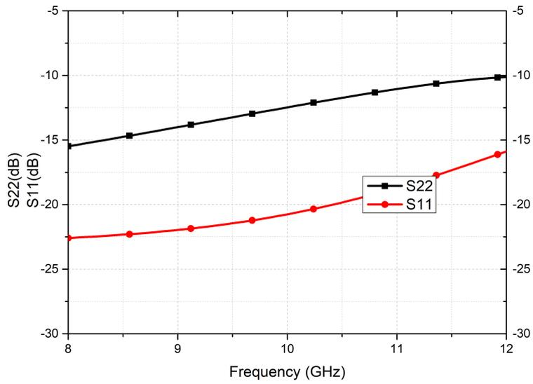
**Figure 61:** S11 and S22 measurement results of designed compact type gain-equalizer for TX chain
