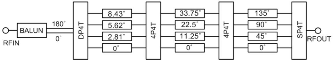
**Figure 24:** Block diagram of 7-bit passive phase shifter
