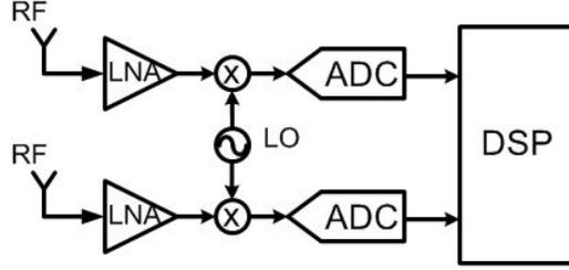
**Figure 11:** Digital beam forming Phased array architectures
