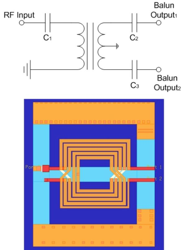
**Figure 25:** Schematic and Layout of the Transformer
