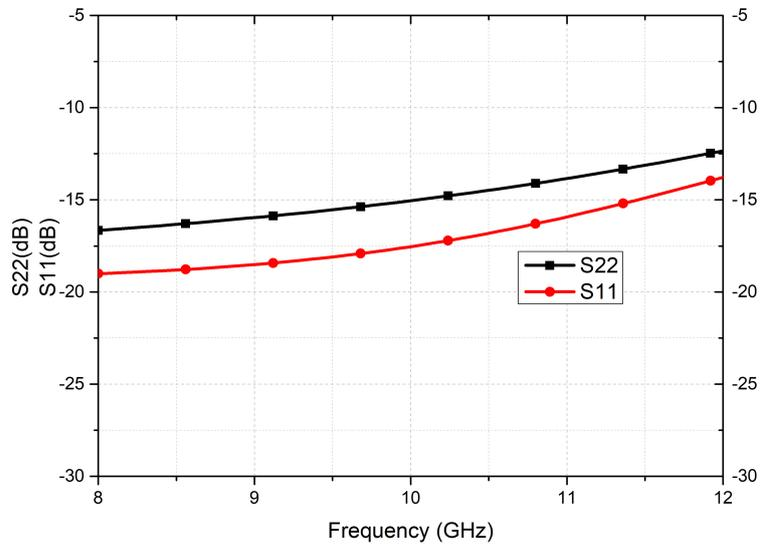
**Figure 59:** S11 and S22 measurement results of designed compact type gain-equalizer for RX chain
