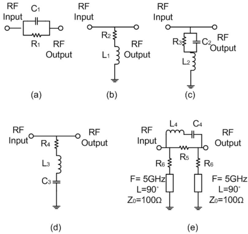
Figure 50: Examples of the schematic of passive gain-equalizers
