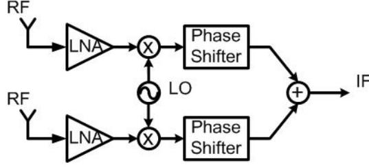
**Figure 9:** IF phase shifting Phased array architectures
