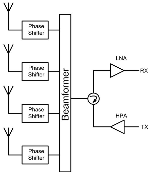
**Figure 4:** Block diagram of passive phased array
