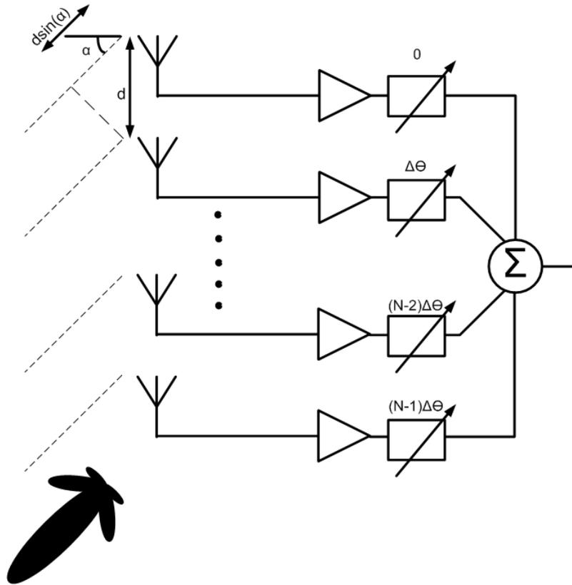
**Figure 2:** Basic receiver block diagram of a phased array system
