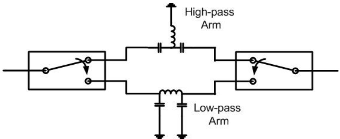
Figure 18: Switched-filter topology with tee networks
