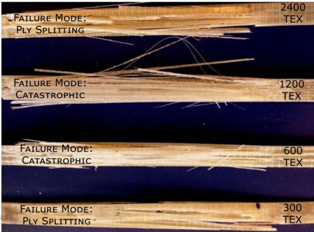
Figure 2.8 Failure modes and images of unidirectional laminated composites after failure.
