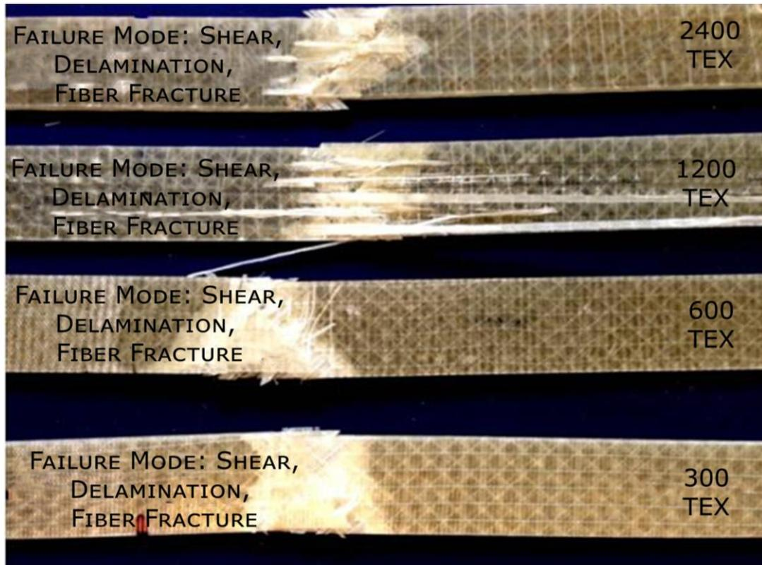
Figure 2.49 Failure modes and images of quasi-isotropic laminated composites after failure.
