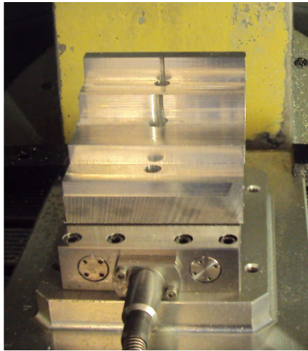
Figure 3.34. Test set-up: dynamometer mounted on machine tool table, workpiece mounted on dynamometer
