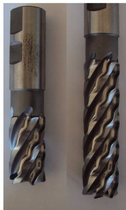
Figure 1.4. End mills with harmonically varying helix angles
