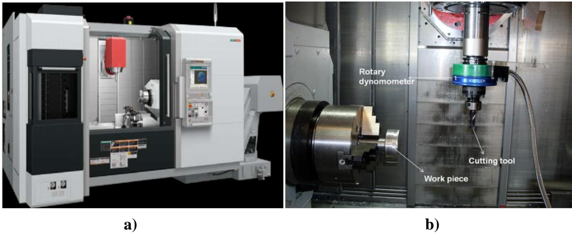
Figure 3-10: a) Mori Seiki NTX 2000 machine tool b) Experimental setup for cutting force measurements
