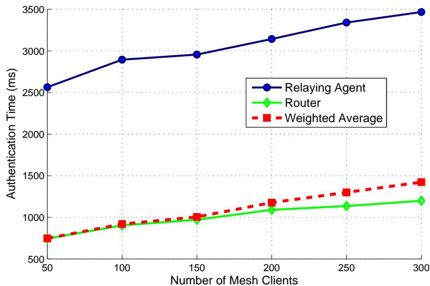
Figure 5.2: Authentication Times at 80-bit Security Level
