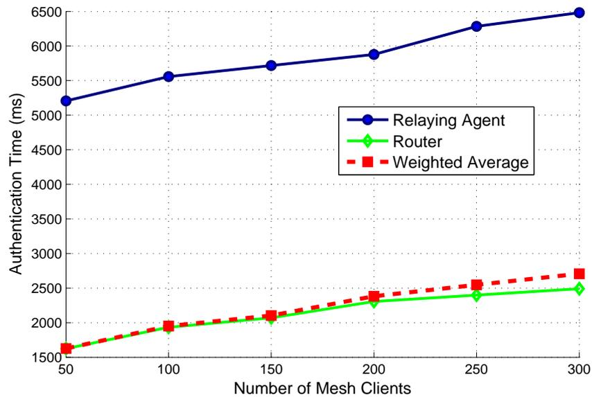
Figure 5.9: Authentication Times at 128-bit Security Level
