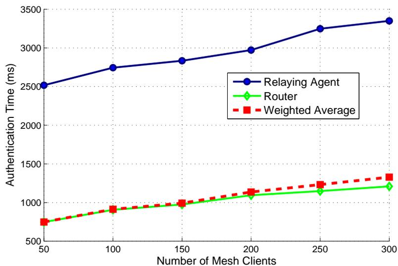
Figure 5.8: Authentication Times at 80-bit Security Level
