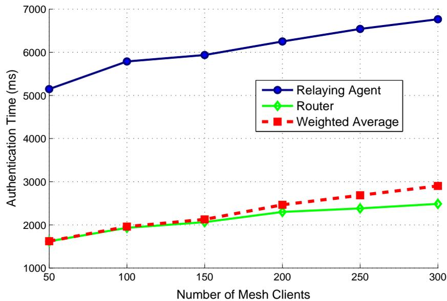
Figure 5.3: Authentication Times at 128-bit Security Level
