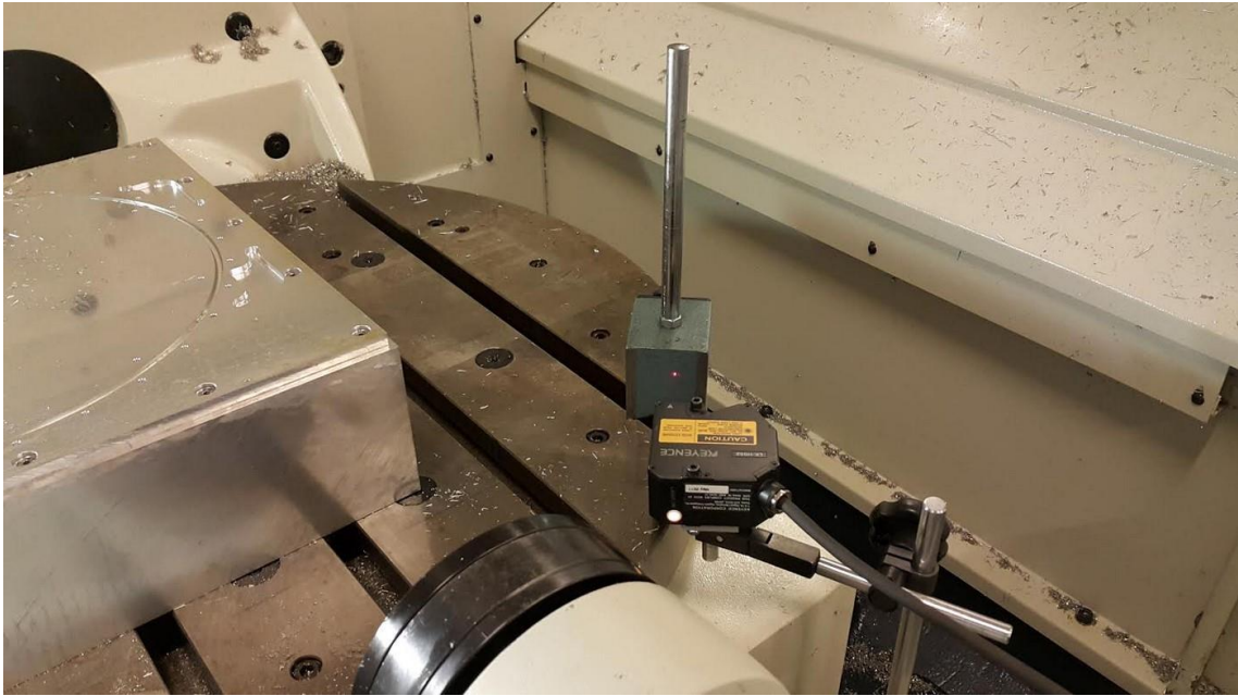
Figure 3-10: Laser Displacement Sensor Test Setup for Rotary C-Axis Measurements
