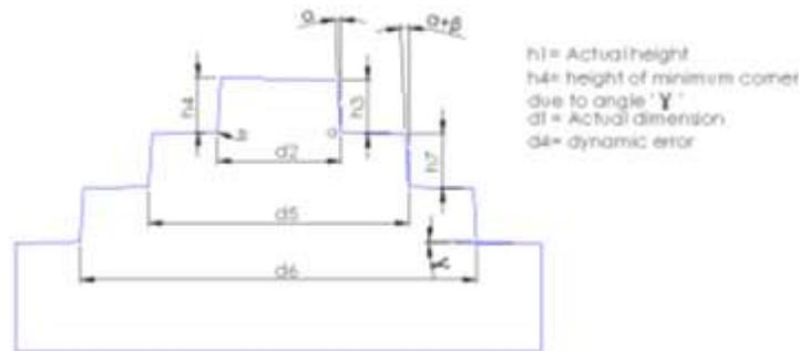
Figure 2 Final Dimensions of the workpiece after machining.
