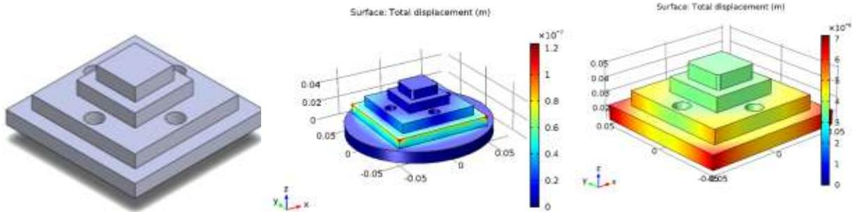
Figure 1 Workpiece design(left), Displacement of workpiece with(middle) and without(right) fixture.
