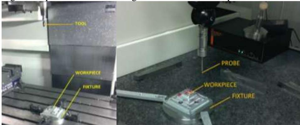
Figure 3 Machining setup (Left), Measurement Setup (Right)
