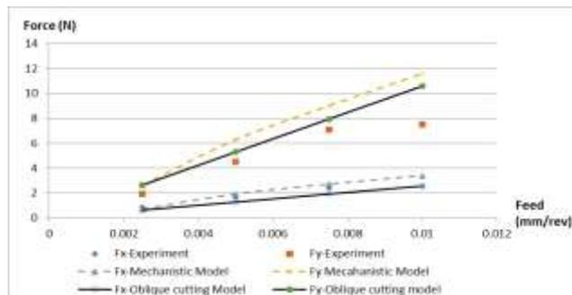
Figure 4 Comparison of force for CBN and aluminium oxide (conventional) wheel, at different feed rate and wheel speed of 40 m/s, depth of cut of 20  $\mu\text{m}$
