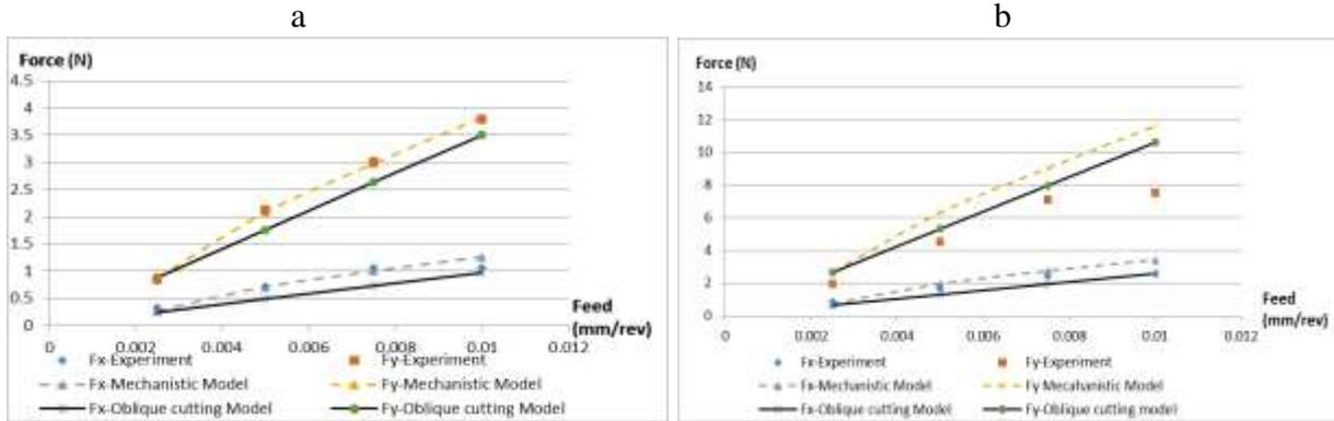
Figure 3 a) Comparison between experimental data, mechanistic and oblique cutting model, at different feed rate. wheel speed of 40 m/s, depth of cut of 20  $\mu\text{m}$ , CBN wheel b) depth of cut of 60  $\mu\text{m}$
