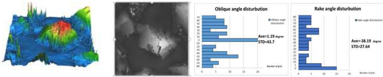
Figure 2 a) Individual grit scans, CBN wheel b) Oblique and rake angles distribution of CBN grits
