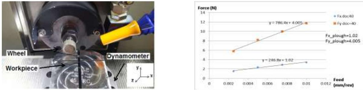
Figure 1 a) Experimental setup and b) grinding force (N) at different feed rate (mm/rev) depth of cut 40μm, wheel speed 40 m/s, CBN wheel.
