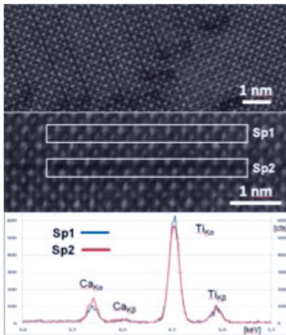
Figure 4. HAADF STEM image of RP loops in thin region of CaO-doped STNO. The EDX spectra acquired from marked frame scans shows that the Ca content at the fault is higher as compared to the matrix.
