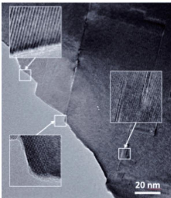
Figure 1. Bright-field TEM image of SrO-doped STNO. The following three regions are observed: the region with ordered RP faults, STNO perovskite solid solution and region with isolated RP faults.
