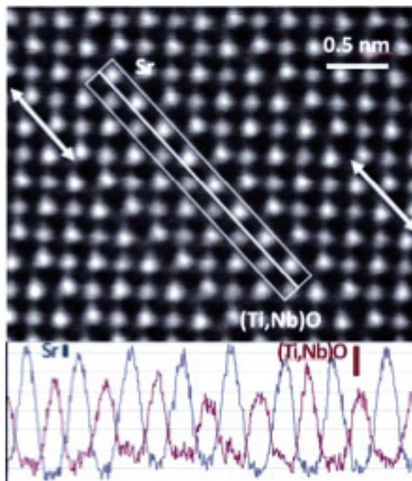
Figure 2. HR HAADF STEM micrograph of RP faults in SrO-doped STNO as seen in the [001] zone axis. Sr and mixed (Ti,Nb)O atomic columns are distinguished due to different intensities. Large scatter in measured intensities of (Ti,Nb)O atom columns is observed.
