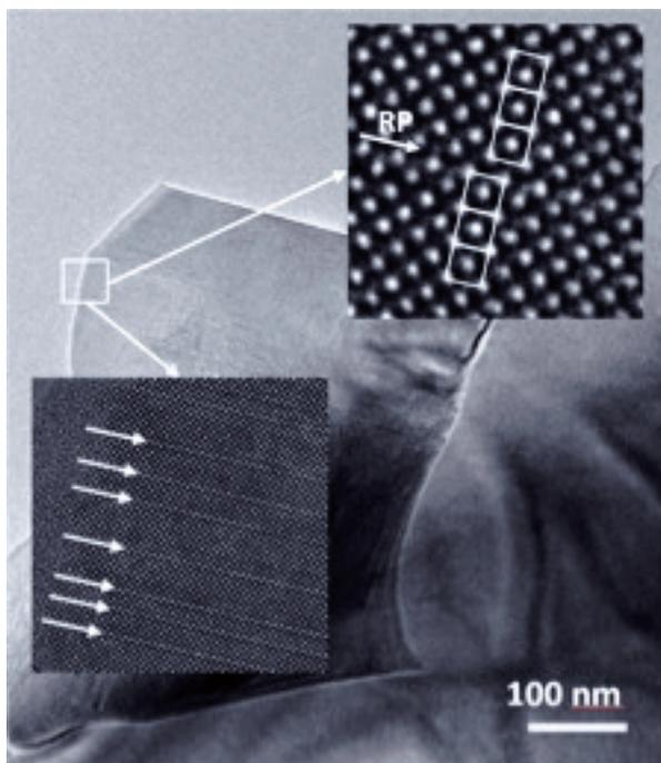
Figure 3. Bright-field TEM micrographs of CaO-doped STNO grains. The insets show the region with ordered RP faults. The RP faults are marked with arrows.
