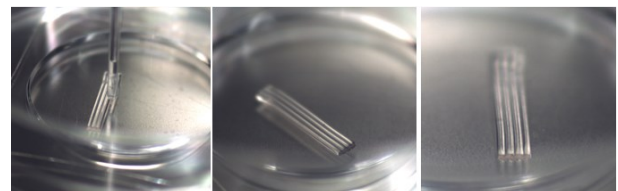
Fig. 2: Bioprinting process of cell-laden hydrogel structure. (Stripe lengths are 10mm)
