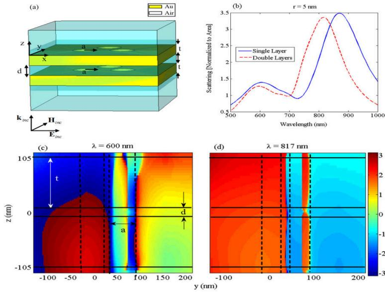
**Figure 1 (a).** The schematic representation of the stacked symmetric nanohole trimers. **(b)** The normalized scattering spectrum for the nanohole trimers milled in a single (solid-line), and double stacked (dashed-line) layers of gold film obtained by simulations. **(c)**, and **(d)** phase variations of  $\angle H_y$  component at  $\lambda = 600$  nm, and  $\lambda = 817$  nm, respectively.
