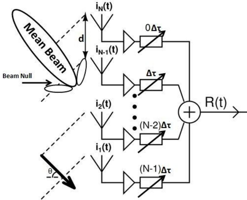
Fig. 2. N-element Phased Array system example
