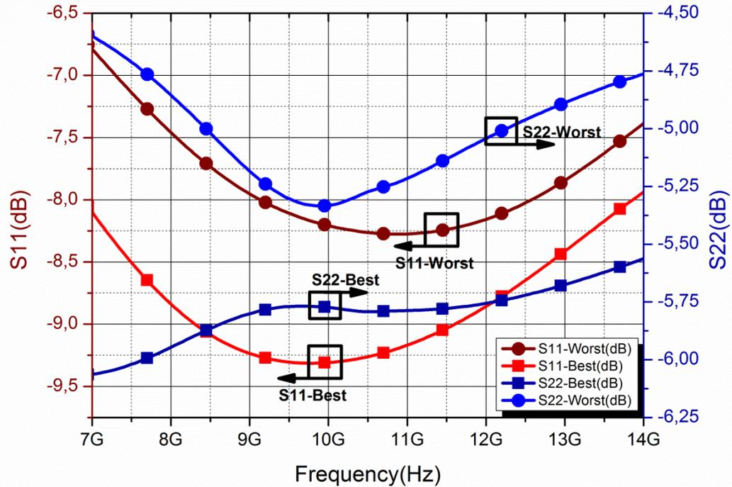
Fig. 50. Best and worst input and output matching performances of hybrid phase shifter
