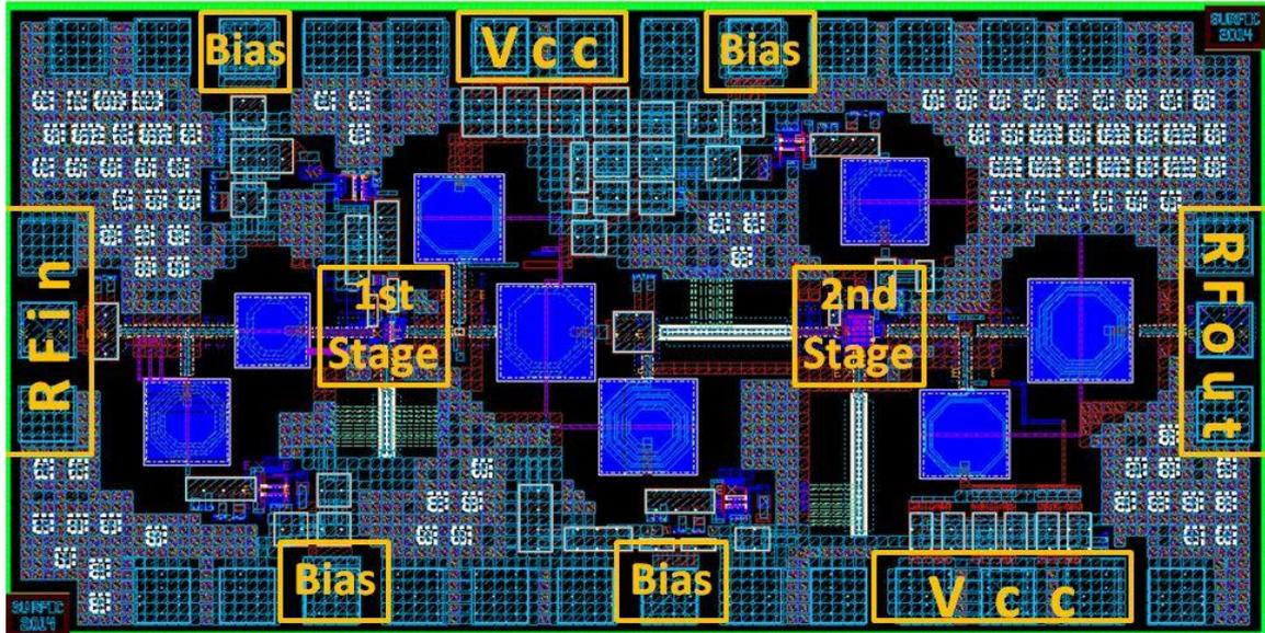
Fig. 26. Layout view of two-stage LNA
