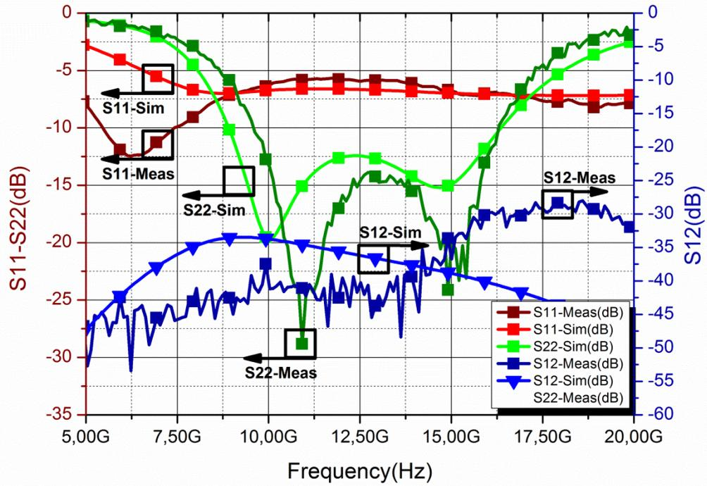
Fig. 17. Correlated measurement and simulation results for Single-Stage cascode LNA
