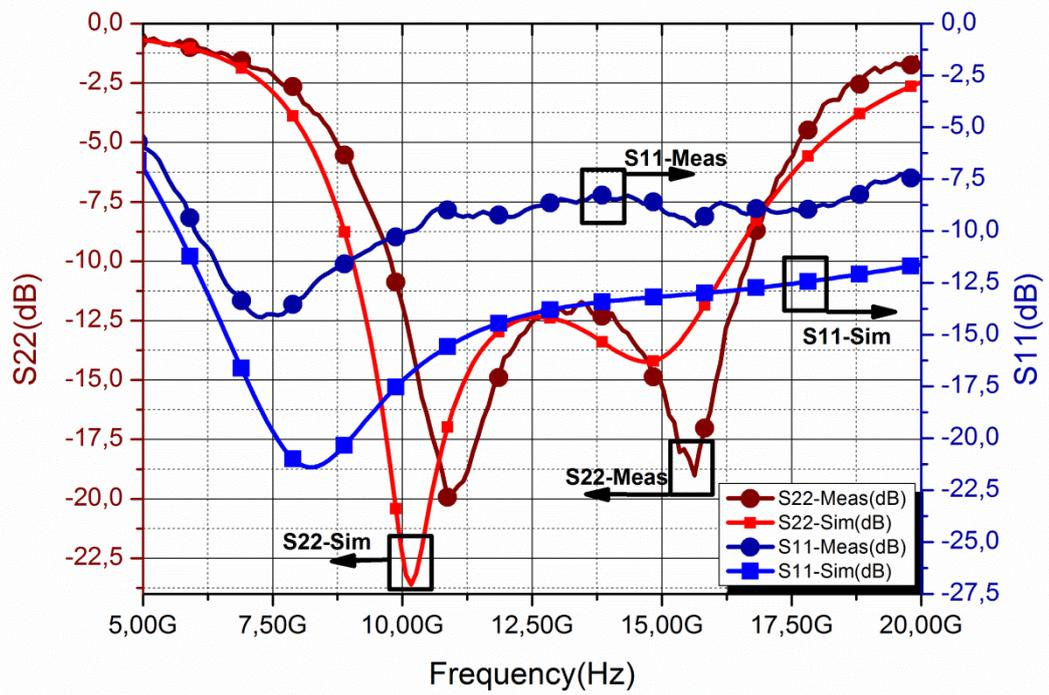
Fig. 12. Simulated and measured return loss performances of Single-Stage LNA
