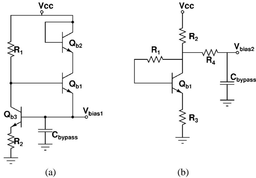
Fig. 10. Preferred active bias networks for Single-Stage cascode LNA
