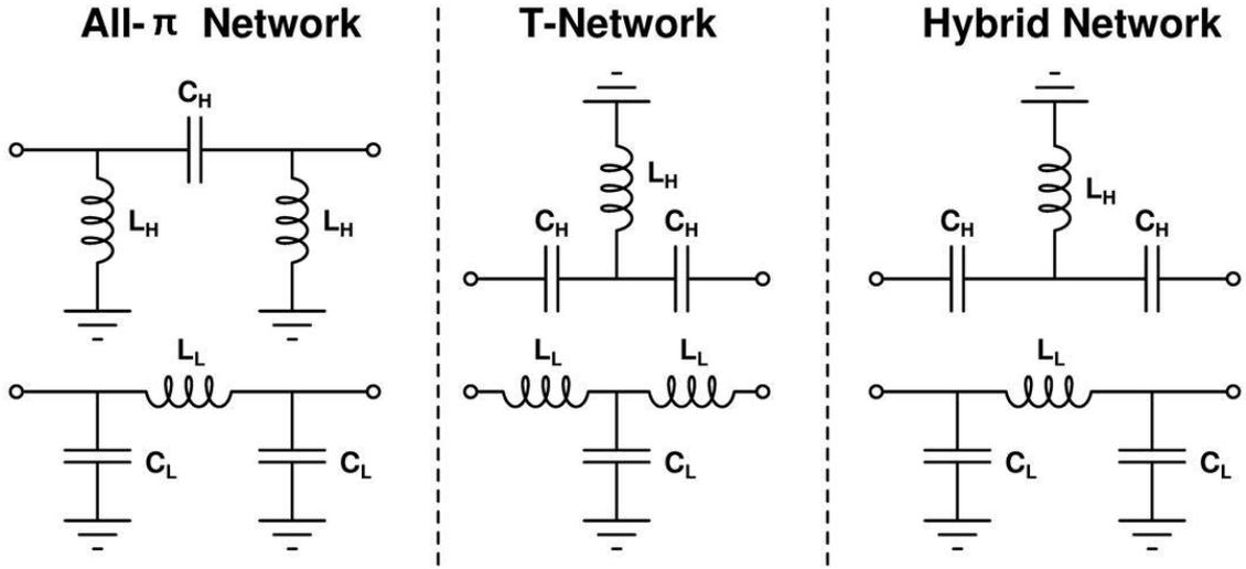
Fig. 37. Different filter type phase shifters architectures
