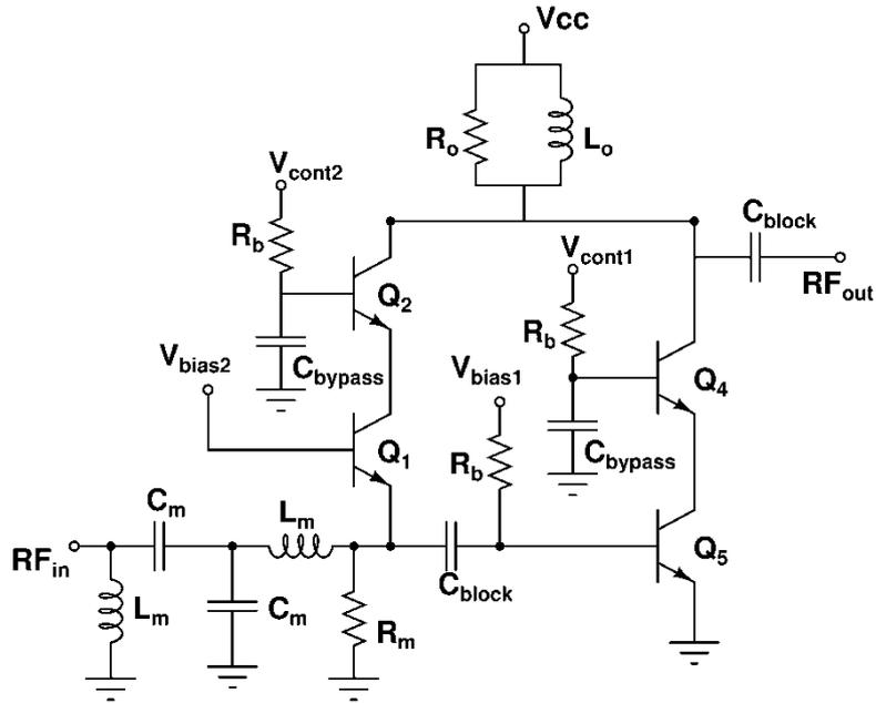
Fig. 40. Common Base – Common Emitter architecture for 6<sup>th</sup> bit
