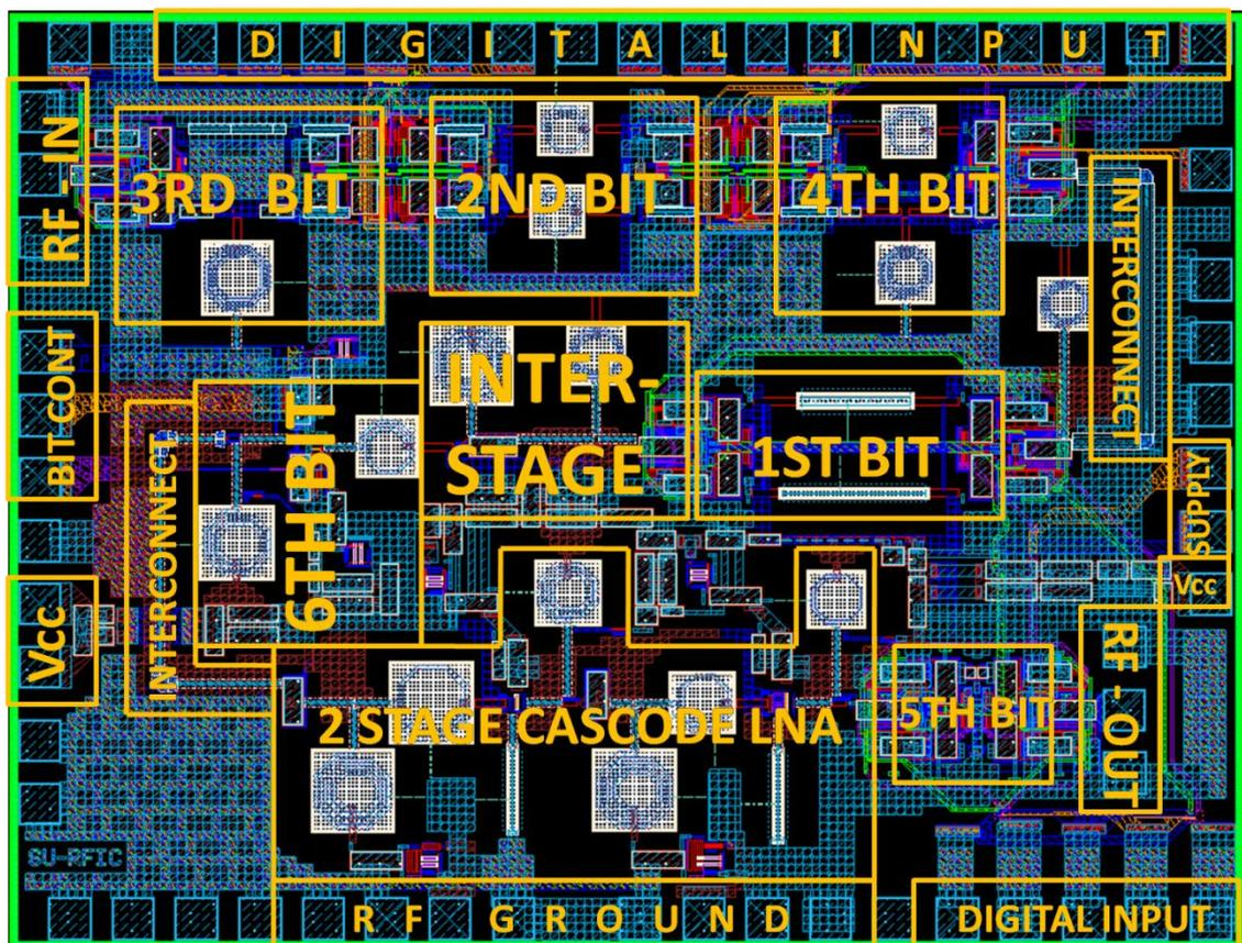
Fig. 46. Layout of hybrid phase shifter
