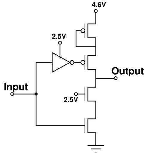
Fig. 44. Level shifter for digital circuitries
