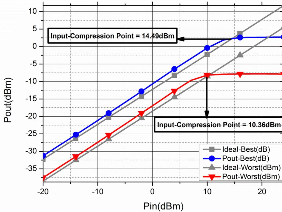
Fig. 49. Best and worst input-P1dB performance 6-bit hybrid phase shifter
