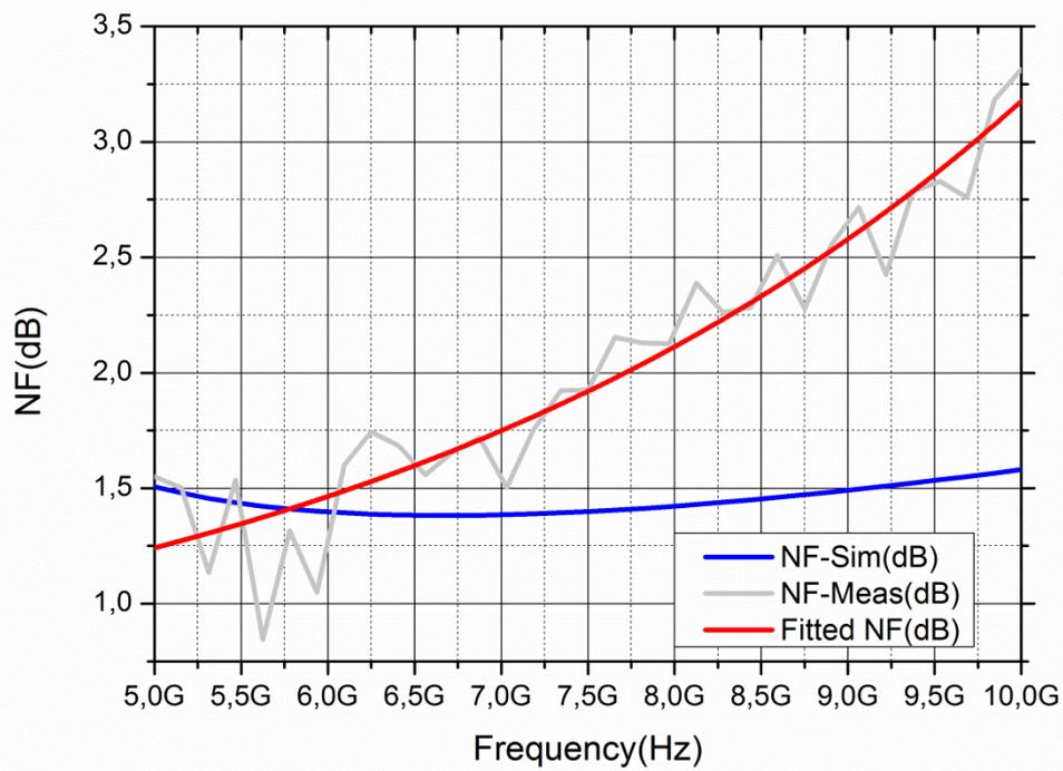
Fig. 22. Simulated and measured NF of Telescopic LNA
