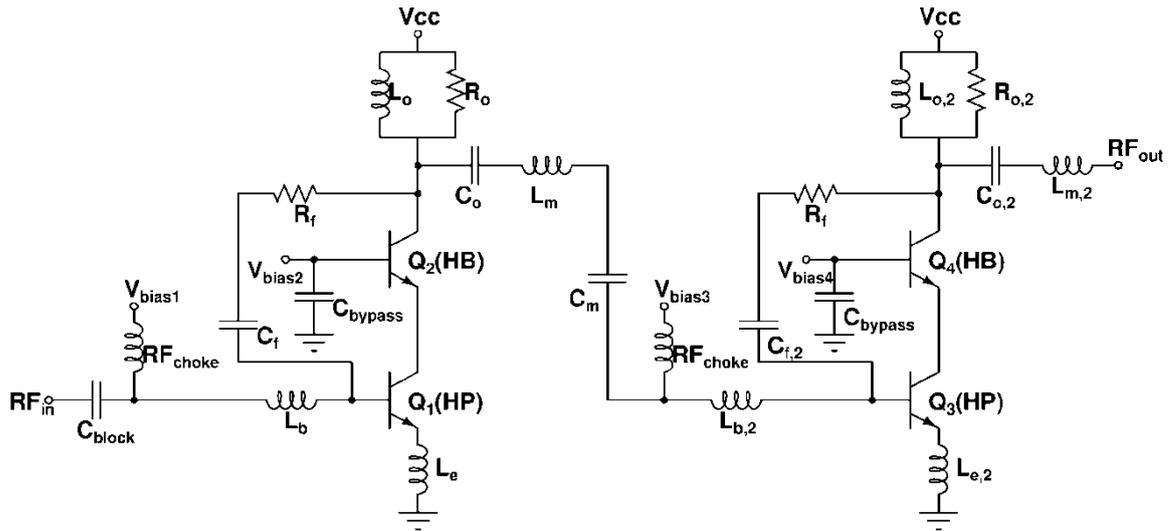
Fig. 24. Two-Stage Cascode Low Noise Amplifier Design
