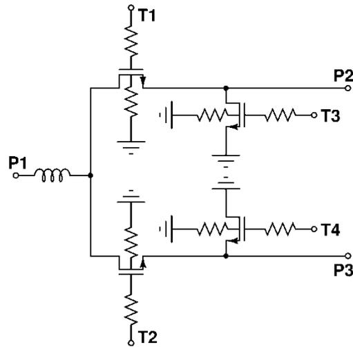
Fig. 34. Basic representation of SPDT switch
