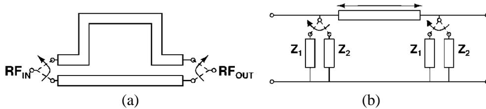
Fig. 30. Representation of a) Switched Line and b) Load Line Phase Shifters
