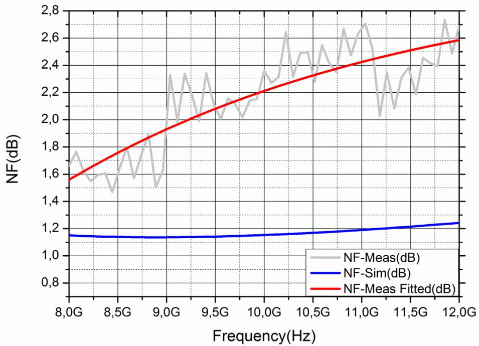
Fig. 15. Simulated and measured NF performance
