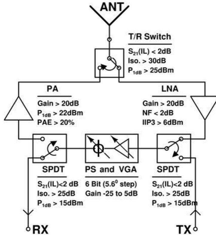
Fig. 7. Block diagram of X-Band phased array T/R Module
