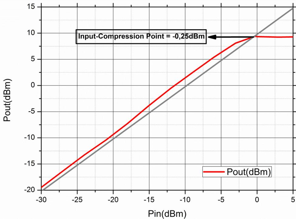
Fig. 16. Measured input-referred compression point of Single-Stage cascode LNA
