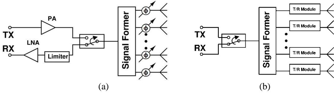
Fig. 3. Block Diagram of a) Passive Phased Array b) Active Phased Array
