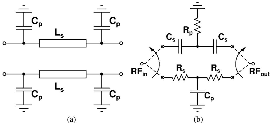
Fig. 39. a) LSB and b) 5<sup>th</sup> bit of hybrid phase shifter
