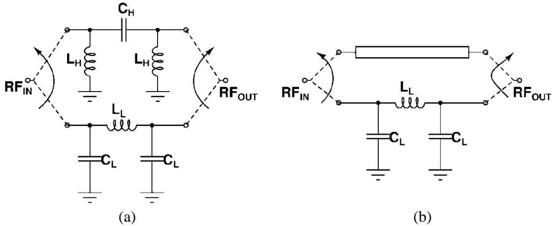
Fig. 31. Representations of a) HP-LP and b) BP-LP phase shifters
