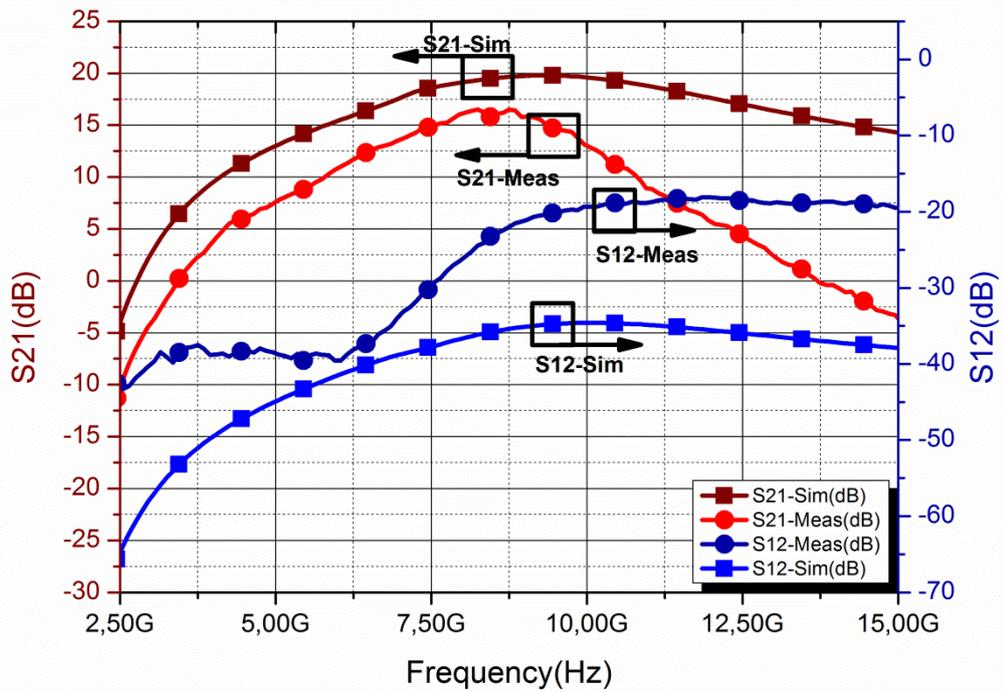
Fig. 21. Simulated and measured S21 and S12 parameters of Telescopic LNA
