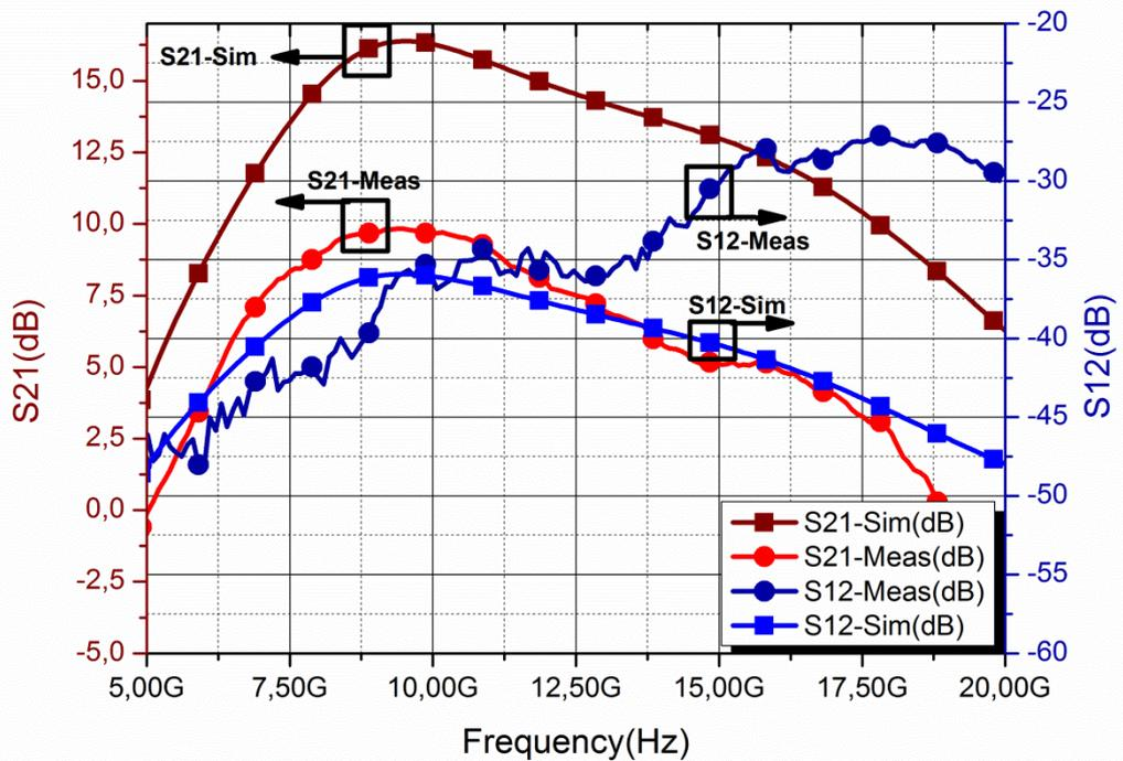
Fig. 13. Simulated and measured S21 and S12 parameter of Single-Stage LNA
