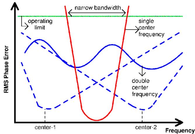
Fig. 41. Description for RMS phase error with double center frequency
