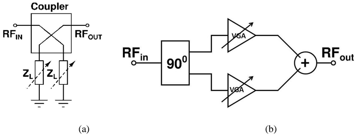
Fig. 32. Representations of a) RTPS and b) Vector Modulator type phase shifter
