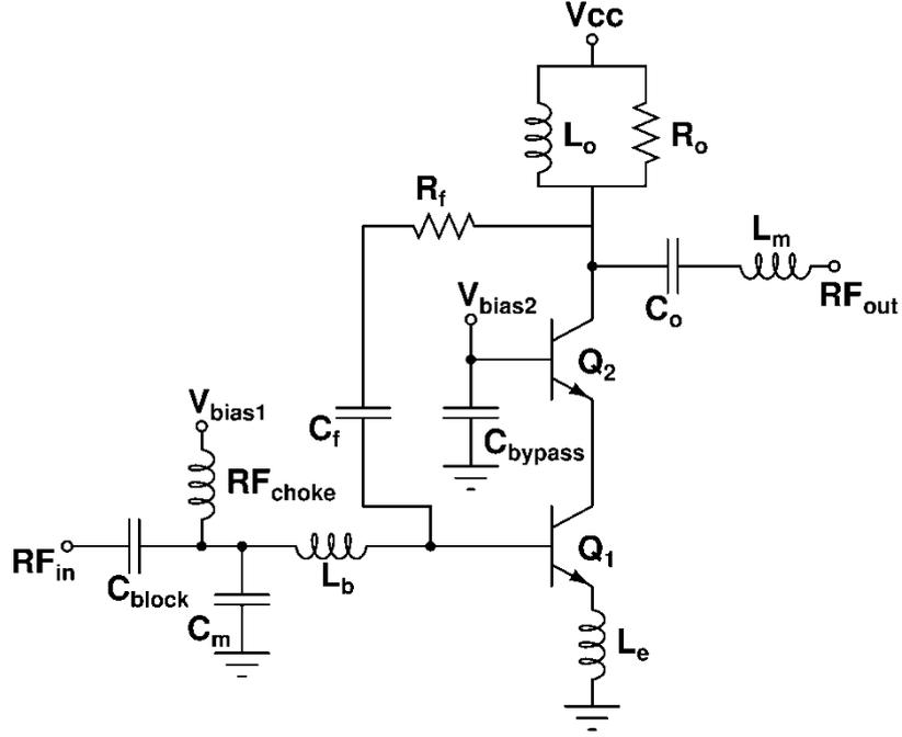
Fig. 8. Schematic view of Single-Stage Cascode Low Noise Amplifier
