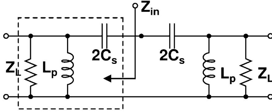
Fig. 38. Half-circuit analyze of HP filter for  $\pi$ -network
