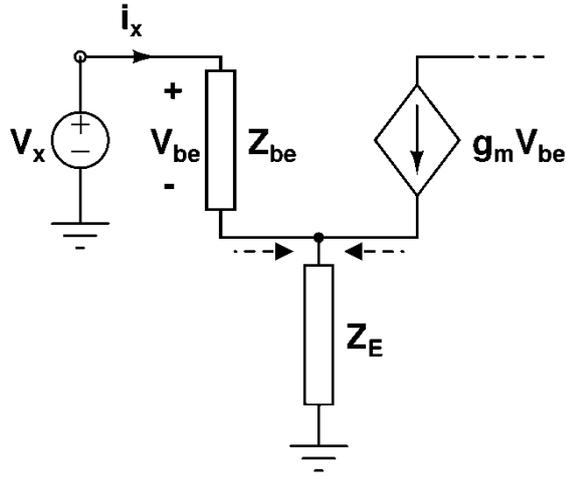
Fig. 9. Small signal representation for driver transistor of cascode design
