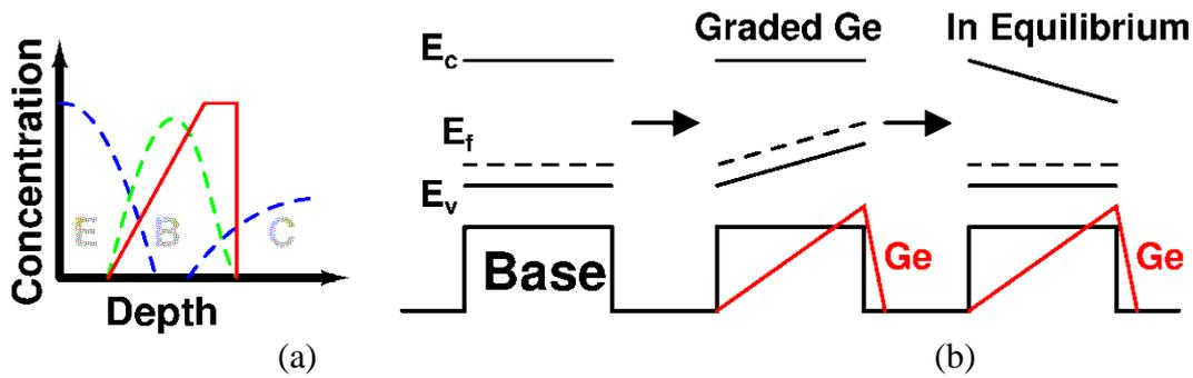
Fig. 6. a) Concentration of Ge through device and b) energy band diagram of HBT
