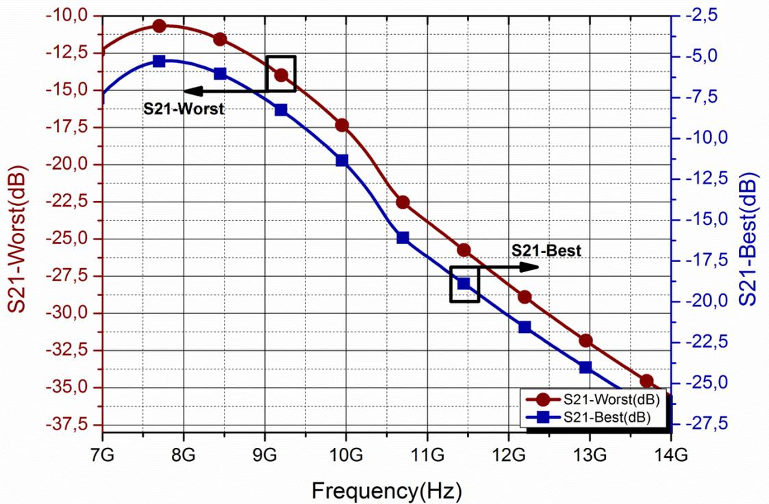
Fig. 48. Best and worst gain performance of 6-bit hybrid phase shifter
