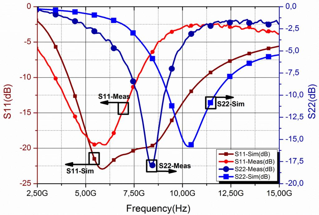
Fig. 20. Simulated and measured return loss of Telescopic LNA
