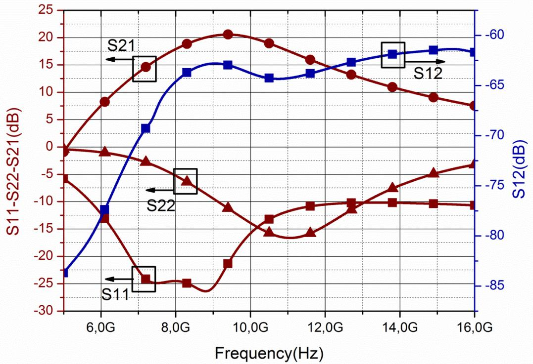
Fig. 27. S-parameter results of two-stage LNA
