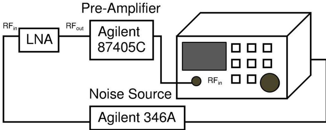
Fig. 14. Noise measurement setup representation for LNA
