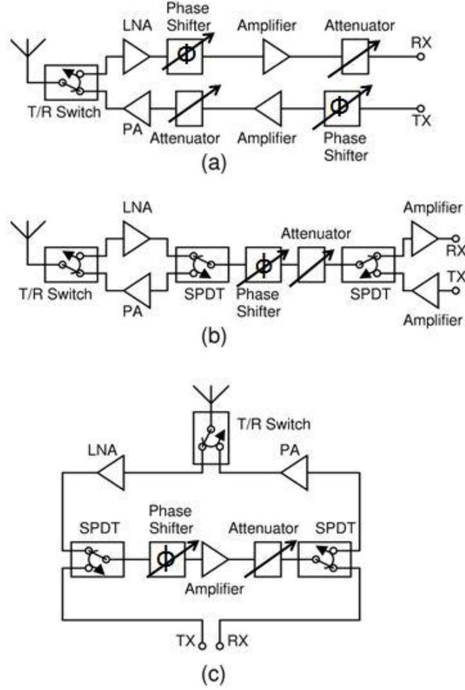
Fig. 4. Various All-RF T/R Module architectures
