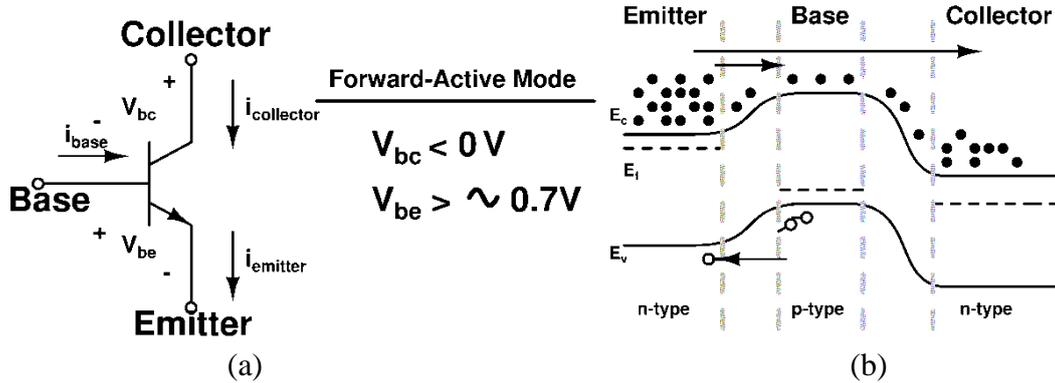
Fig. 5. a) Symbolic and b) band diagram description of BJT
