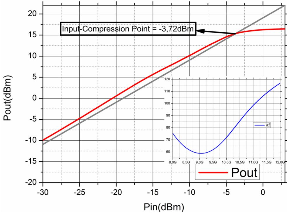
Fig. 29. Input compression point of two-stage LNA
