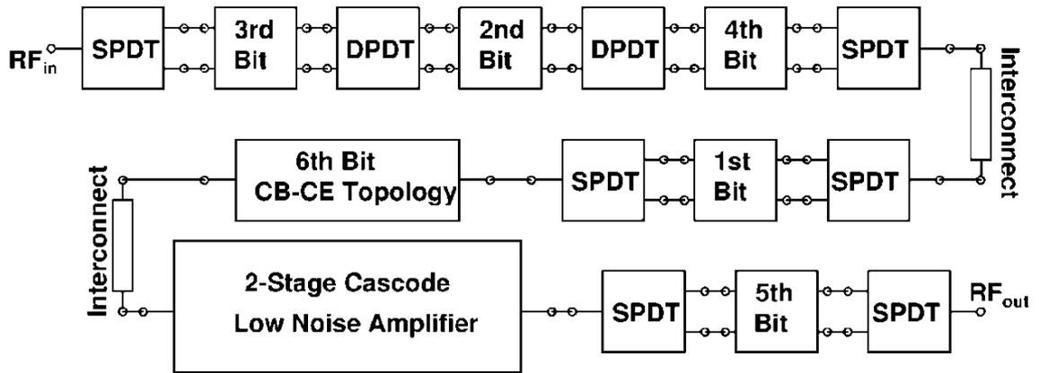
Fig. 45 Order of stages for hybrid phase shifter
