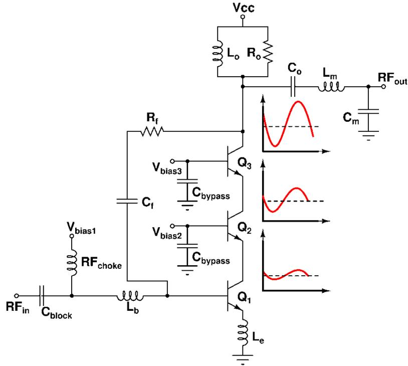
Fig. 18. Schematic view of preferred telescopic LNA
