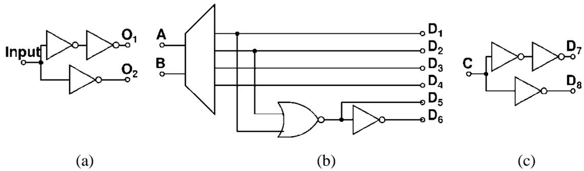
Fig. 43. Control circuitries for SPDT and DPDT switches
