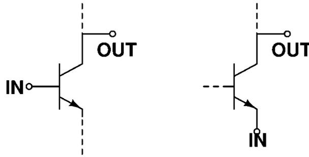
Fig. 25. Representation of Common-Base and Common-Emitter amplifiers
