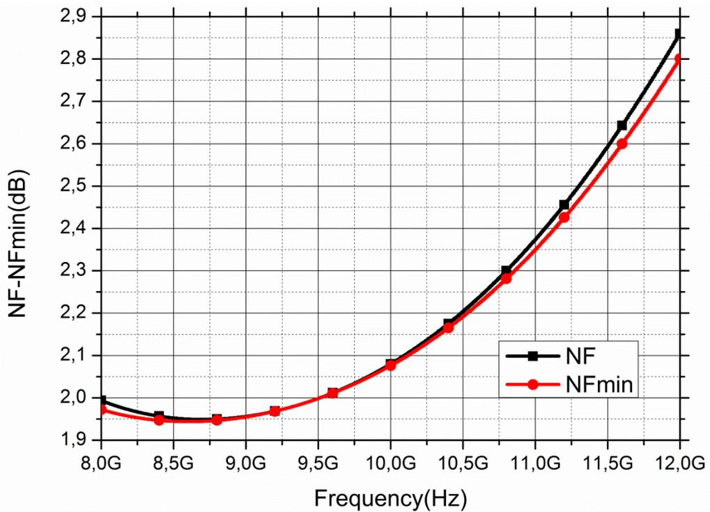
Fig. 28.  $NF_{min}$  and NF results for two-stage LNA
