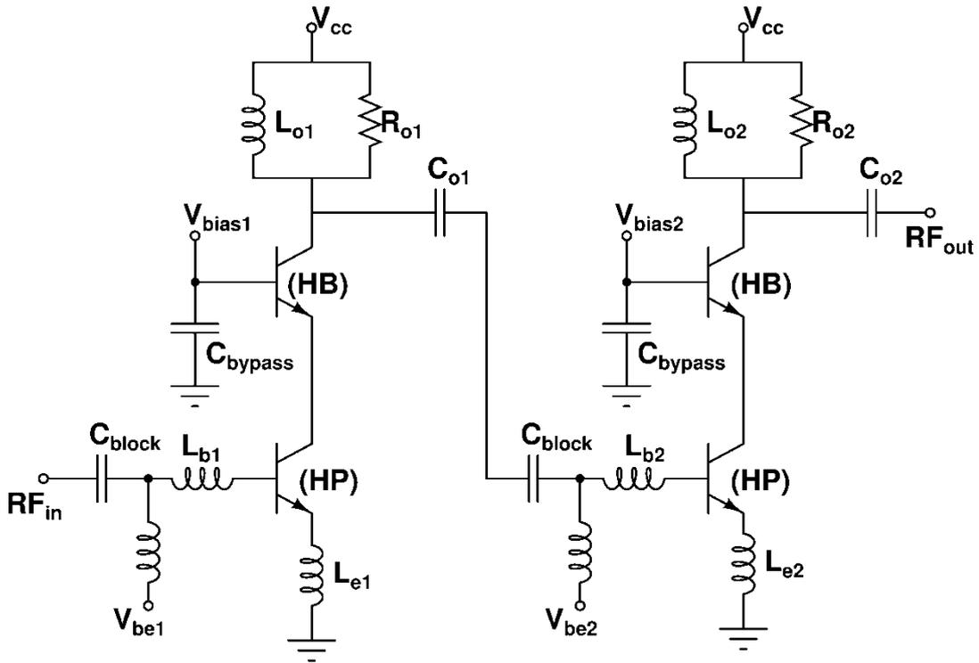
Fig. 42. Low Noise Amplifier for hybrid phase shifter
