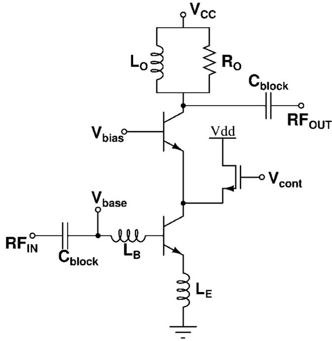
Fig. 33. Representations of VGA with current-steering technique
