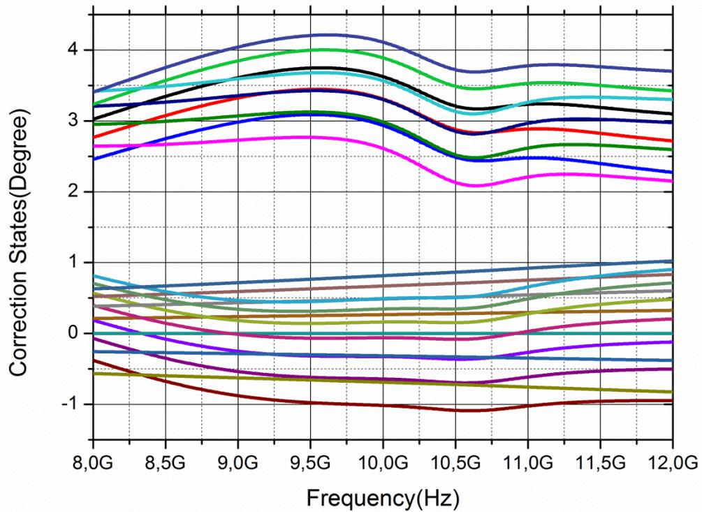
Fig. 51. Correction states of hybrid phase shifter
