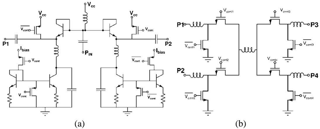
Fig. 35. Basic representation of a) Active-SPDT and b) Cascaded-SPDT switch
