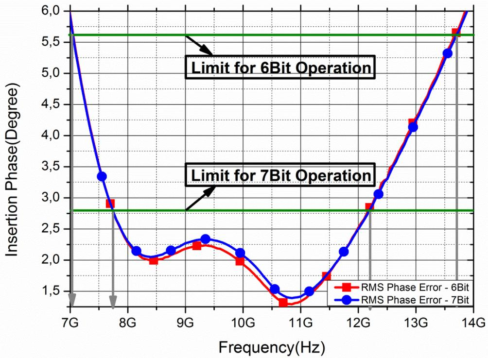
Fig. 47. RMS phase error for 6-bit and 7-bit operation of hybrid phase shifter
