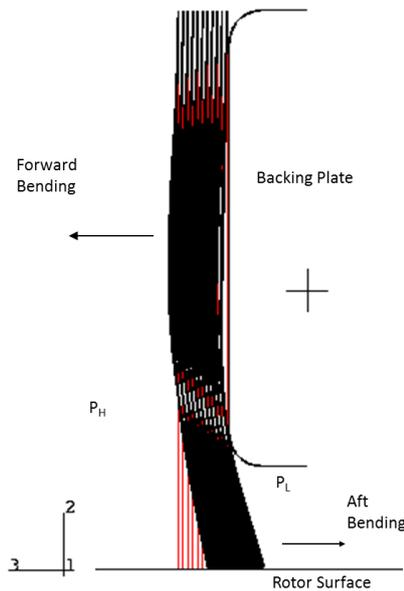
Figure 8: Brush pack behavior under pressure load [5].
