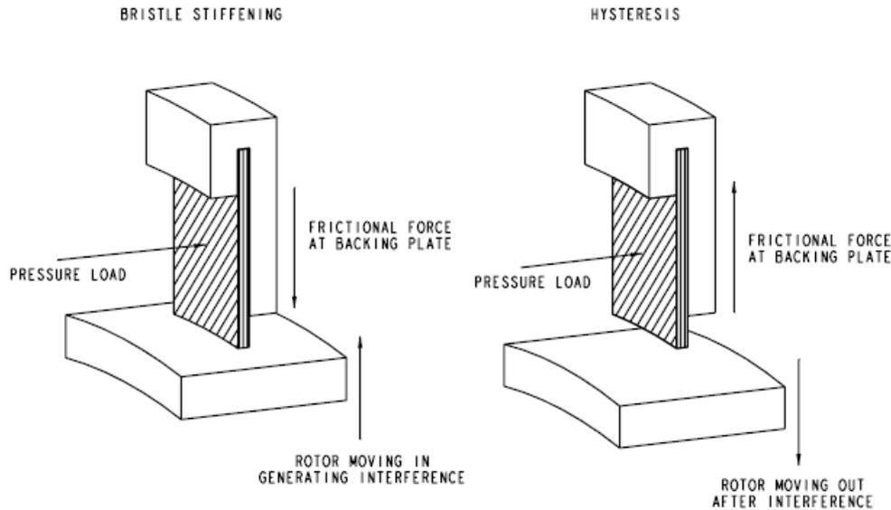
Figure 5: Role of friction in seal stiffening [5].
