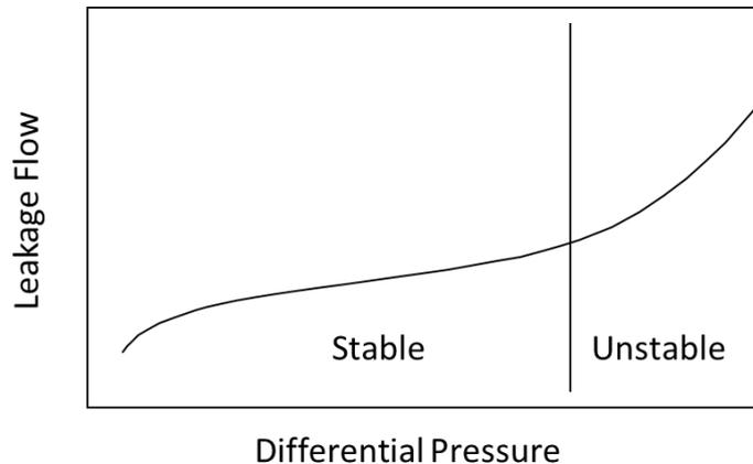
Figure 9: Brush seal leakage under increasing pressure load.
