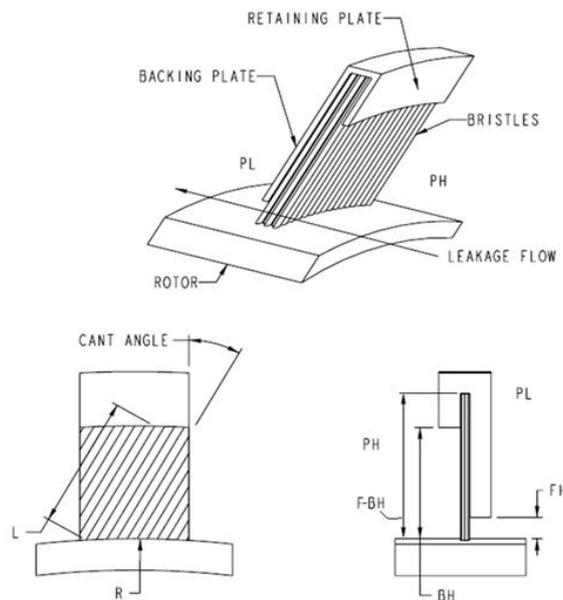
**Figure 1: Brush seal schematic and main design parameters.**
