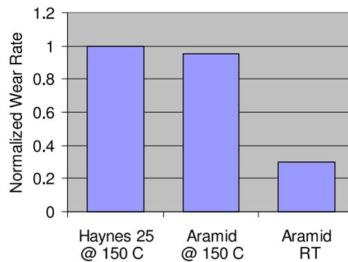
Figure 3: Wear test results for aramid and Haynes 25 tufts against Ni-Cr-Mo-V. Data are normalized with wear rate of Haynes 25 bristles at 150 °C [6].
