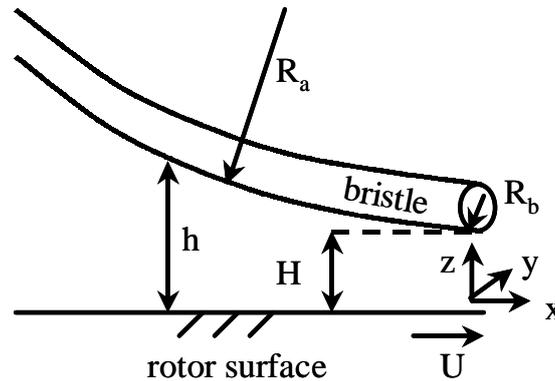
Figure 7: Hydrodynamic lift geometry for bristles [8].
