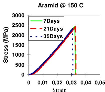
Figure 4: Aramid fiber strength upon exposure to 150 °C (300 °F) [6].
