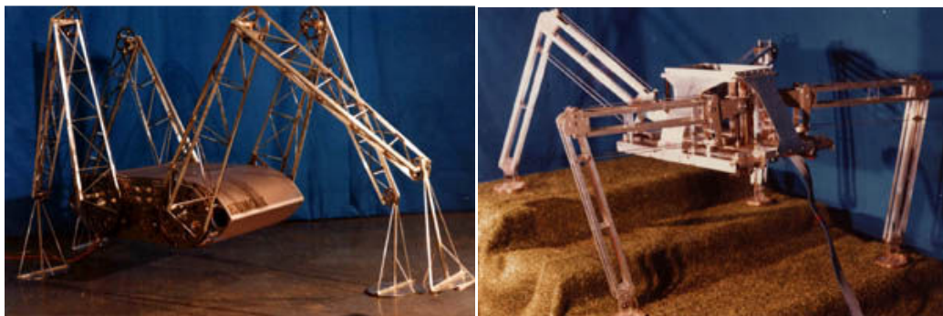
Figure 2.11: Quadruped robots KUMO I (left) and PV II (right)
