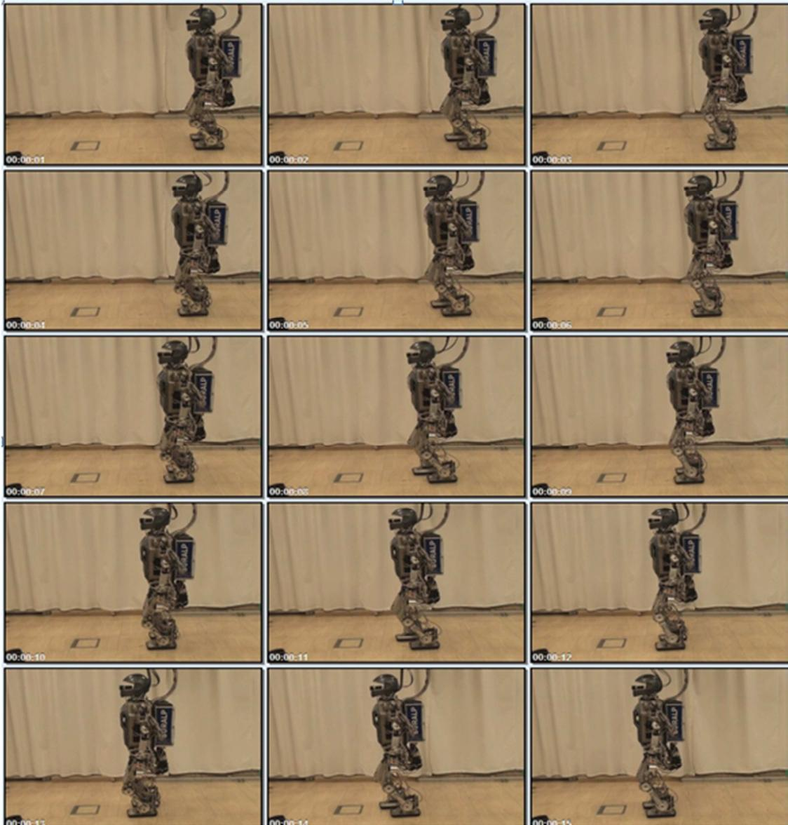
Figure 6.9: Snapshots of SURALP walking with  $v_{average} = 0.07m/s$
