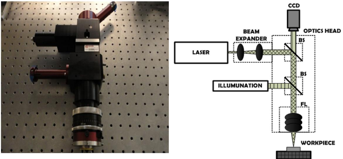
Figure 4.14. – Laser micromachining head (left) and sketch of optical system (right)
