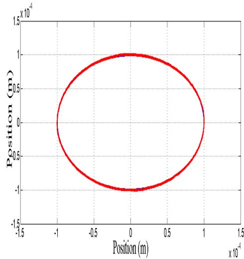
Figure 5.1. - Trajectory tracking for circular reference of  $100\mu\text{m}$  radius
