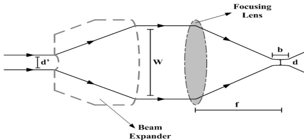
Figure 3.4. – Beam Expander and Focusing Lens
