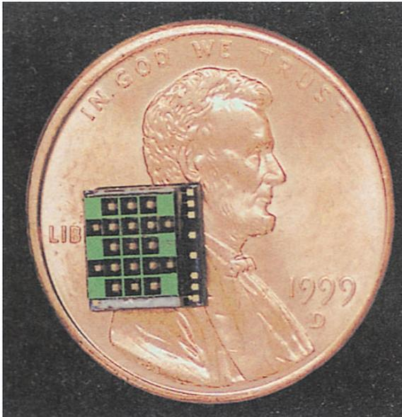
Figure 2.2. - A (3x 5) array of digitally addressable microthrusters. [9]
