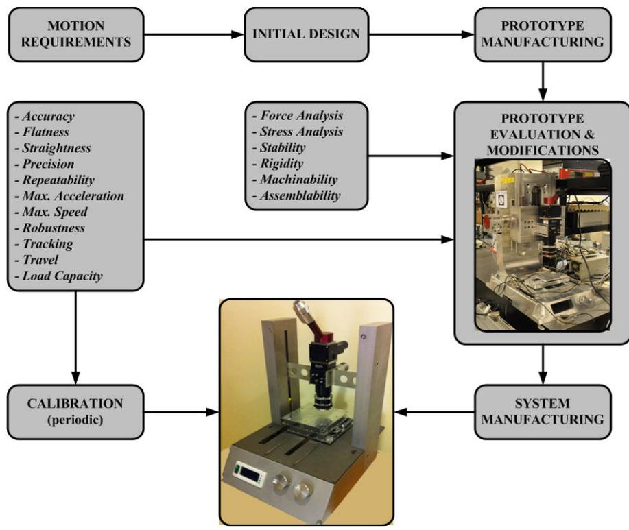
Figure 3.2. – Overall design process
