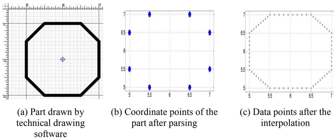
Figure 4.6. – dxf file processing and interpolation steps
