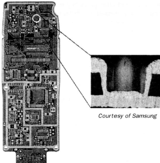
Figure 2.9. - Personal communication system with microvias. [30]
