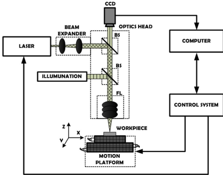
Figure 3.1. - Schematic of laser micromachining system
