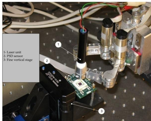
Figure 5.8. – Experimental setup
