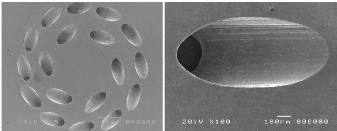
Figure 2.4. - Gasoline injector for a high performance racing engine (left) and high magnification of one of the holes (right) [31]
