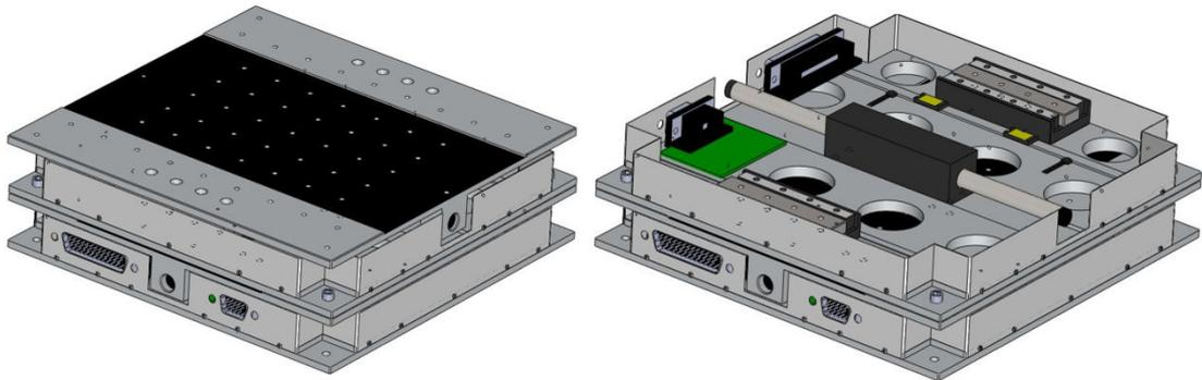
Figure 4.5. – Planar x-y positioning stage
