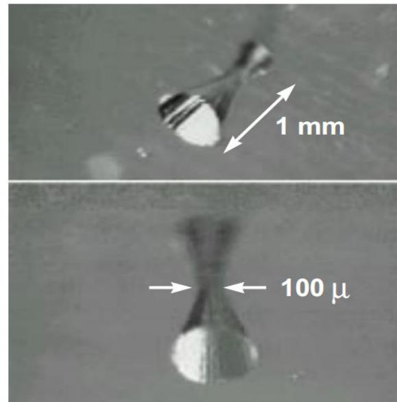
Figure 2.3. - Optical microphotographs of a laser machined converging/diverging nozzle.[10]
