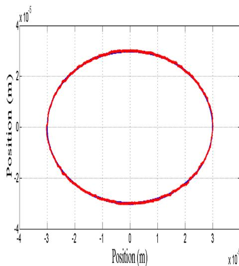
Figure 5.4. - Trajectory tracking for circular reference of  $30\mu\text{m}$  radius
