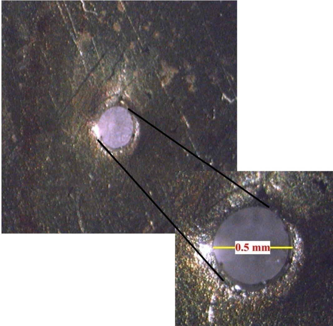
Figure 5.13 – Hole drilled in Brass
