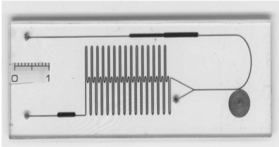
Figure 2.7. - Sample pattern fabricated in PMMA substrate. The scale bar is 1 cm. [27]
