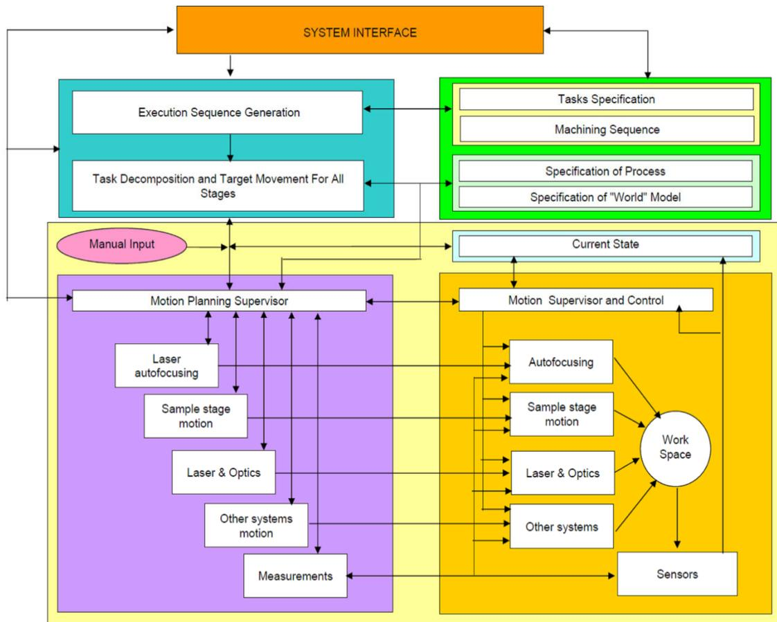
Figure 3.5. – Overall System Controller
