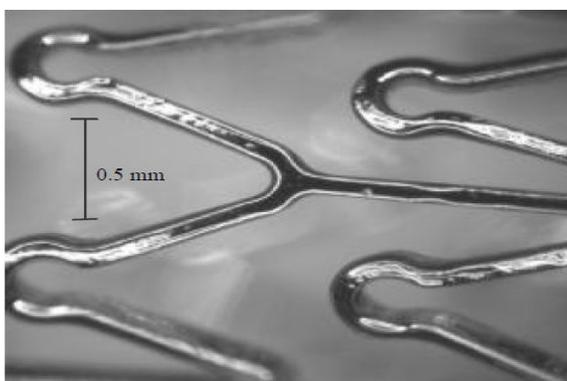
Figure 2.5. - Laser cut stainless steel stent [20]
