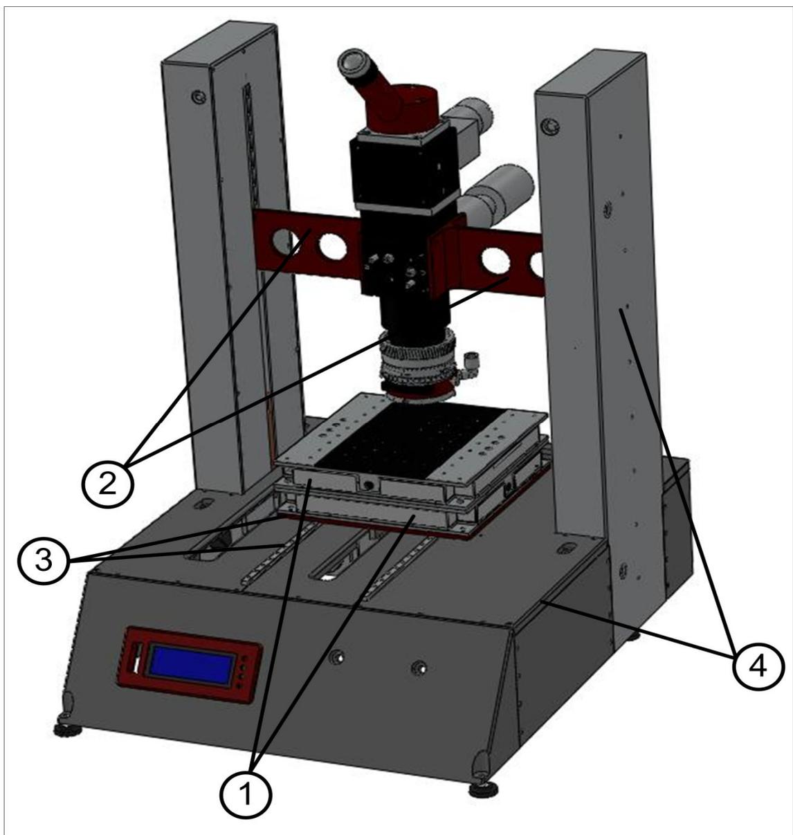
Figure 4.2. – Mechanical structure of laser micromachining system
