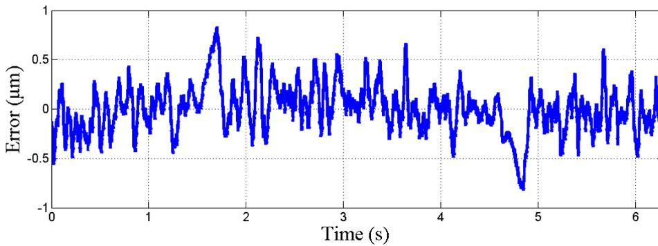
Figure 5.2. – Error in trajectory tracking for x axis
