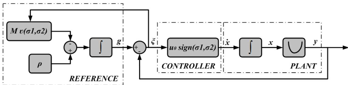
Figure 4.12 - Sliding mode optimization controller
