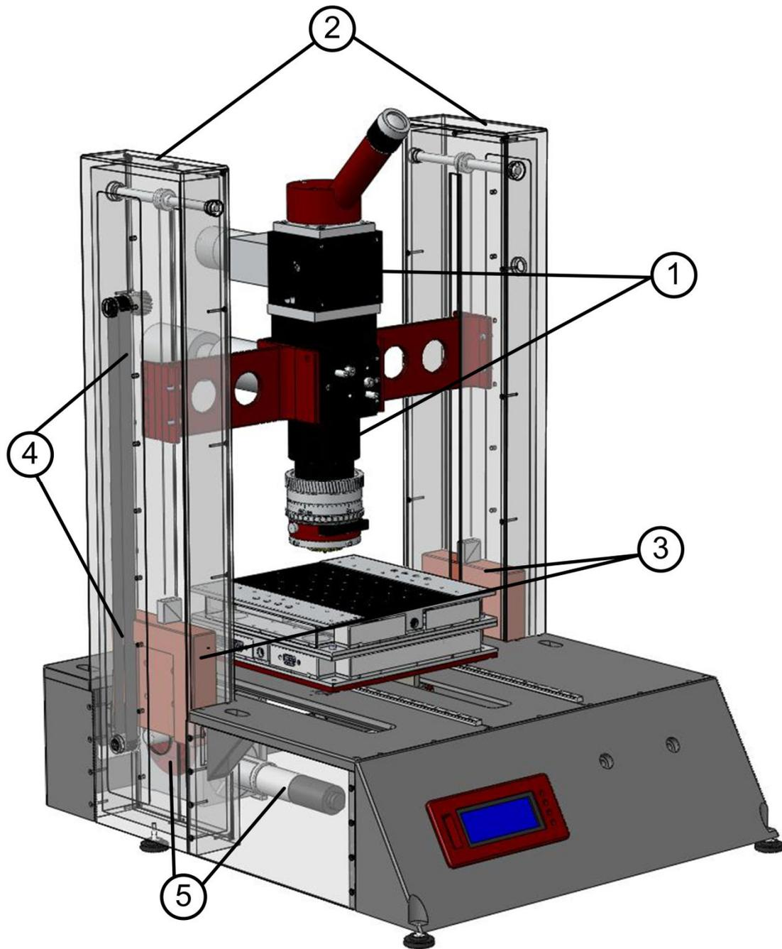
Figure 4.3. – Optics head lift mechanism
