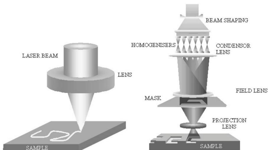
Figure 2.1. - Direct writing (left) and mask projection techniques (right) [3]
