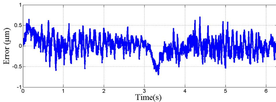
Figure 5.3. – Error in trajectory tracking for y axis
