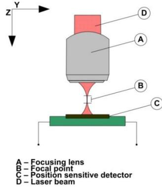
Figure 4.9 – Autofocusing system
