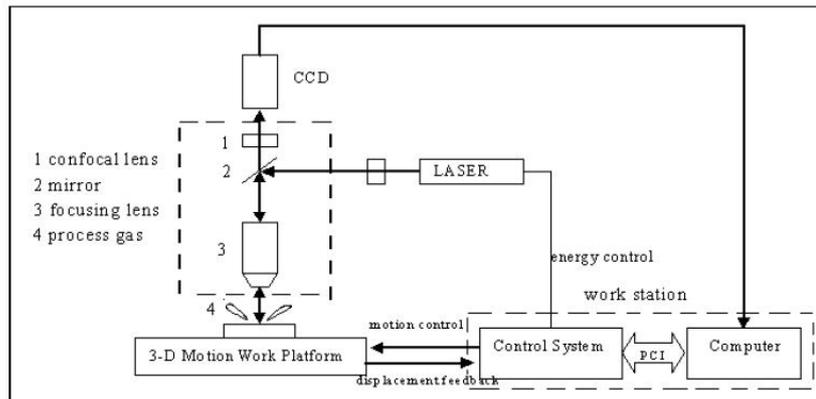
Figure 2.11. – Schematic of laser system [47]
