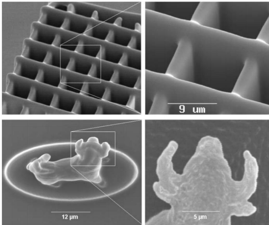
Figure 2.10. SEM images of a three-dimensional periodic structure (top) and a micro-bull statue (bottom) fabricated by two photon-polymerization in a hybrid polymer using femtosecond laser pulses. Corresponding enlarged fragments are shown on the right side of the figure [34]
