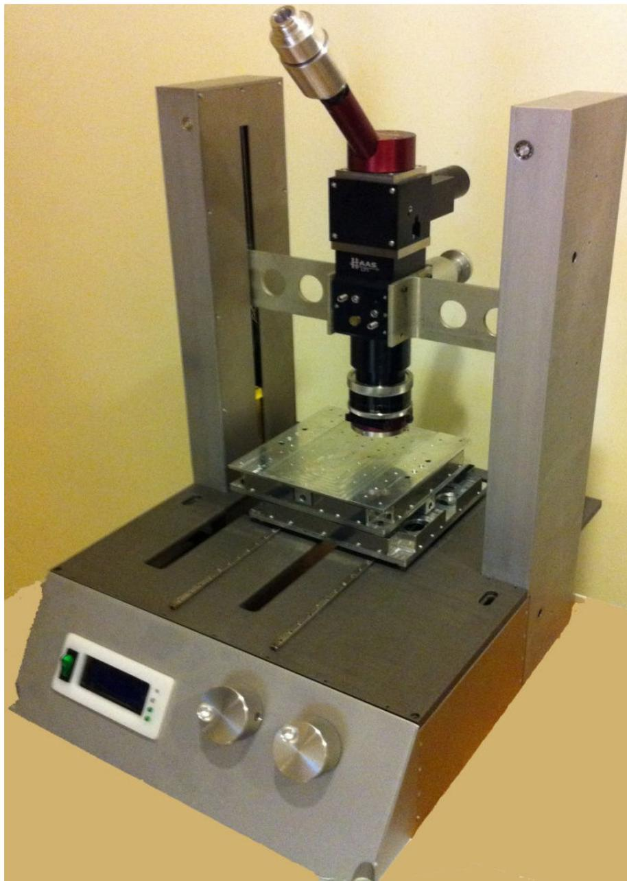
Figure 4.1 – Laser micromachining system
