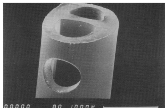
Figure 2.6. – 0.7 mm diameter hole for blood passage drilled with a laser [21]
