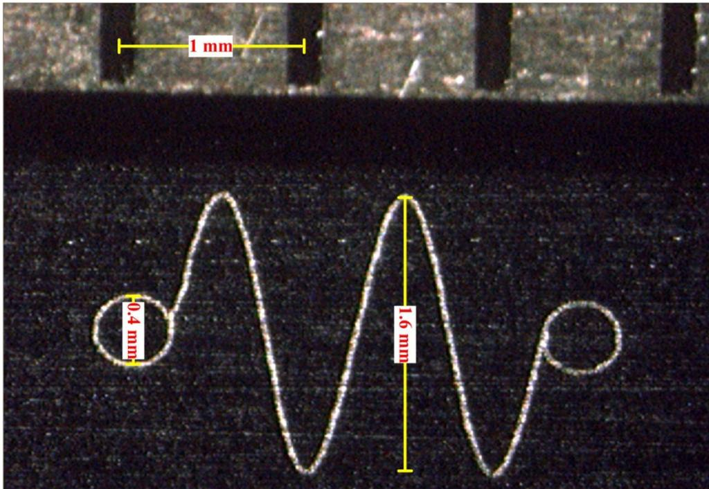
Figure 5.11 – Marking of coated anodized aluminum
