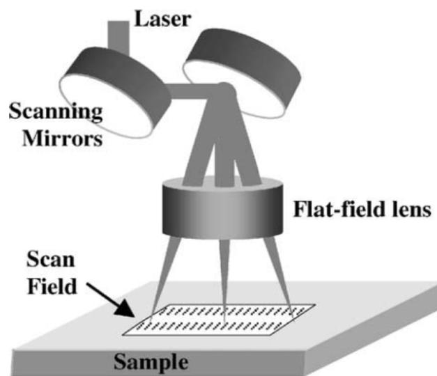
Figure 3.3. – Galvanometric scanner setup [32]
