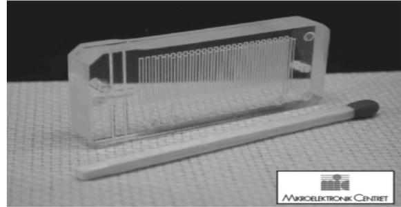
Figure 2.8. - Three-layered PMMA-microfluidic system for the detection of ammonia in aqueous samples. [22]
