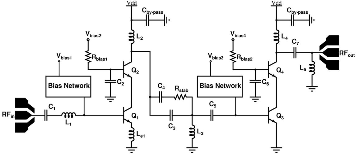
**Figure 11:** Schematic of the designed two-stage power amplifier.
