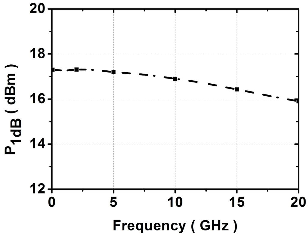
Figure 32: P1dB versus frequency of the SPDT switch.
