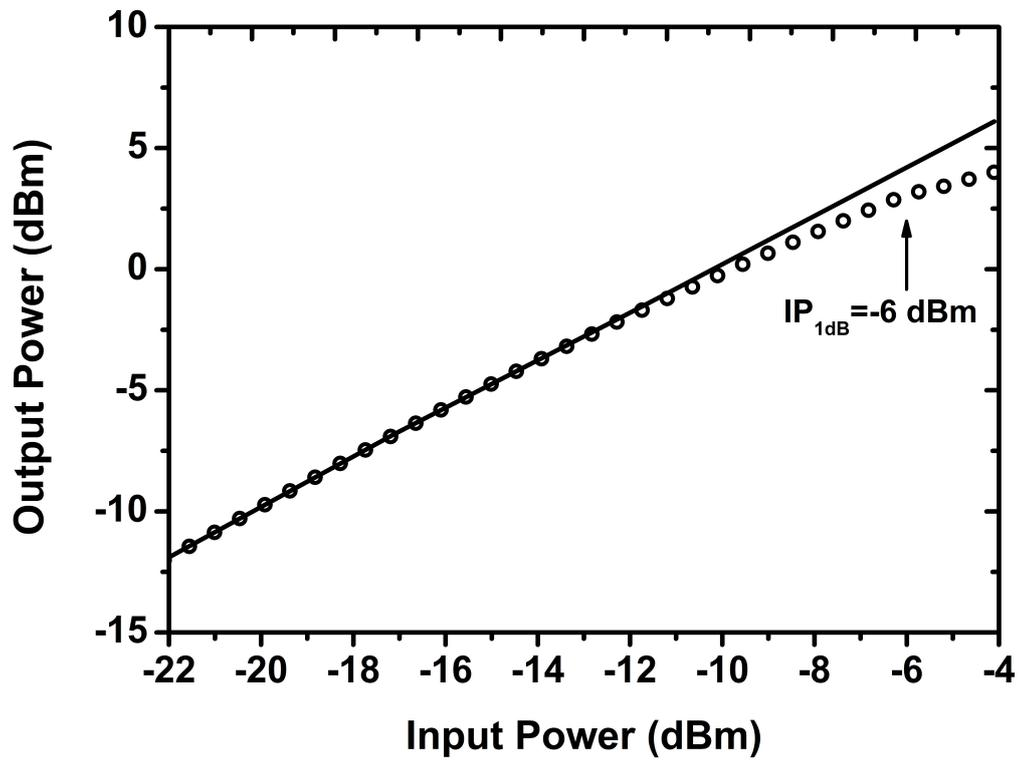
Figure 55: Measured P1dB of the switched LNA in gain mode.
