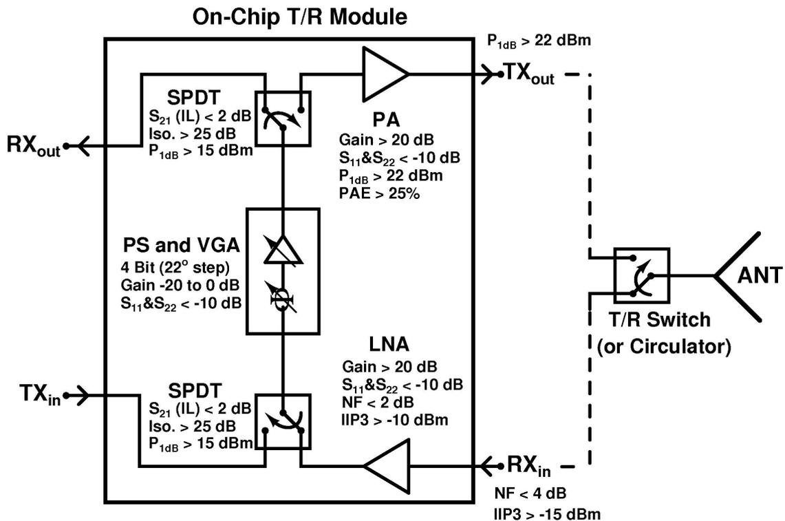
Figure 59: Block diagram of the X-Band SiGe BiCMOS T/R Module.
