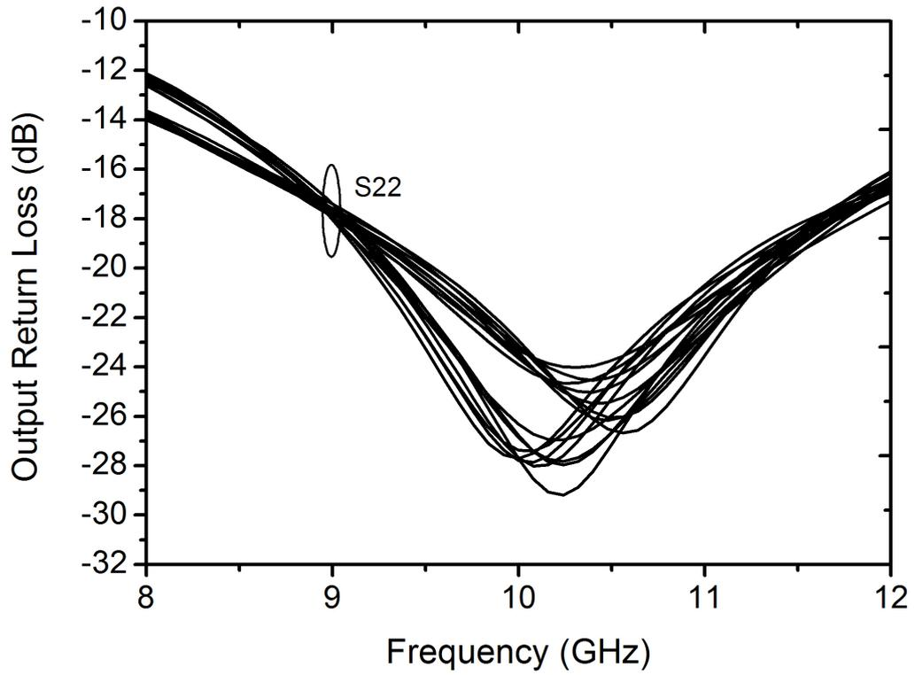
**Figure 64:** Simulated output return loss of the T/R module in the receive mode for all phase states.
