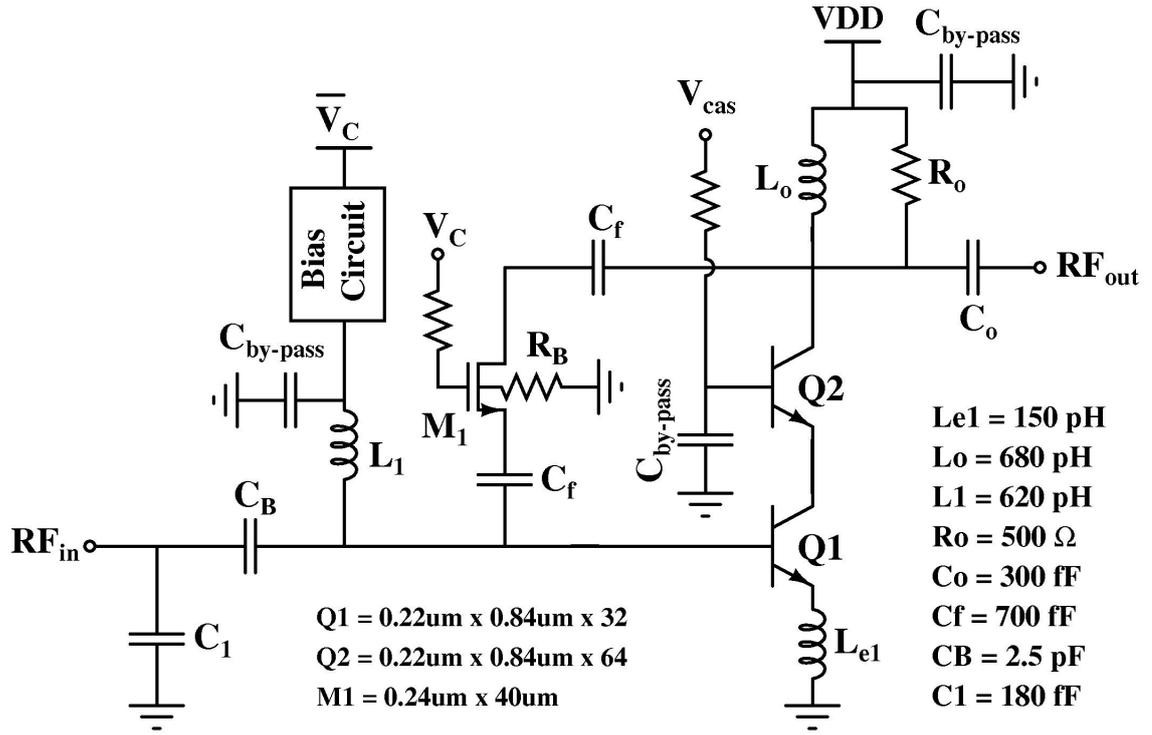
Figure 50: Circuit schematic of the switched gain LNA.
