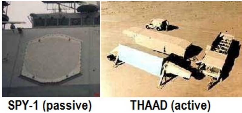
Figure 5: Photograph of a passive and active phased array radar
