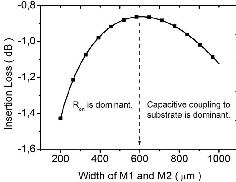
**Figure 19:** Transistor width versus insertion loss of the SPDT T/R switch.
