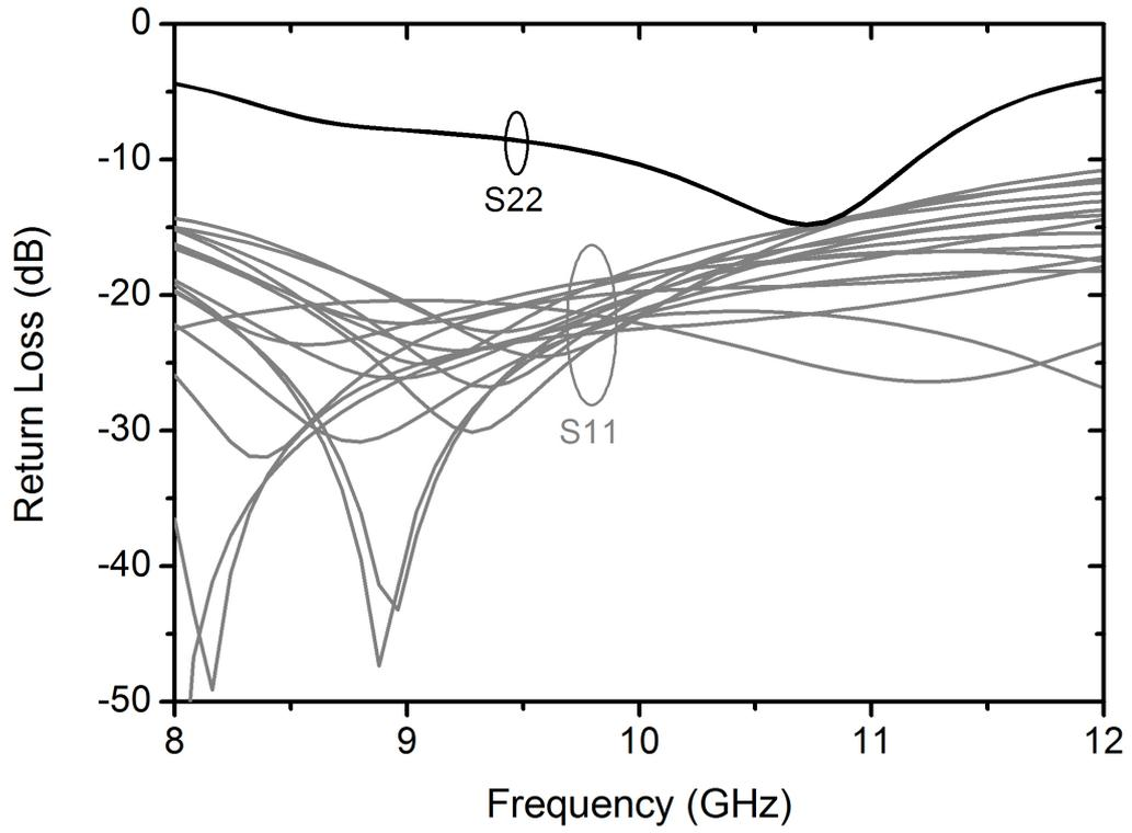
**Figure 70:** Simulated input and output return losses of the T/R module in the transmit mode for all phase states.
