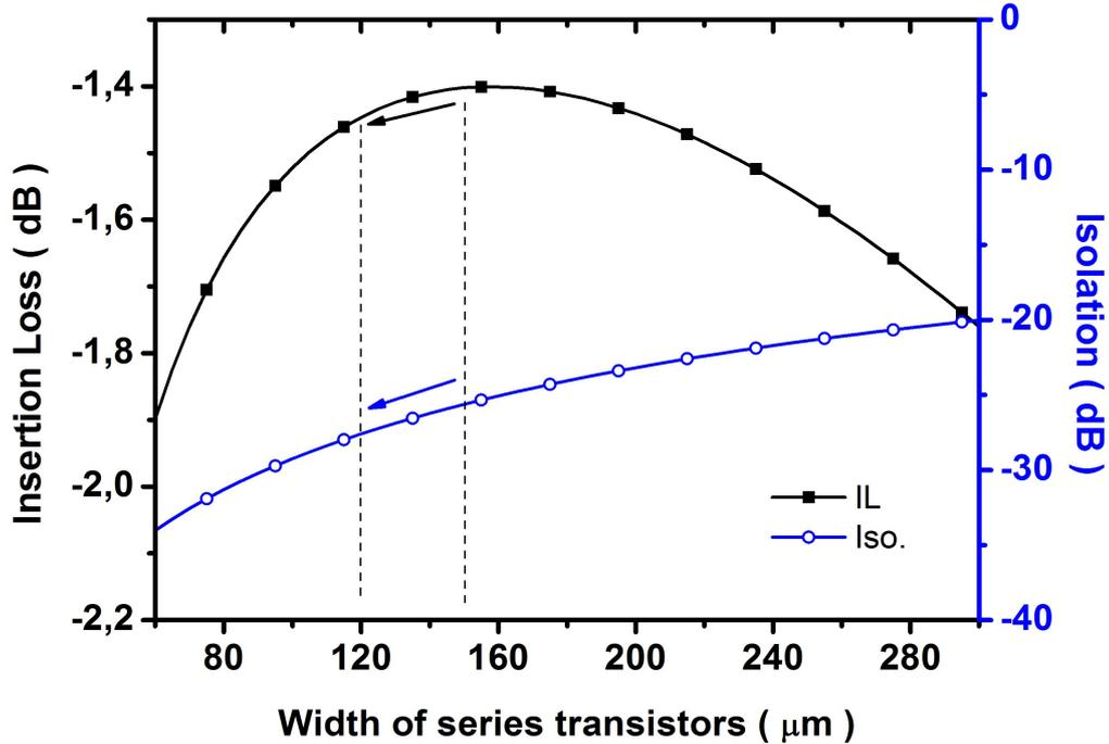
**Figure 28:** Simulated series transistor width versus insertion loss and isolation.
