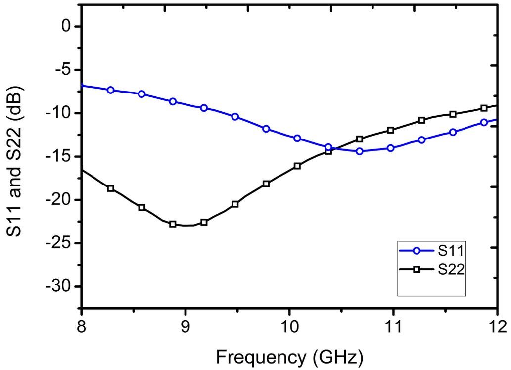
Figure 39: Measured return losses of the S-MSL based T/R switch.
