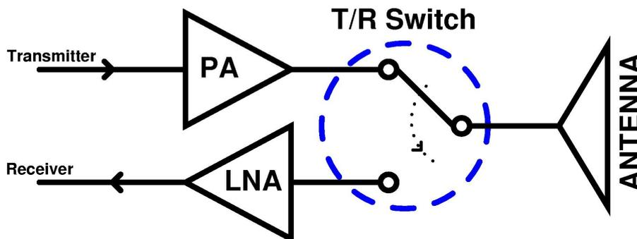
Figure 14: A simple block diagram of T/R module
