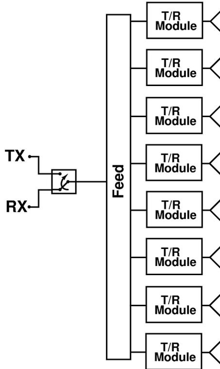
**Figure 4:** Simple block diagram of an active phased array radar.
