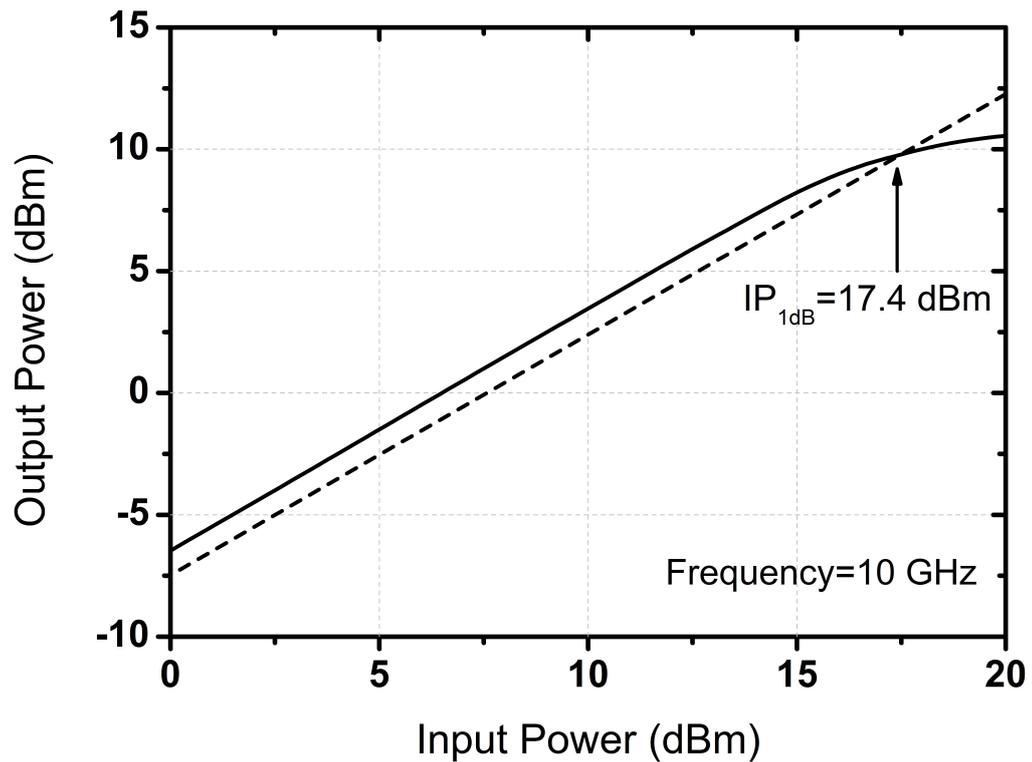
Figure 57: Measured P1dB of the LNA in bypass mode.
