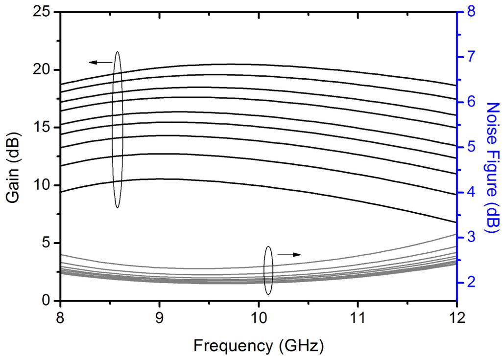
**Figure 68:** Simulated variation of the gain and noise figure of the T/R module in receive mode.
