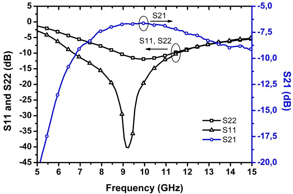
Figure 56: Measured S-parameters of the LNA in bypass mode.
