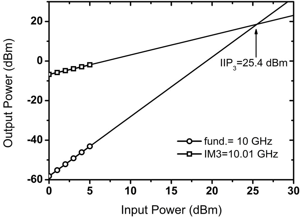
**Figure 58:** Input-referred third-order intercept point (IIP<sub>3</sub>) in bypass mode.
