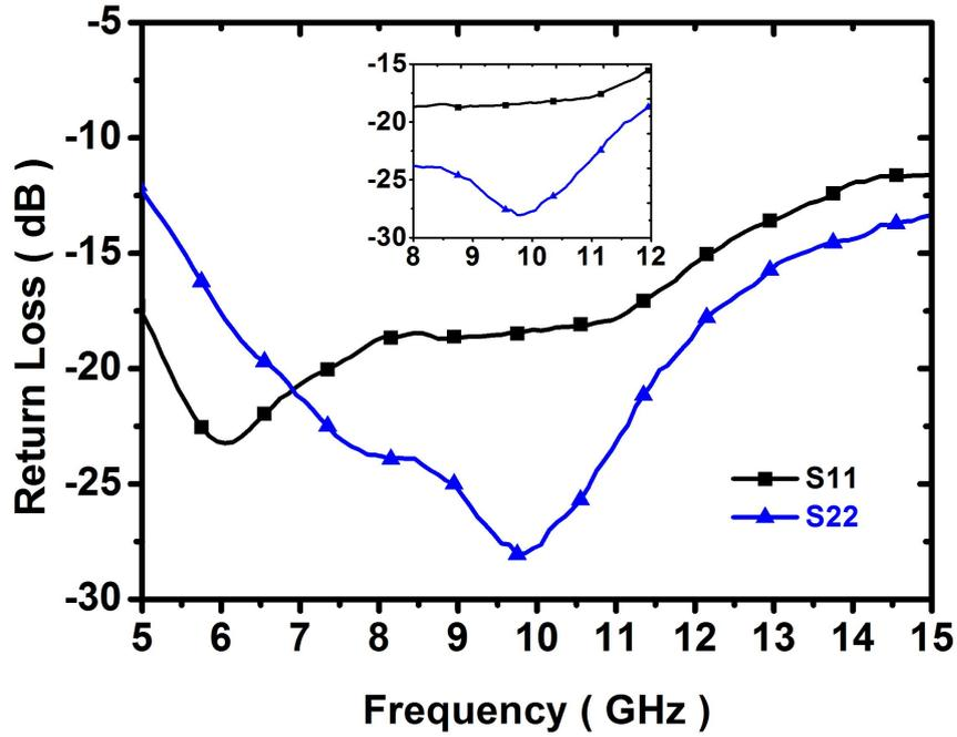
Figure 25: Measured input return loss,  $S_{11}$ , and output return loss,  $S_{22}$  of the T/R switch.
