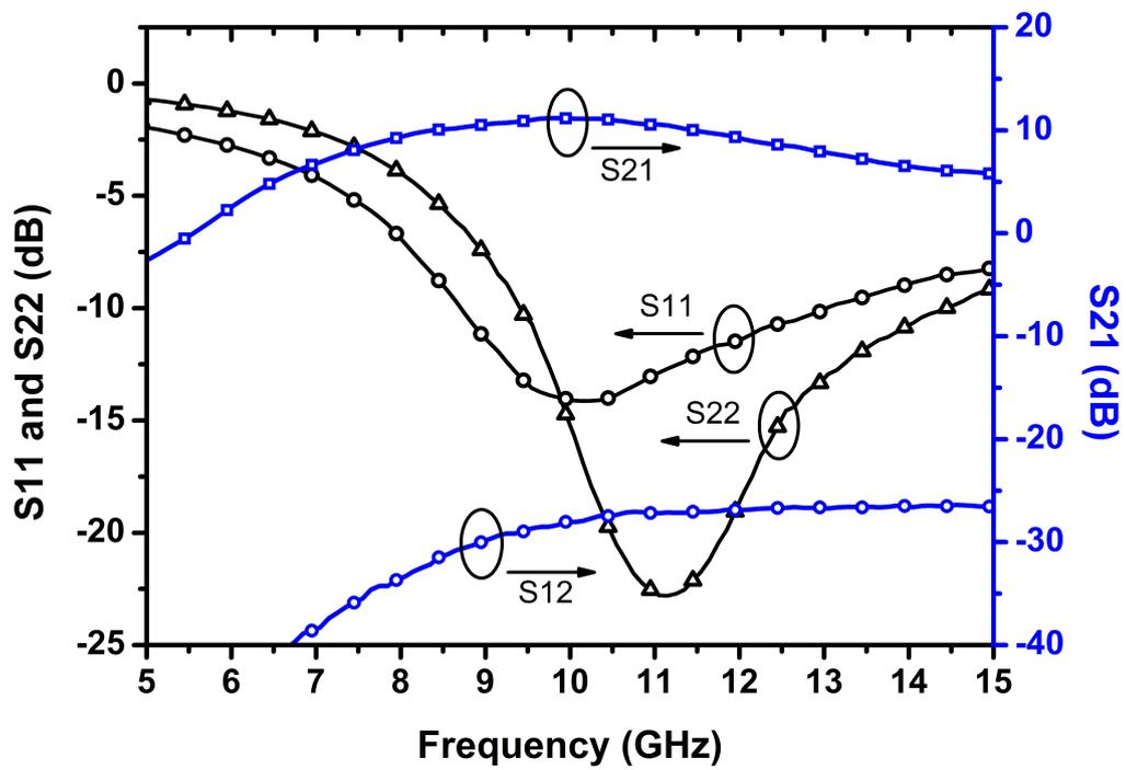
Figure 53: Measured S-parameters of the switched LNA in gain mode.
