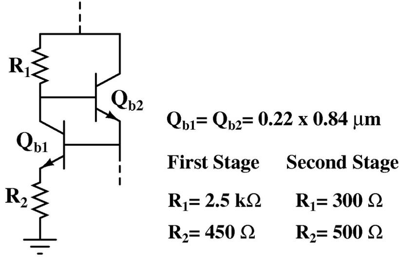
Figure 42: Schematic of the active bias circuit.
