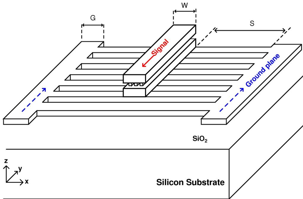
**Figure 35:** Structure of the slow-wave microstrip transmission line (S-MSL).
