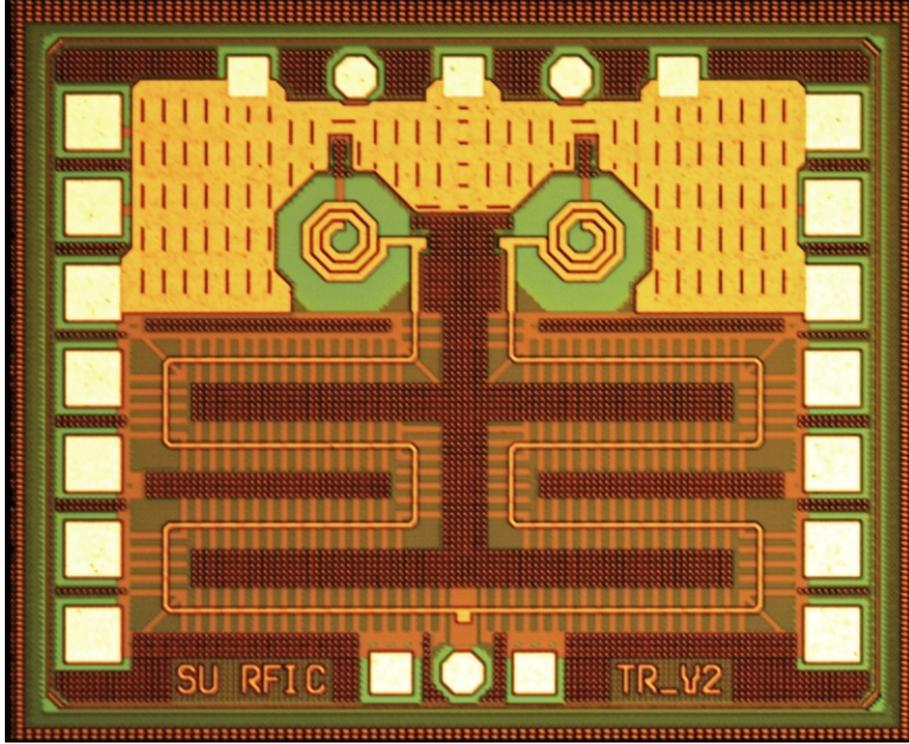
**Figure 37:** Die photo of the DC-20 GHz SPDT switch. The active chip area is  $0.48 \times 0.36 \text{ mm}^2$ .
