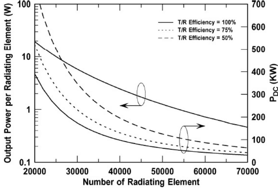
**Figure 8:** Output power per radiating element and total DC power required for all of the T/R modules versus number of elements for a fixed power-aperture-gain product [24].
