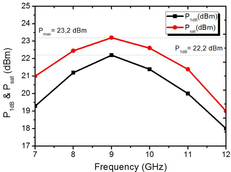
**Figure 13:** Measured saturated output power and the output referred  $P_{1dB}$ .
