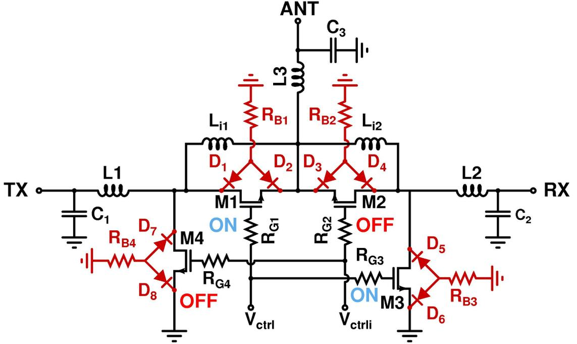
Figure 22: The switch core with body floating technique in TX mode.
