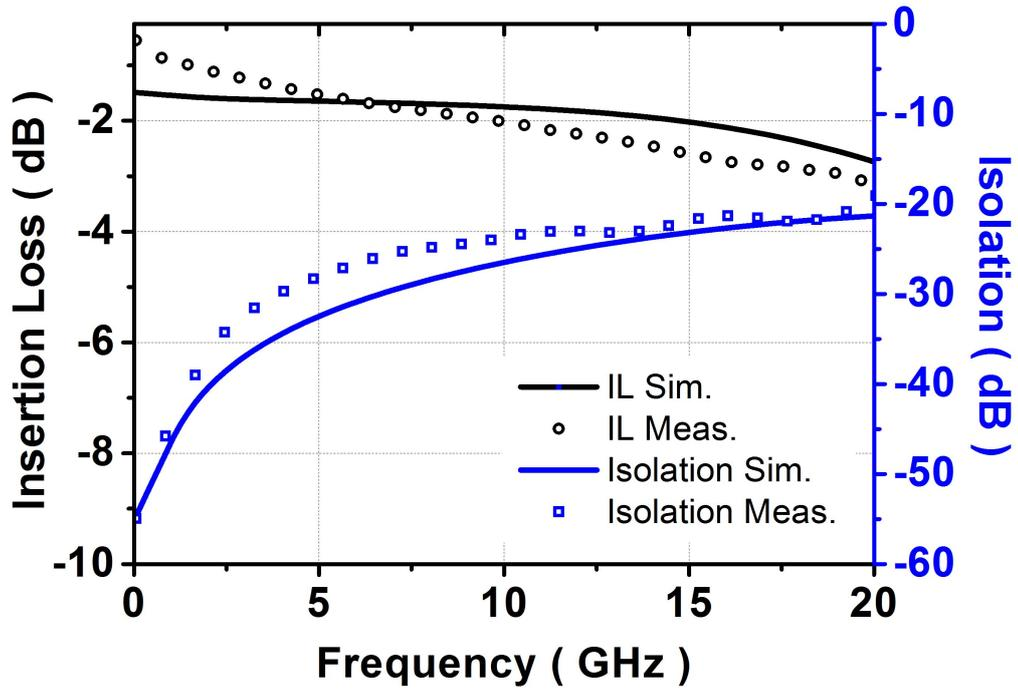
Figure 30: Measured insertion loss and isolation of the SPDT switch.
