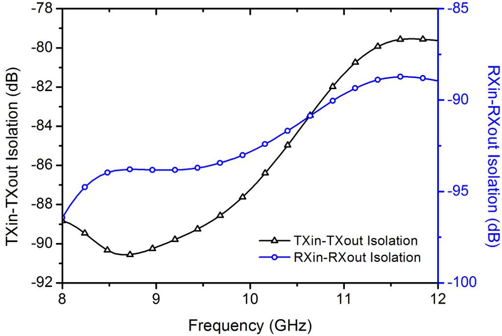
Figure 72: Simulated isolation of the transmit and receive modes.
