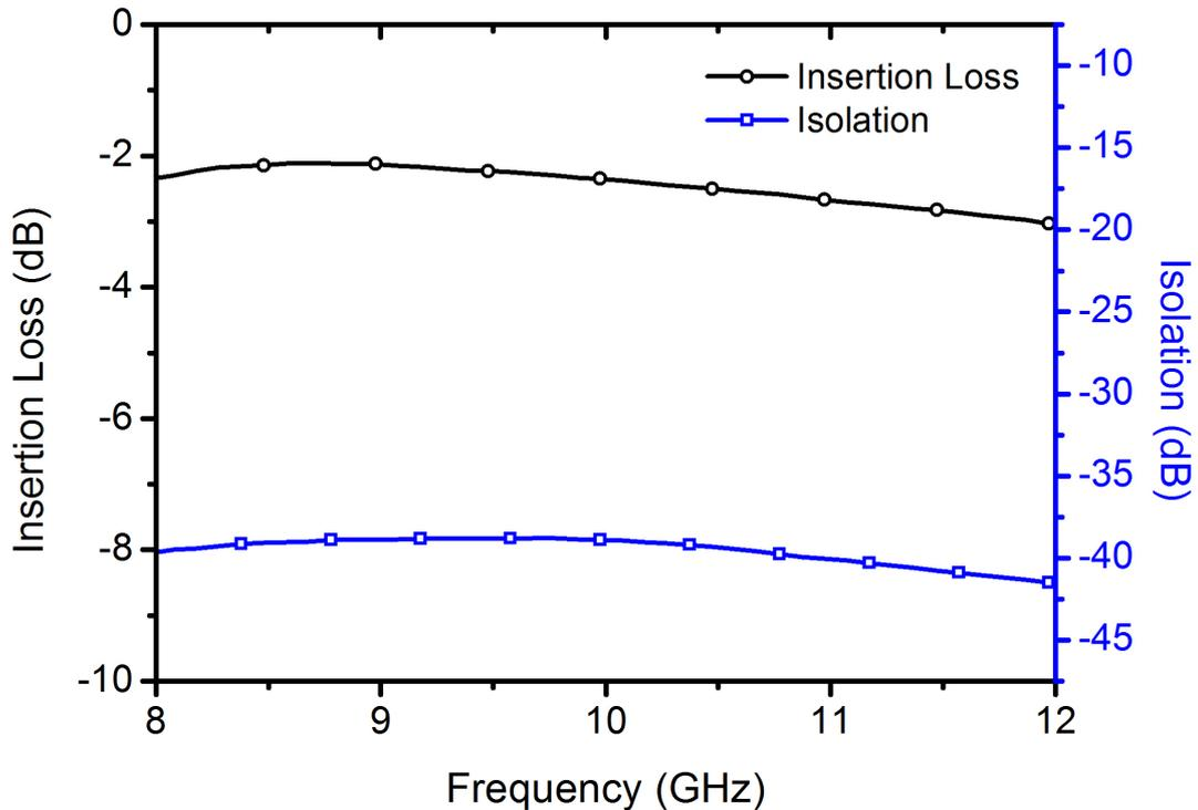
**Figure 38:** Measured insertion loss and isolation of the S-MSL based T/R switch.
