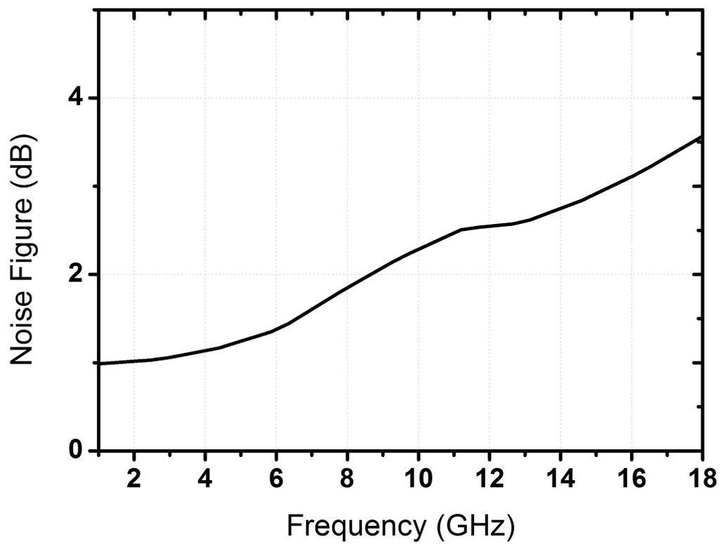
Figure 33: Measured noise figure of the SPDT switch.
