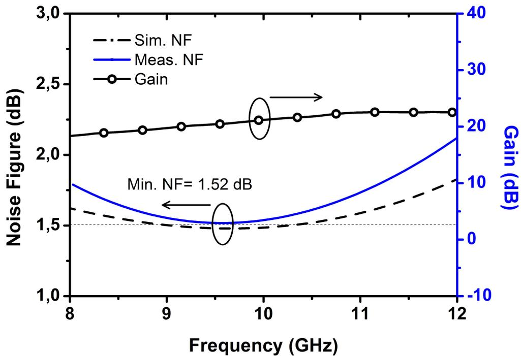
Figure 46: Measured noise figure and gain of the LNA across X-Band.
