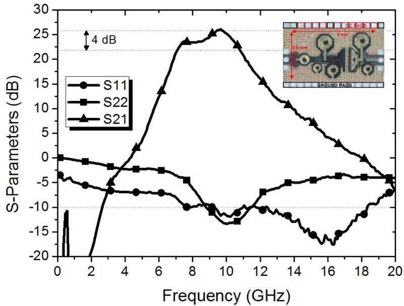
**Figure 12:** Measured small-signal gain and return loss of the two-stage power amplifier.
