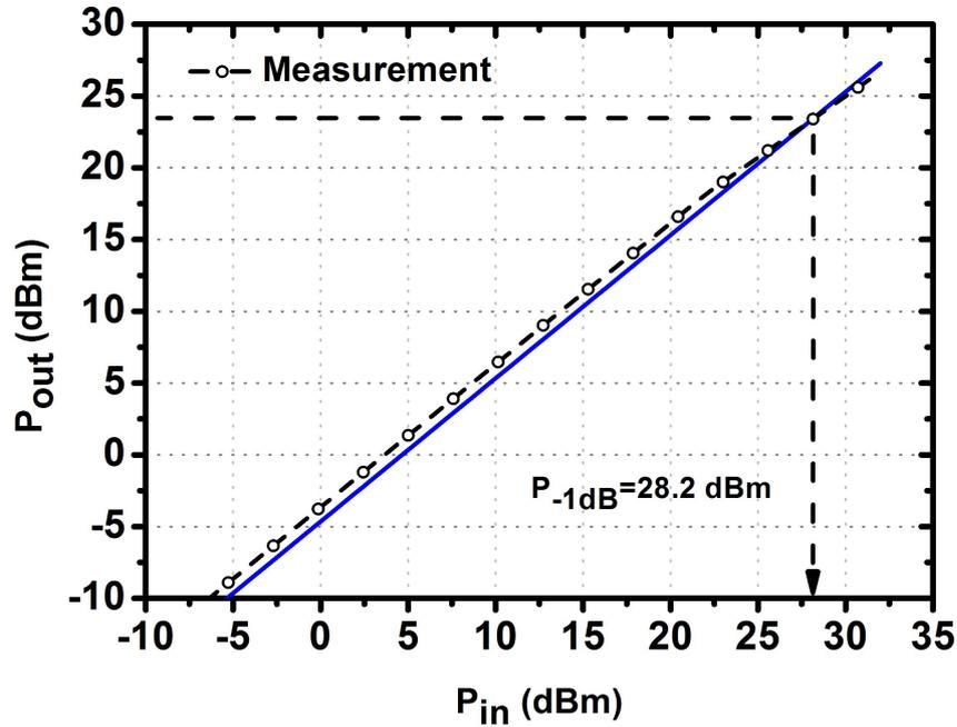
Figure 26: Measured 1 dB compression point ( $IP_{1dB}$ ) of the switch at 10 GHz.
