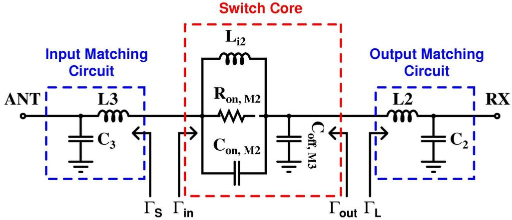
Figure 17: Transmit mode small-signal simplified model.
