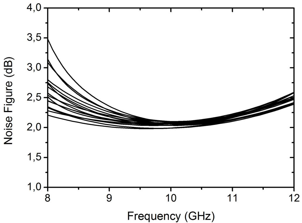
**Figure 65:** Simulated noise figure of the T/R module in the receive mode for all phase states.
