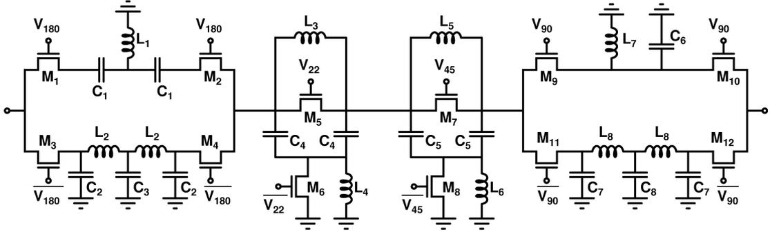
**Figure 60:** Layout of the X-Band T/R Module in IHP 0.25- $\mu\text{m}$  SiGe BiCMOS process.
