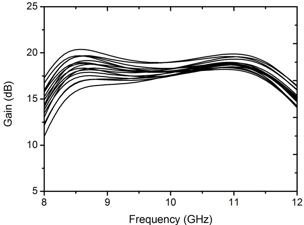
**Figure 69:** Simulated gain of the T/R module in the transmit mode for all phase states.
