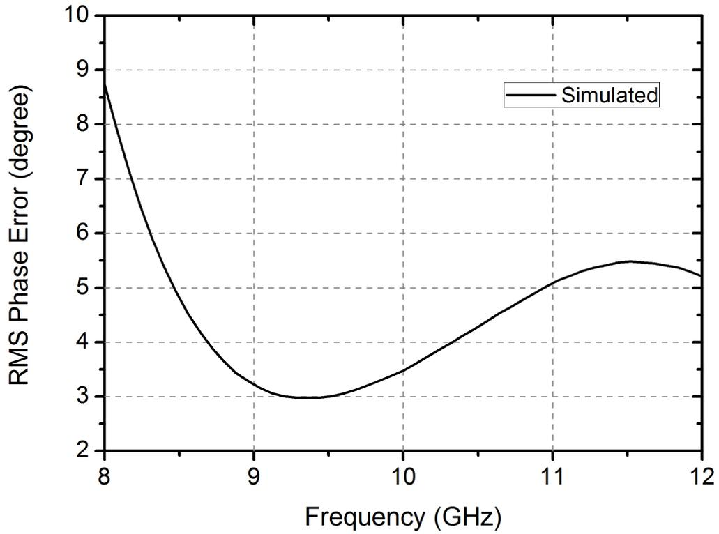
**Figure 67:** Simulated RMS phase error of the T/R module in the receive mode.
