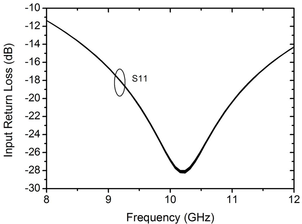
**Figure 63:** Simulated input return losses of the T/R module in the receive mode for all phase states.
