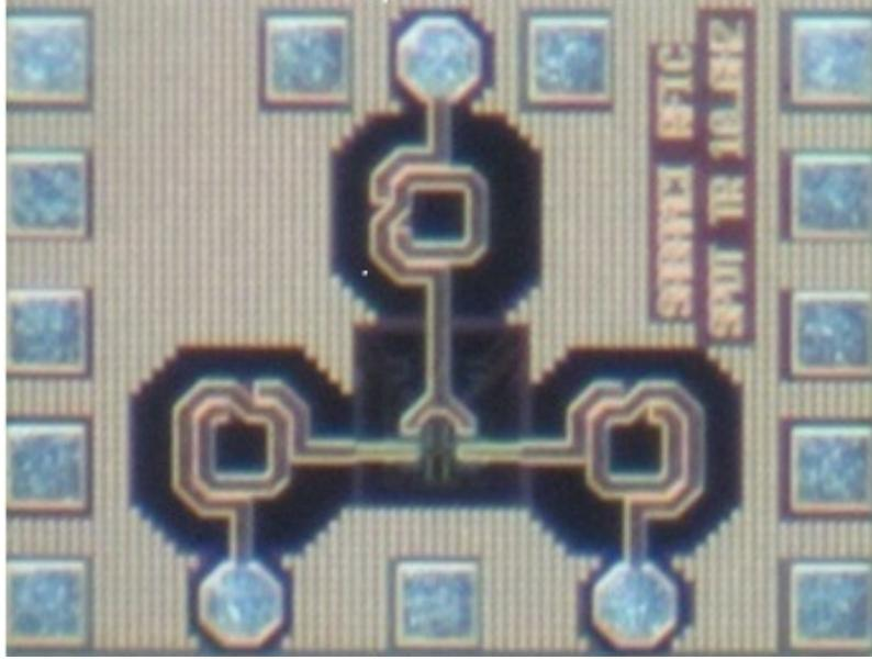
**Figure 29:** Die photo of the DC-20 GHz SPDT switch. The active chip area is  $0.48 \times 0.36 \text{ mm}^2$ .
