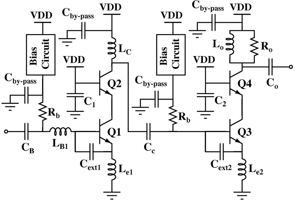
**Figure 41:** Schematic of the designed two-stage low noise amplifier.
