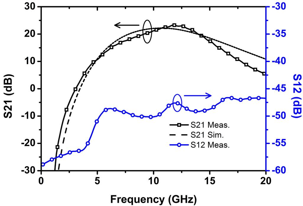
Figure 45: Measured  $S_{21}$  and  $S_{12}$  of the LNA (gain and isolation).
