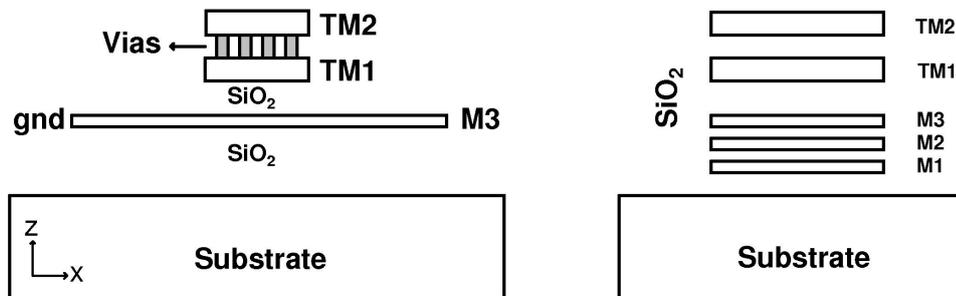
**Figure 36:** Simplified cross-section of the slow-wave transmission line and metal layers in the technology.
