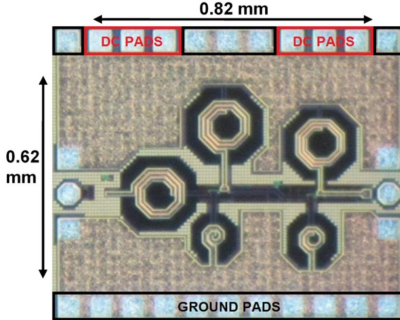
**Figure 43:** Micrograph of the X-Band two-stage low noise amplifier.
