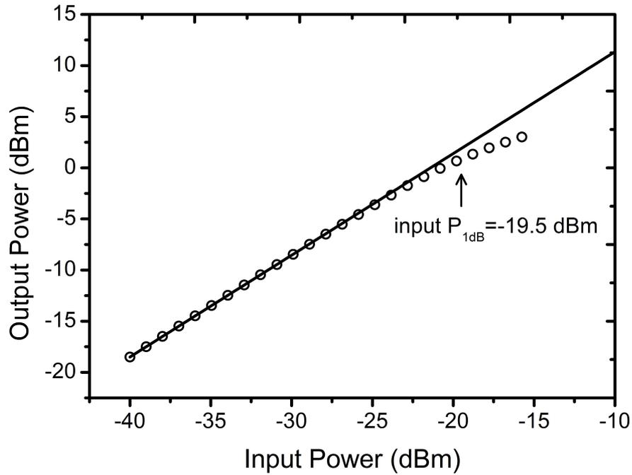
Figure 48: Measured 1-dB compression point of the LNA.
