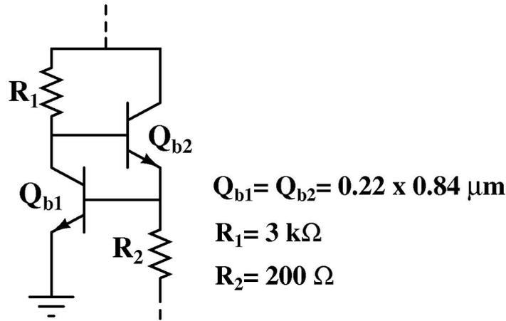
Figure 51: Bias circuit of the switched gain LNA.
