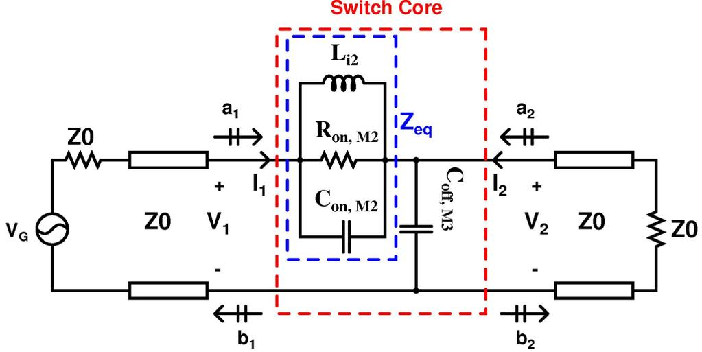
**Figure 18:** Circuit configuration to derive  $S_{21}$  of the ON transistor.
