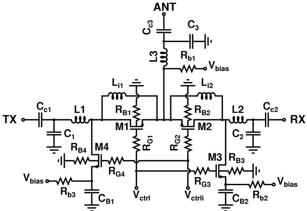
**Figure 15:** Circuit schematic of the designed SPDT T/R switch.
