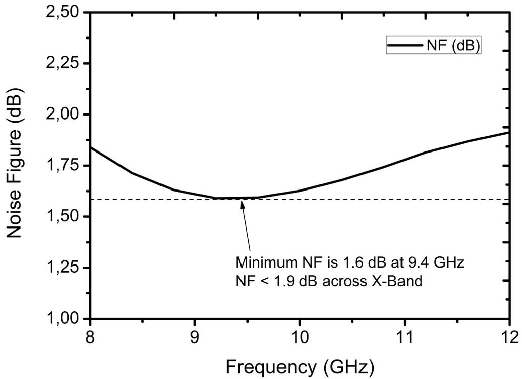
Figure 54: Measured noise figure of the switched LNA in gain mode.
