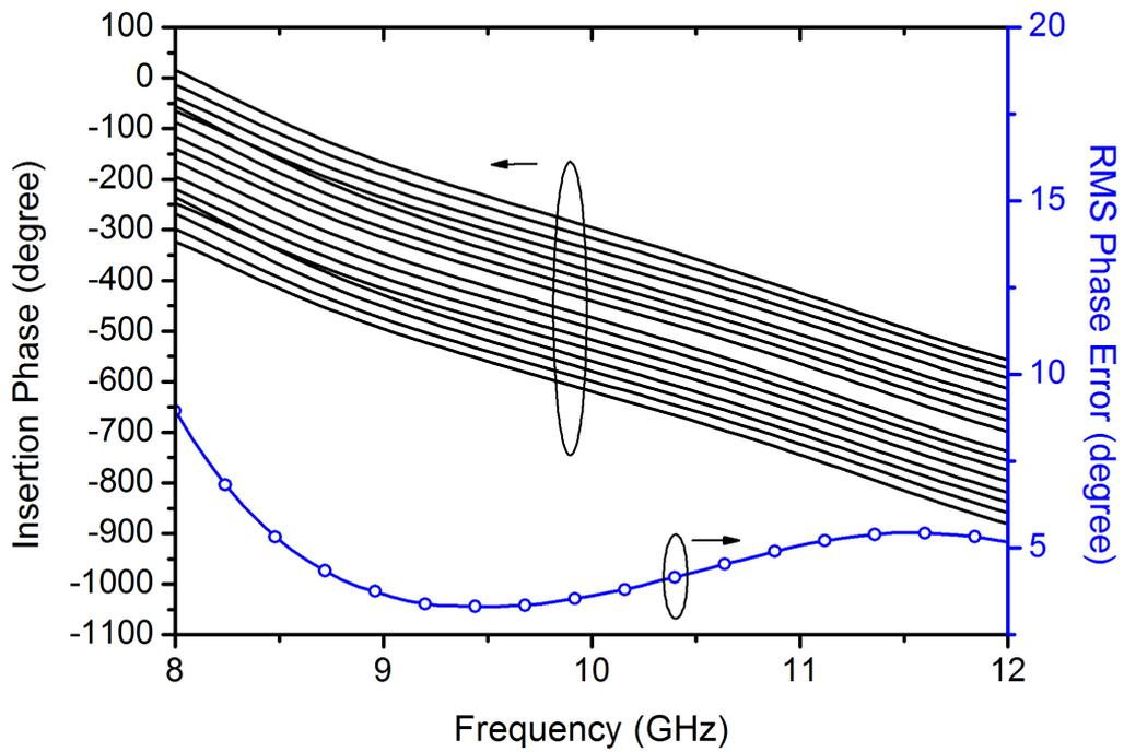
**Figure 71:** Simulated 4-bit phase response and RMS phase error of the T/R module in the transmit mode.
