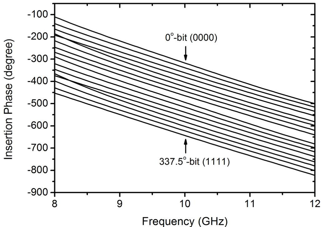
**Figure 66:** Simulated 4-bit phase response of the T/R module in the receive mode.
