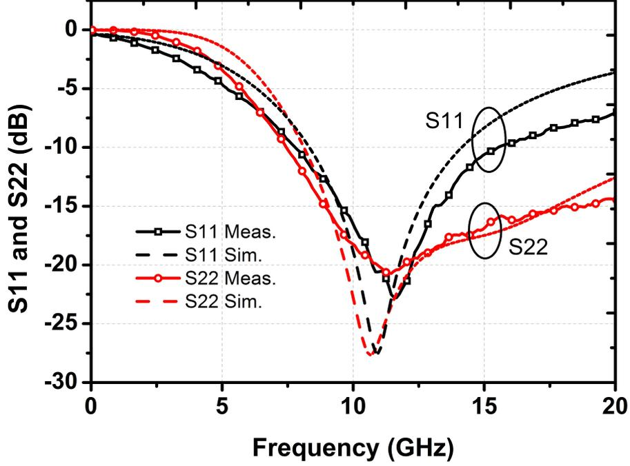
**Figure 44:** Measured  $S_{11}$  and  $S_{22}$  of the LNA (input and output matching).
