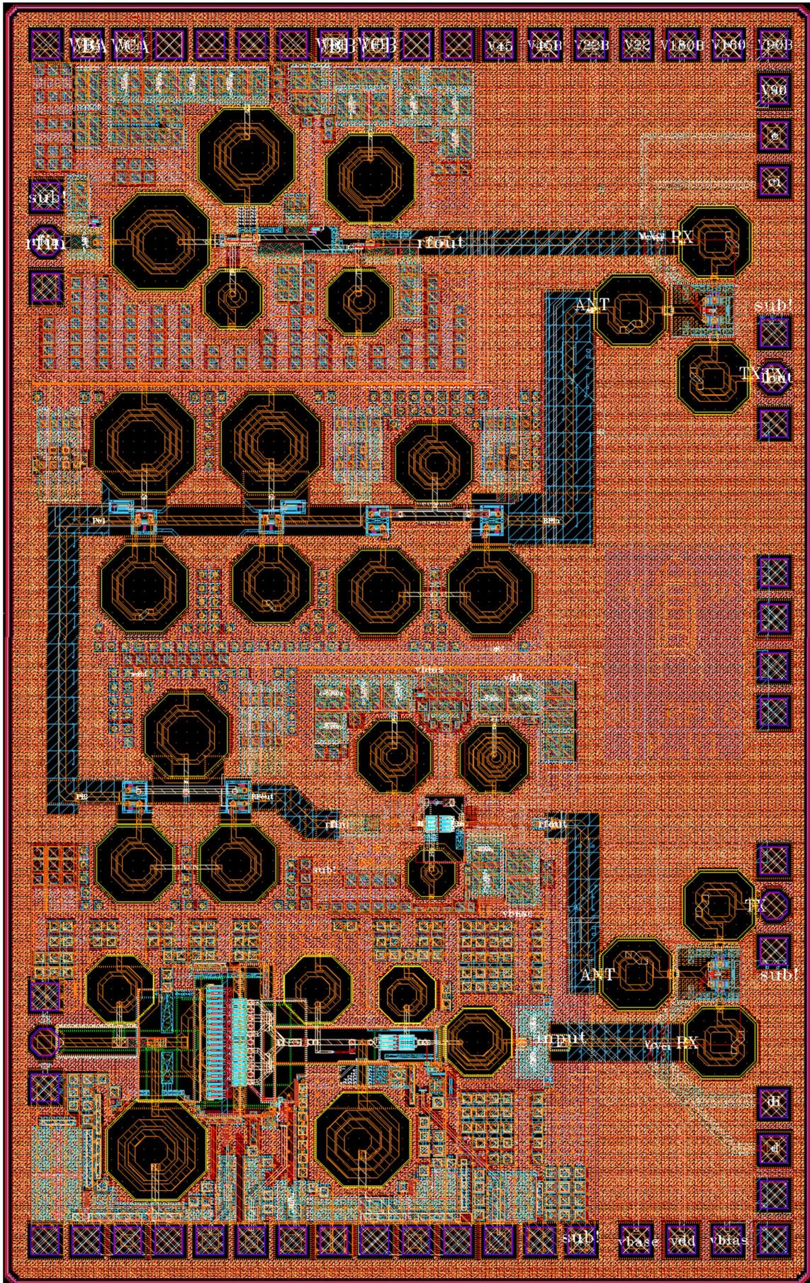
**Figure 61:** Layout of the X-Band T/R Module in IHP 0.25- $\mu\text{m}$  SiGe BiCMOS process.
