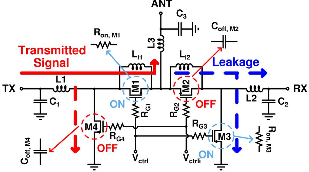
Figure 20: T/R switch in the transmit mode.
