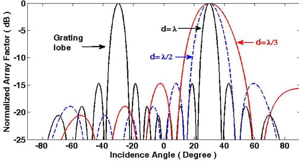
**Figure 2:** Normalized array factor of a 8-element phased array with three different antenna spacing
