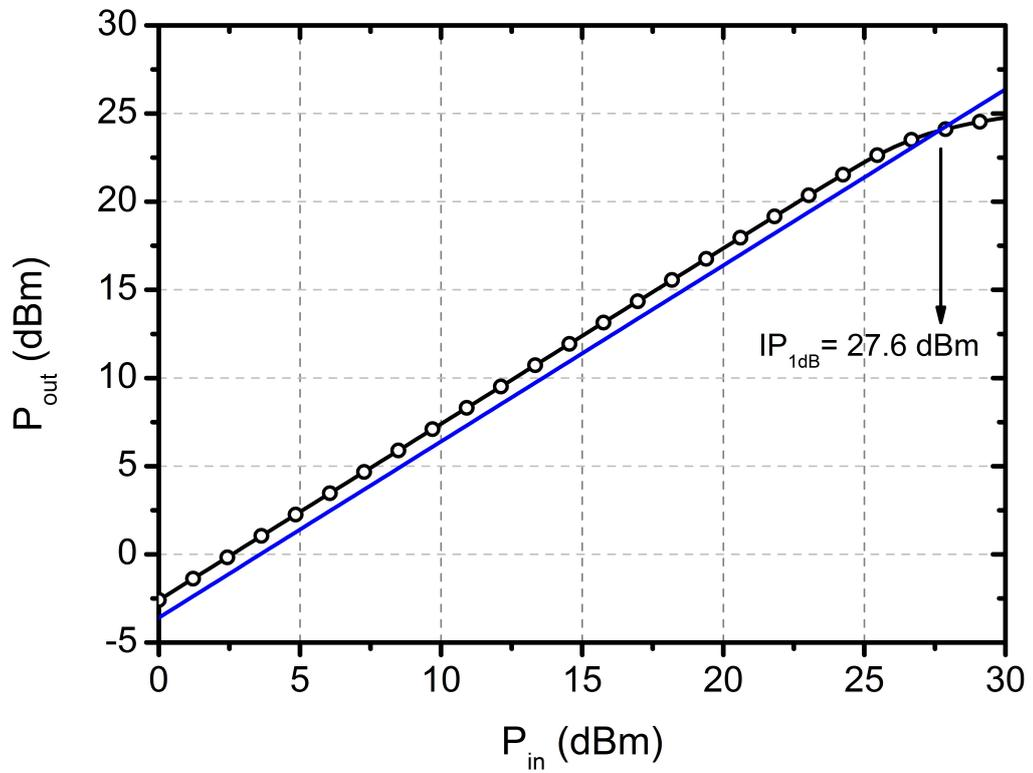
Figure 40: Measured 1 dB compression point ( $IP_{1dB}$ ) of the T/R switch at 10 GHz.
