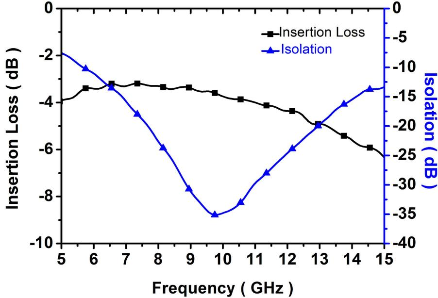
Figure 24: Measured insertion loss and isolation of the T/R switch.
