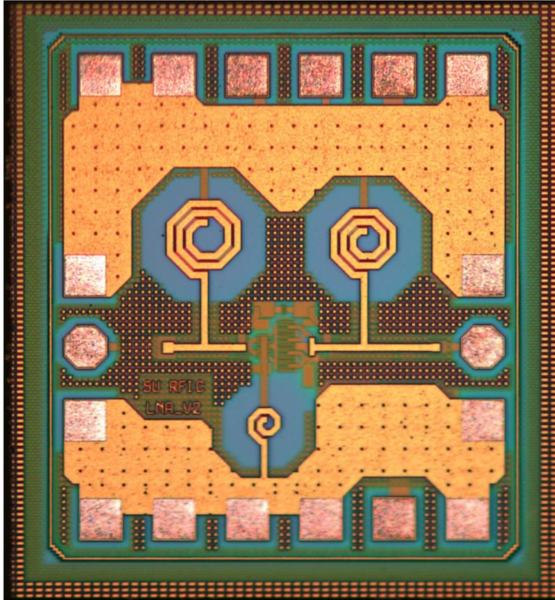
Figure 52: Die photo of the switched gain LNA. The active chip area, without pads, is  $0.52 \times 0.58 = 0.3 \text{ mm}^2$ .
