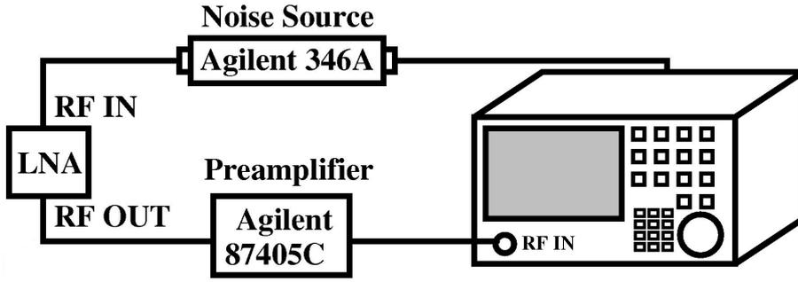
Figure 47: Measurement setup for noise figure.
