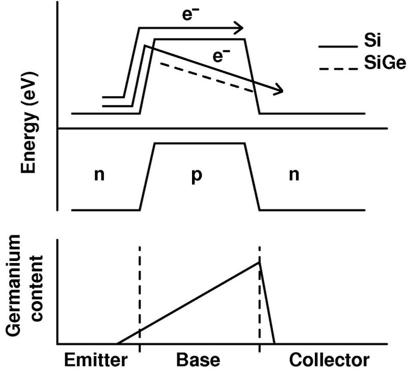
**Figure 9:** Ge concentration (bottom) and band structure (top) of a SiGe HBT. The Ge provides a lower barrier to injection from emitter to base as well as an accelerating field through the base.
