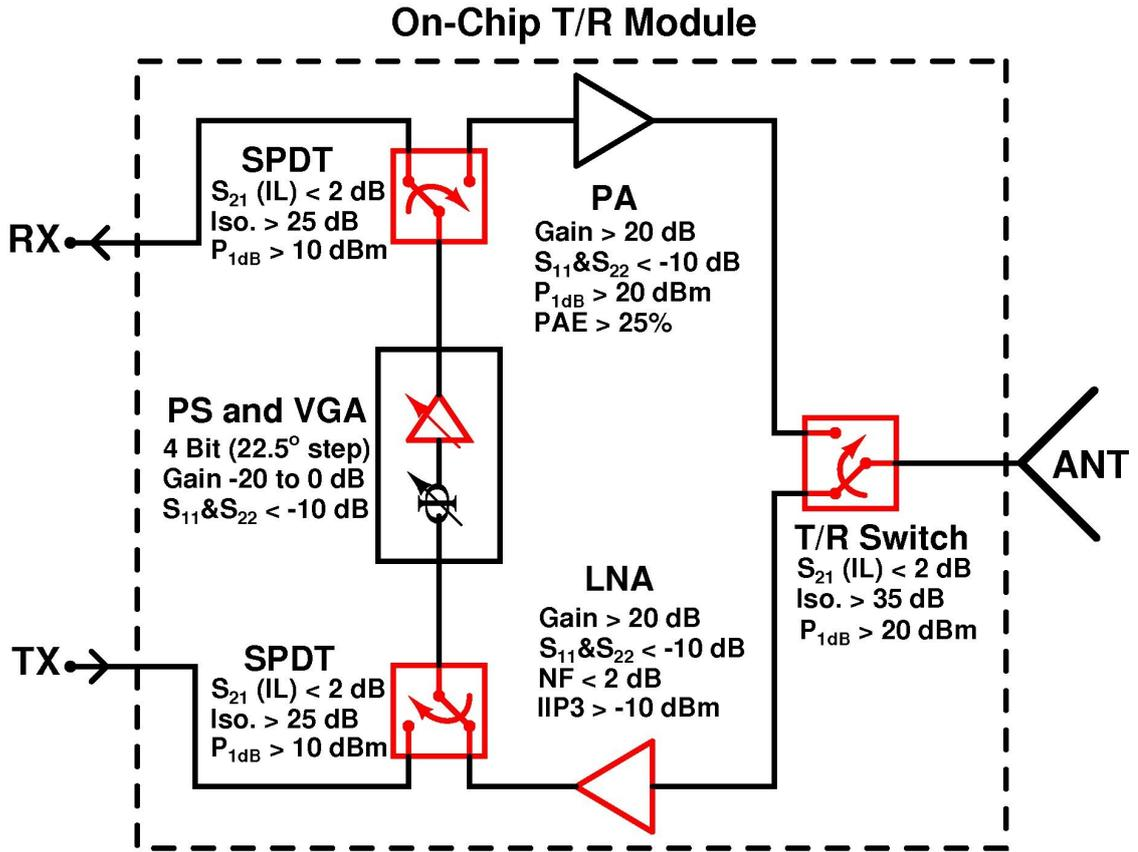
**Figure 10:** SiGe X-Band T/R module system block diagram. The highlighted blocks are the main focus of this thesis.
