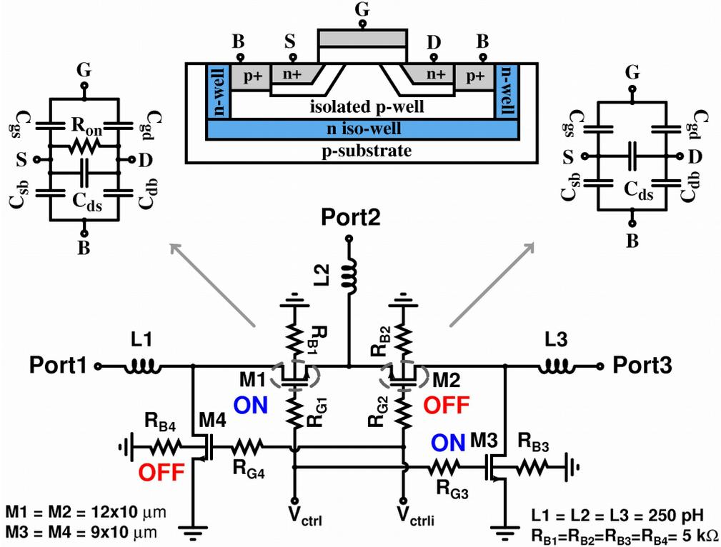
**Figure 27:** Circuit schematic of the designed SPDT switch and cross-sectional view of a typical isolated NMOS transistor.
