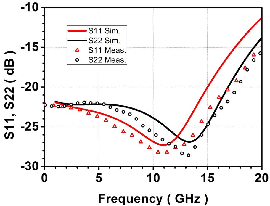
Figure 31: Measured and simulated return loss of the SPDT switch.
