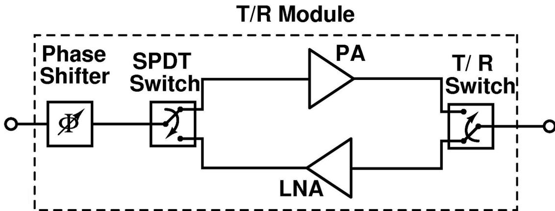
Figure 6: Simple block diagram of a solid state T/R Module
