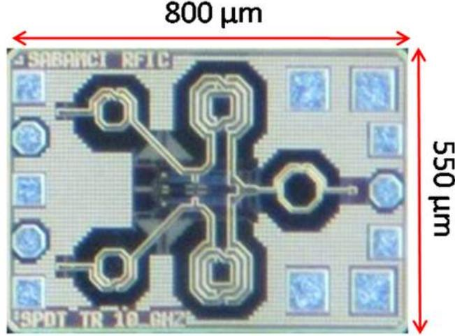
**Figure 23:** Die photo of the T/R switch. The chip area including pads is  $0.44 \text{ mm}^2$ .
