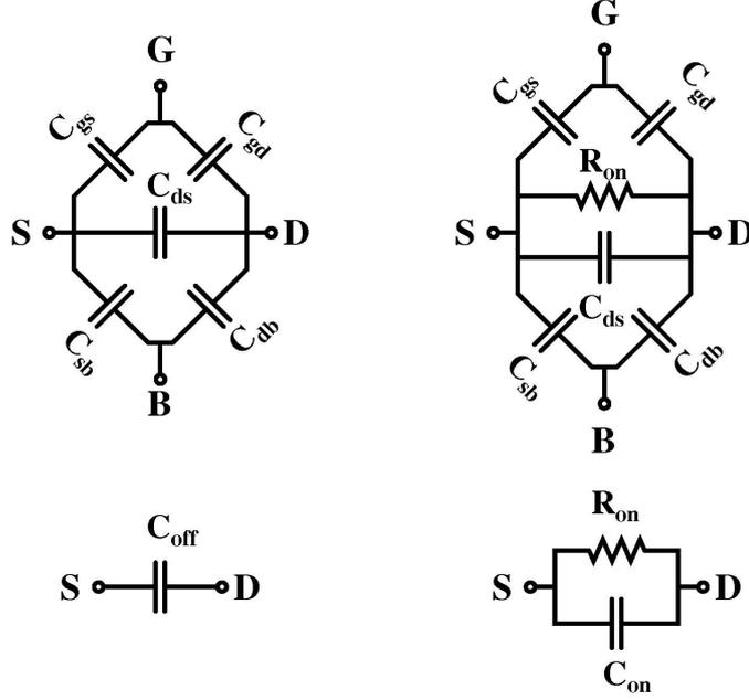
Figure 16: (a) OFF-state Model and (b) ON-state Model of NMOS.
