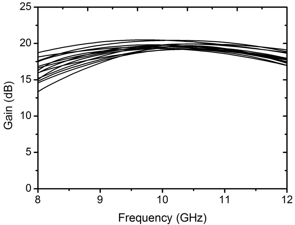
**Figure 62:** Measured gain of the T/R module in the receive mode for all phase states.
