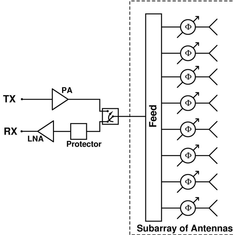
**Figure 3:** Simple block diagram of a passive phased array radar.
