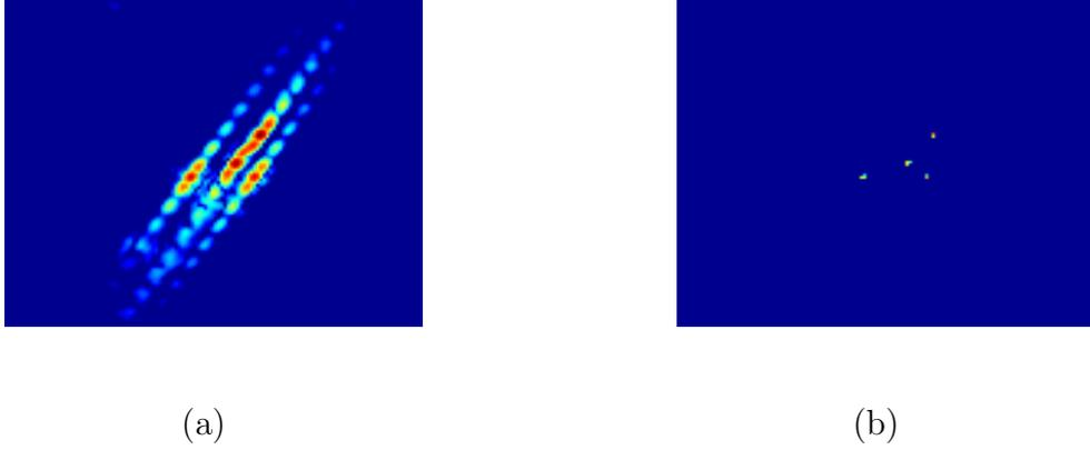
Figure 3.10: Experiments on the Slicy data with 30% frequency band omissions : (a) Conventional imaging from the data without phase error. (b) Sparsity-driven imaging from the data without phase error.
