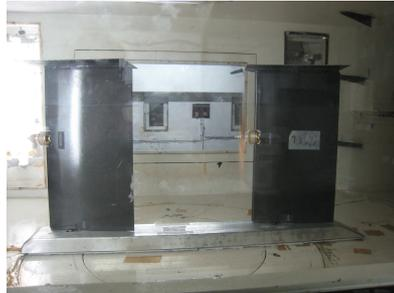
Figure 2.14: Half model in the wind tunnel
