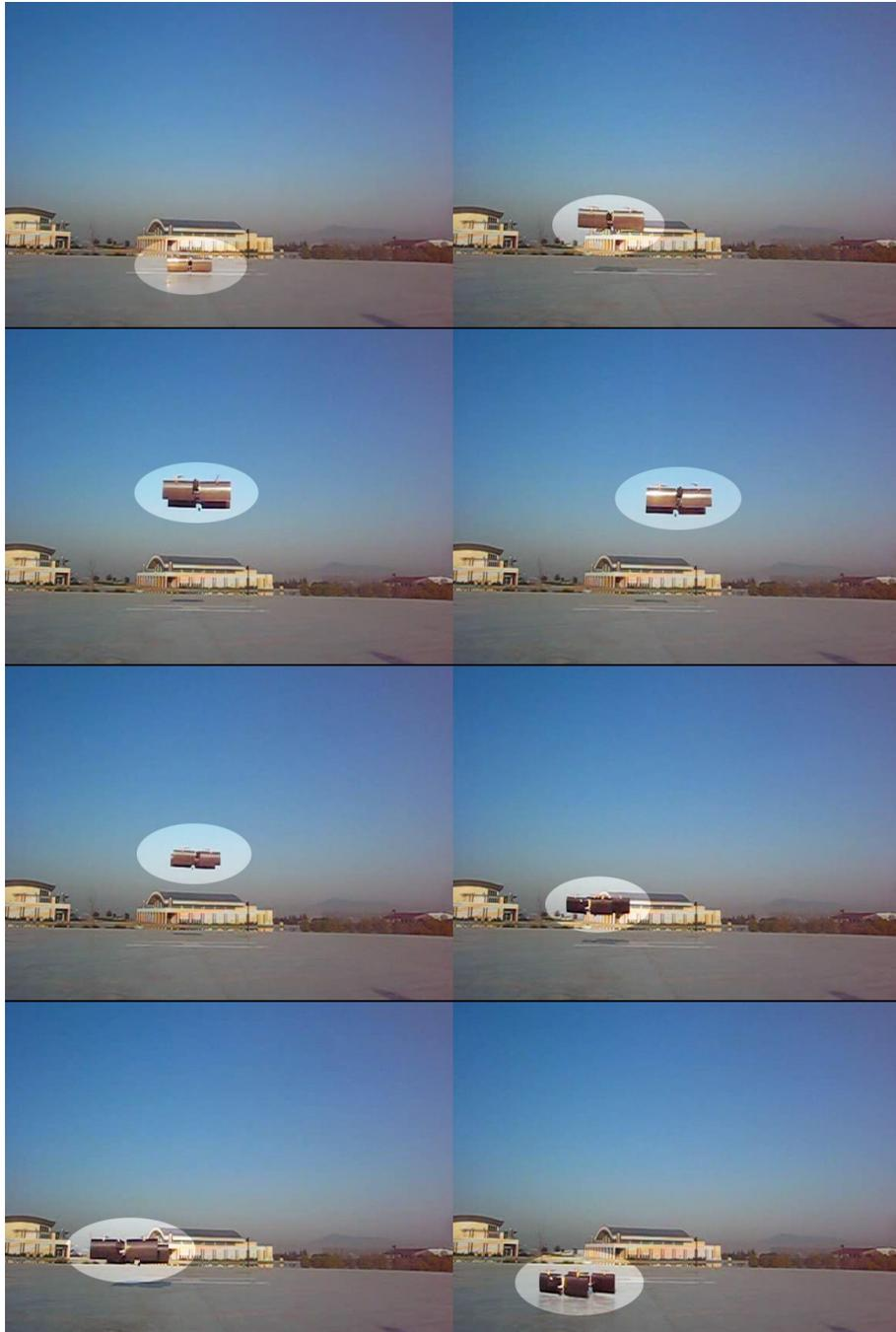
Figure 6.23: Outdoor hover test with SUAVI in helicopter field
