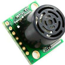
Figure 5.5: Ultrasonic distance sensor used in the system
