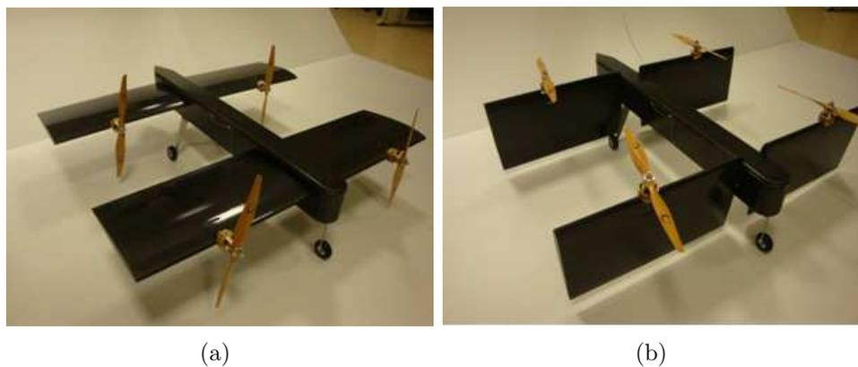
Figure 3.9: SUAVI prototype in horizontal (a) and vertical (b) flight modes
