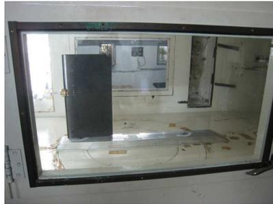
Figure 2.15: Half model with single wing in the wind tunnel
