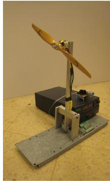
Figure 2.2: The motor test bench
