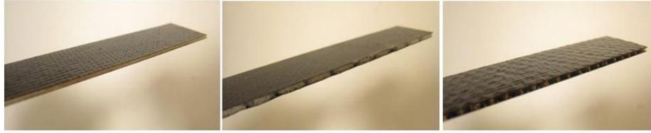
Figure 3.11: Specimens with balsa (a), Aero-mat (b) and Aramid honeycomb (c) core material
