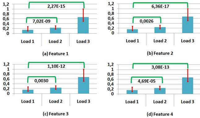
**Fig. 5.** EMG features and p-values of Subject D: (a) Maximum, (b) sum, (c) energy of the signal between the 3000<sup>th</sup> – 5000<sup>th</sup> samples, and (d) energy of the 1500 samples centered around the maximum point of the EMG in a trial.
