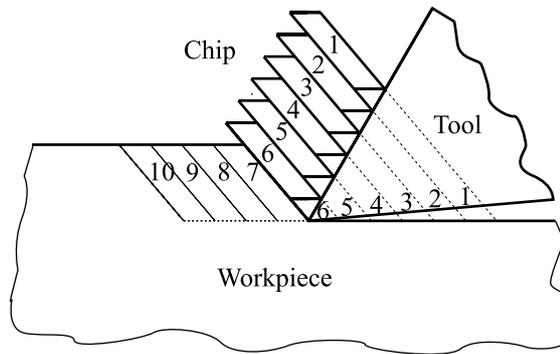
Figure 3. Piispanen's model of chip formation
