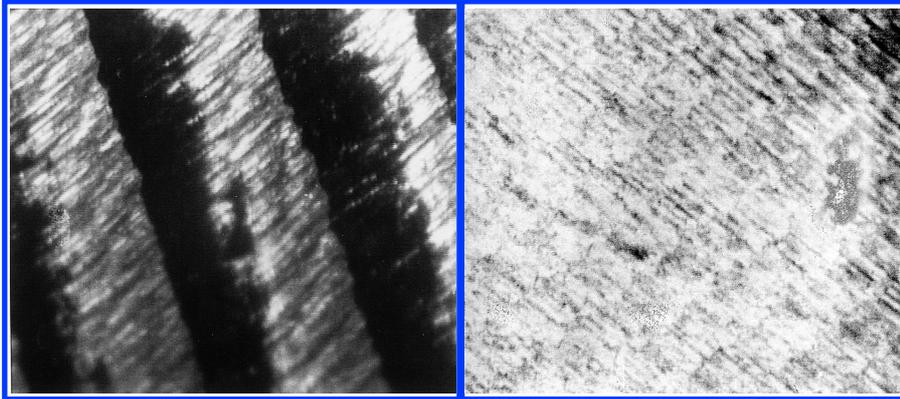
Figure 13. Surface improvement due to variable pitch cutter in Example 2
