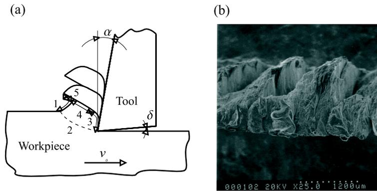
Figure 6. (a) Schematic of the segmented chip formation, (b) SEM image of the segmented chip
