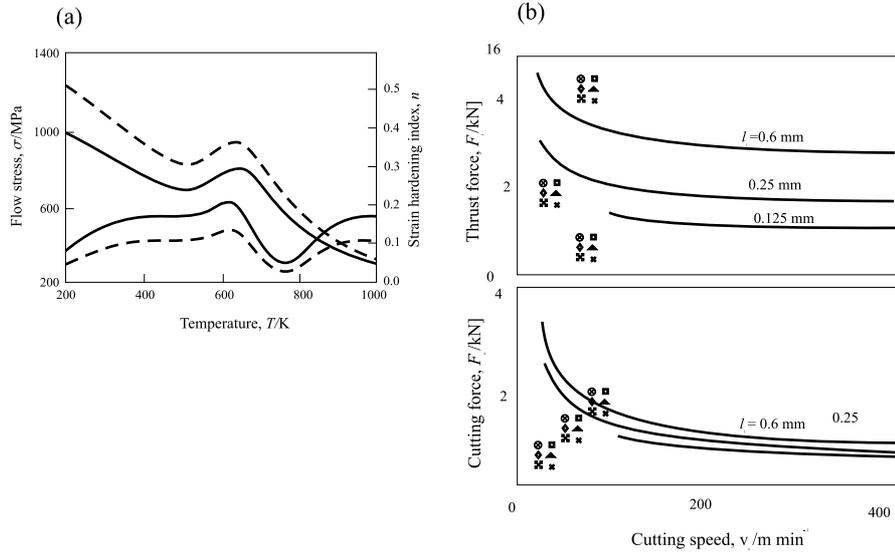
Figure 7. (a) Flow stress versus the chip temperature, (b) Cutting force against the cutting speed [after Hastings, Matthews and Oxley, 1980]
