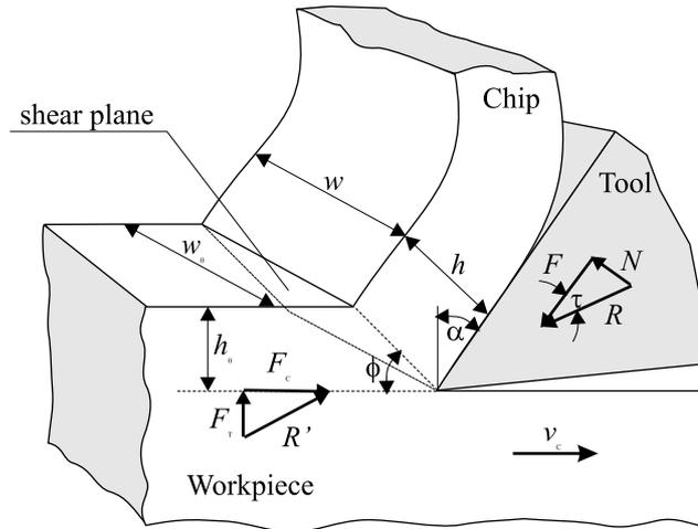
Figure 2. Model of orthogonal metal cutting
