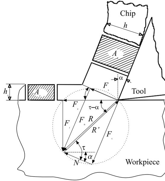
Figure 4. Merchant's force diagram
