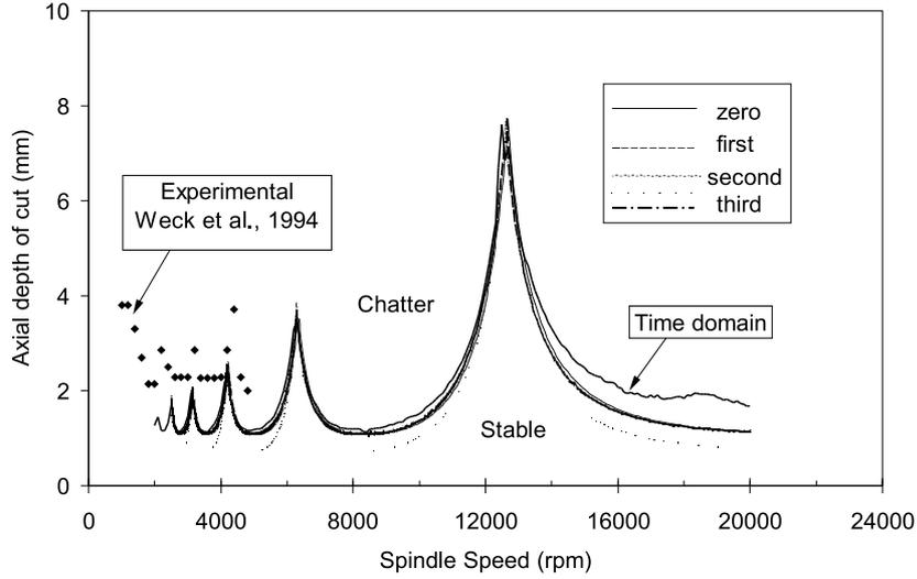
Figure 11. Analytical and experimental stability diagrams for a 2-DOF milling system considered in the example
