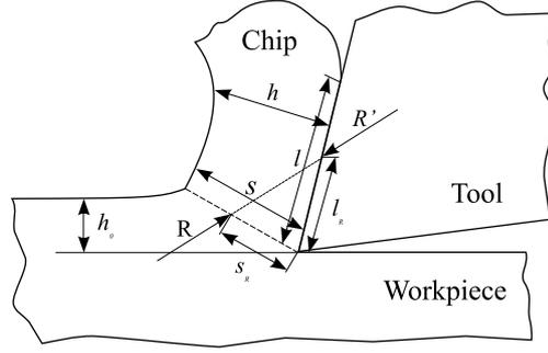
Figure 5. Schematic for calculation of the shear angle,  $\phi$
