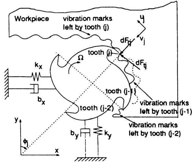
Figure 10. Dynamic model of milling
