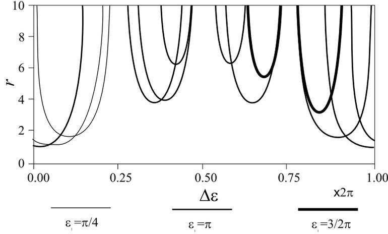
Figure 12. The effect of  $\Delta\varepsilon$  on stability gain for a 4-fluted end mill with linear pitch variation
