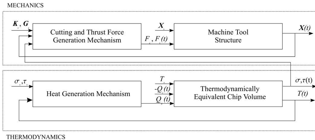
Figure 8. Closed-loop model of dynamic and thermodynamic interaction in the metal cutting system
