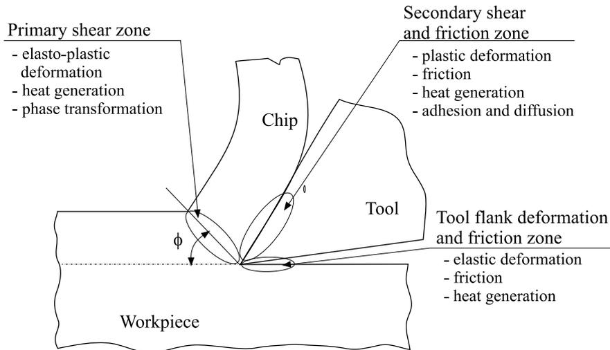
Figure 1. Physical phenomena in the cutting zone
