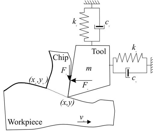
Figure 9. Two degree-of-freedom model of the metal cutting system
