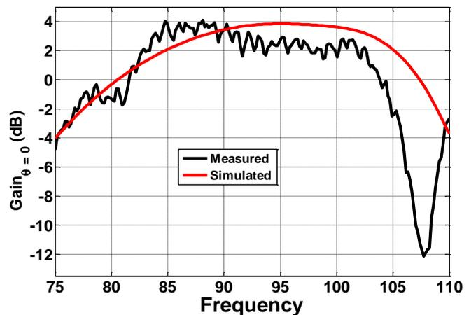
Fig. 9. Measured and simulated antenna gain versus frequency.
