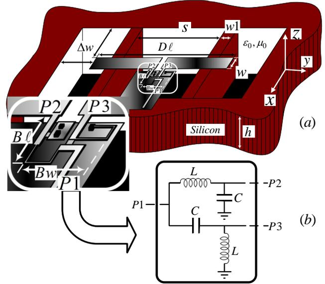
Fig. 1. 3-D schematic of the designed 77 GHz flat dipole antenna and its equivalent lumped circuit for the feeding LC balun.
