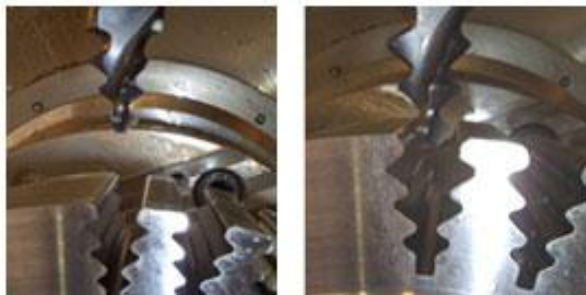
Figure 2.10: Fir tree tool and machining of the turbine blade slots
