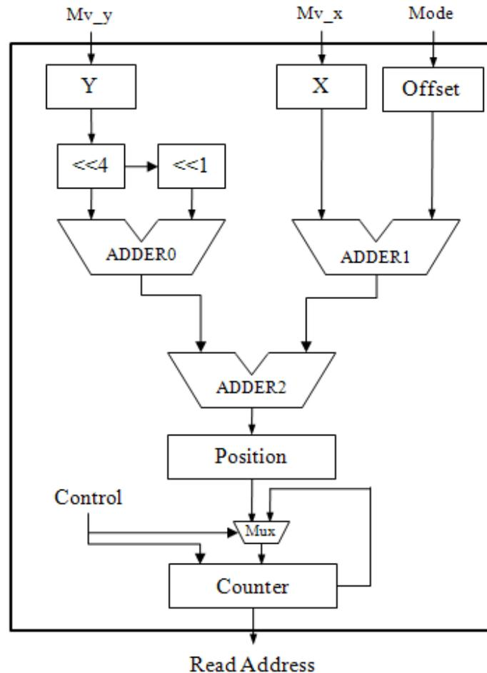
**Figure 3.5** Motion Compensation Hardware
