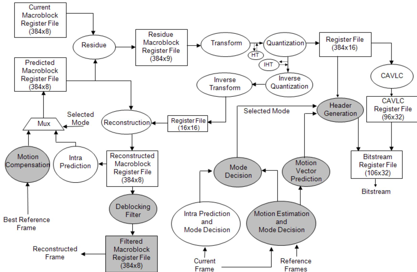
**Figure 3.1** Top-Level Block Diagram of H.264 Video Encoder Hardware
