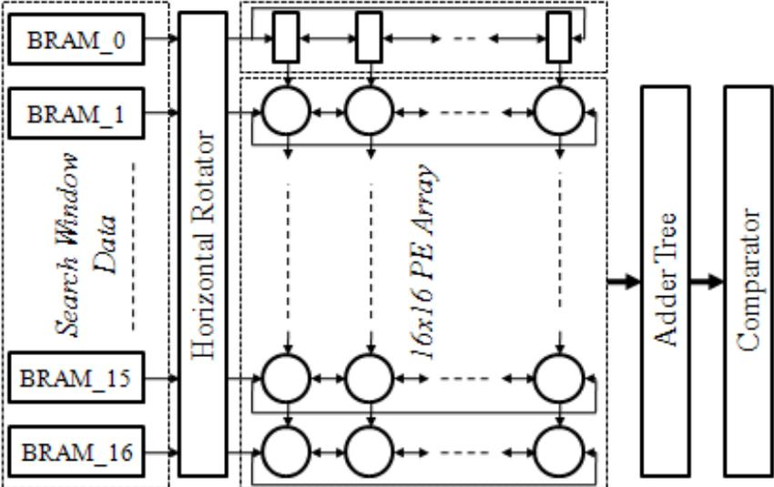
Figure 2.5 256 PE VBS ME Hardware Architecture
