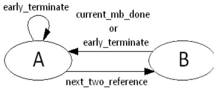
**Figure 2.7** Top Level Control FSM of Parallel Implementation
