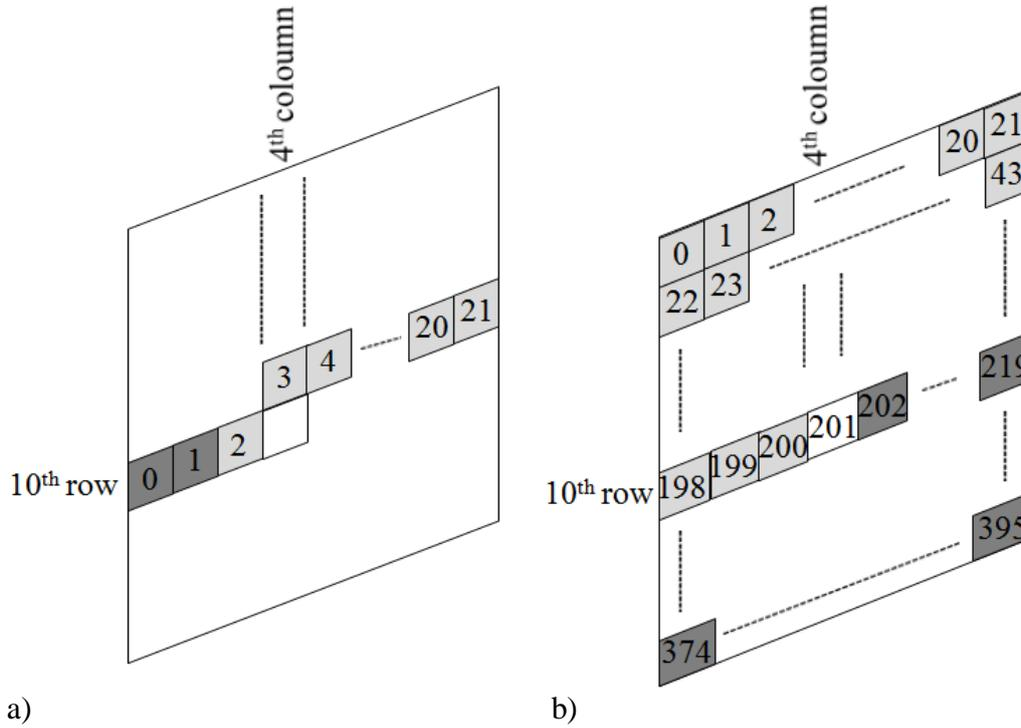
**Figure 2.9** On-chip Memory for Storing BRFs of a) Spatially Correlated MBs b) Temporally Correlated MBs
