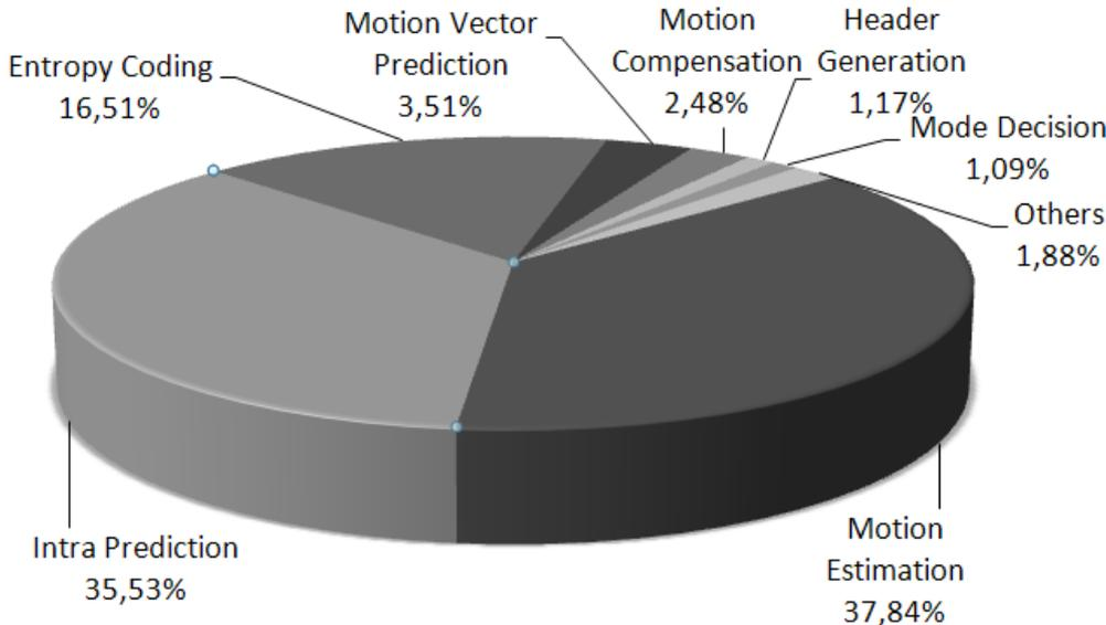
**Figure 3.8** FPGA Slice Usages of H.264 Video Encoder Modules
