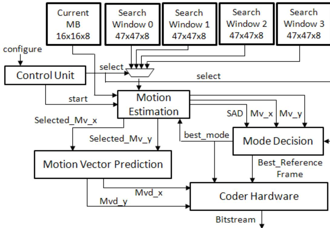
**Figure 3.2** Top-Level Block Diagram of the Motion Estimation, Mode Decision, Motion Vector Prediction and Coder Hardware
