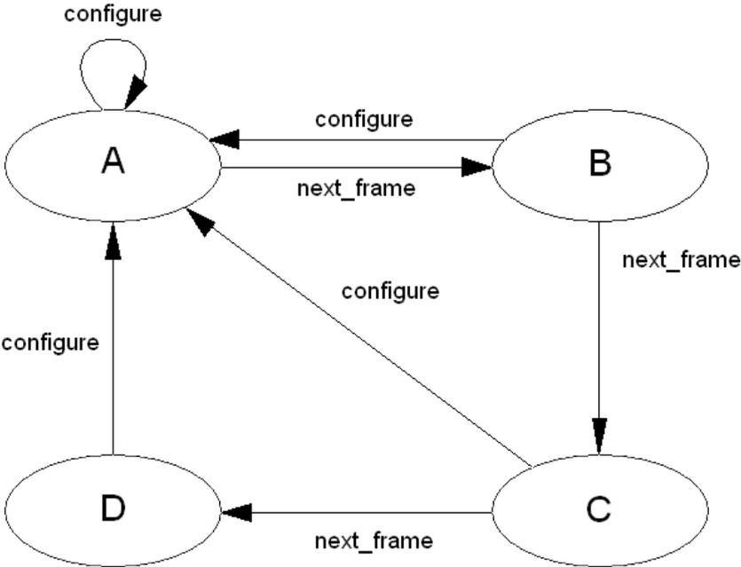
**Figure 3.3** Top-Level FSM of Reconfigurable H.264 MRF Motion Estimation Hardware
