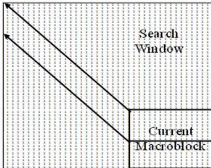
**Figure 3.4** Motion Compensation of Current MB for 16x8 Mode
