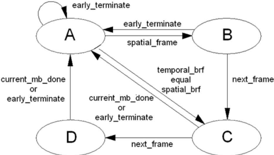
**Figure 2.6** Top Level Control FSM of Serial Implementation
