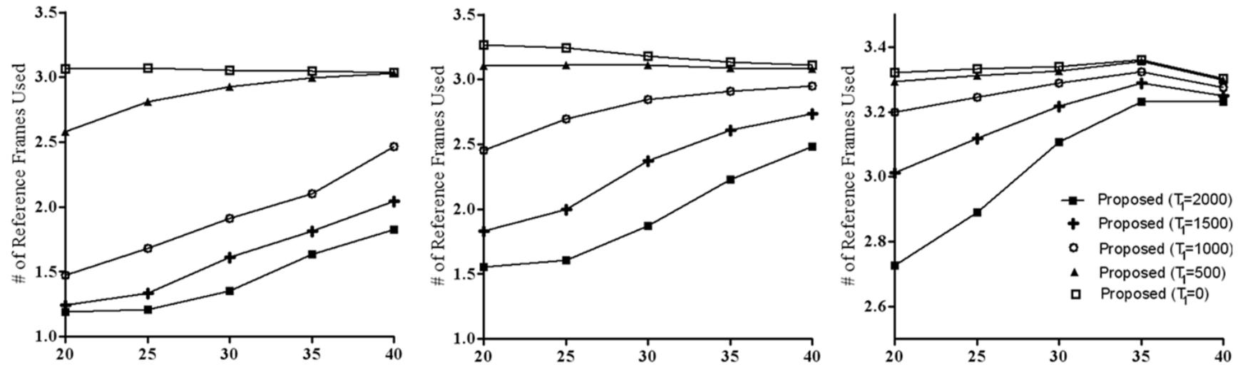
Figure 2.4 Number of Reference Frames Used vs. Quantization Parameter for a) Foreman, b) Akiyo, and c) Mobile
