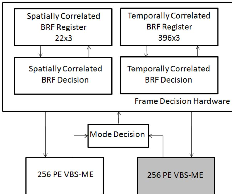
**Figure 2.8** Top Level Block Diagram of Proposed MRF ME Hardware
