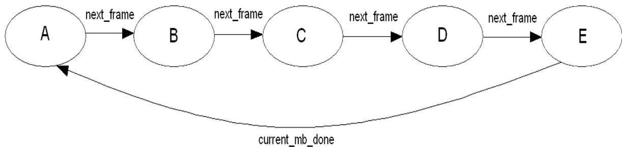
**Figure 2.10** Top Level Control FSM of Ref-5 Hardware
