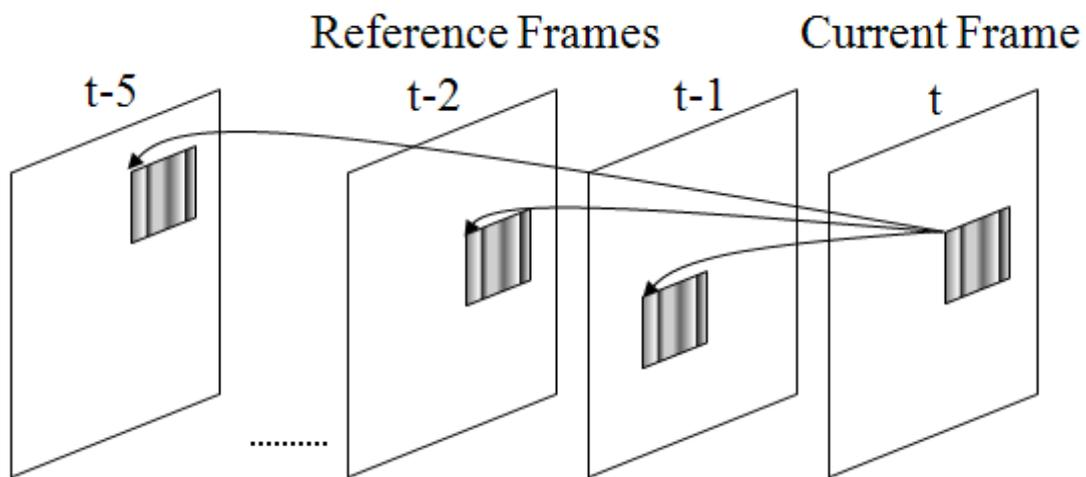
**Figure 2.1** Multiple Reference Frame Motion Estimation
