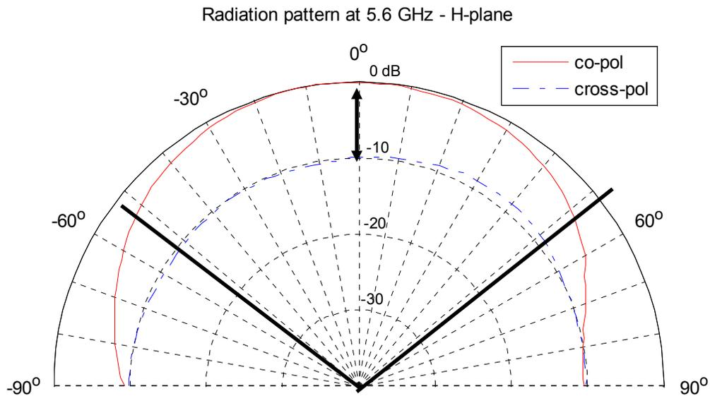
**Fig. 20** H-plane measured radiation pattern at 5.6 GHz for co. pol. and cross polarizations
