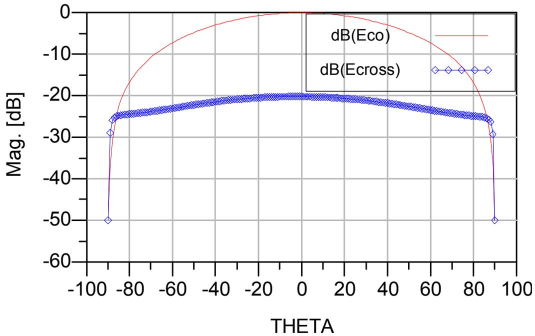
Fig. 10 H-plane radiation pattern at 2.337 GHz for co. pol. and cross polarizations
