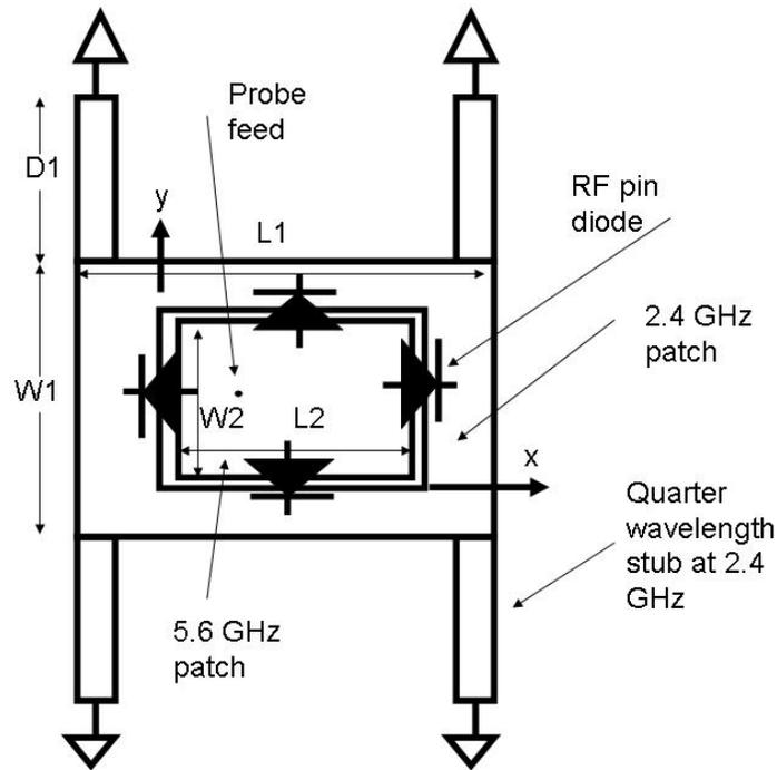
**Fig. 1** Dual band 2.4/5.6 GHz reconfigurable patch antenna
