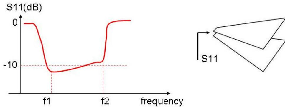
**Fig. 3** An UWB parallel plate TEM antenna operating from  $f_1$  to  $f_2$  frequency
