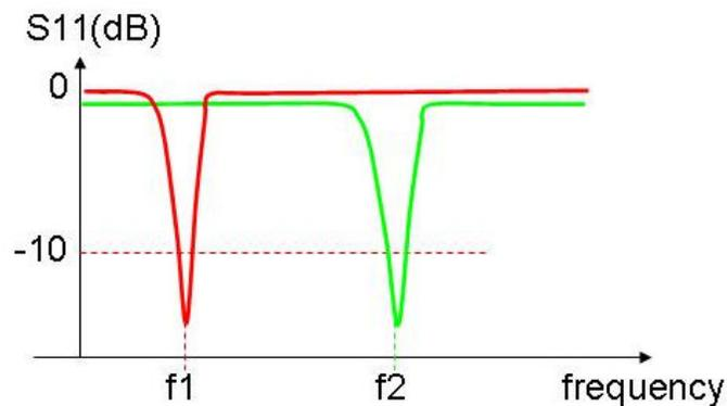
**Fig. 4** Return loss of a reconfigurable antenna with switchable resonances  $f_1$  and  $f_2$
