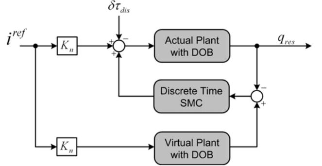
Fig. 5. Model following controller structure
