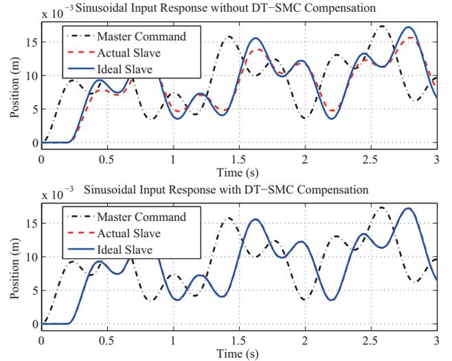
Fig. 7. Environment contact motion with sinusoidal input
