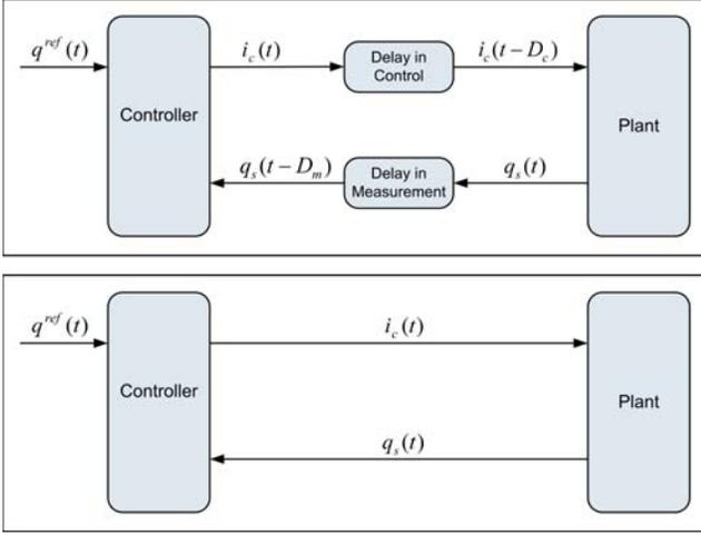
Fig. 2. Structure of system with and without delay
