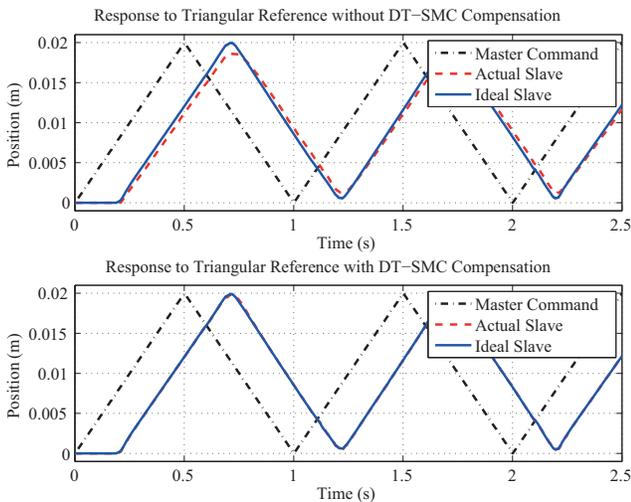
Fig. 9. Environment contact motion with triangular input
