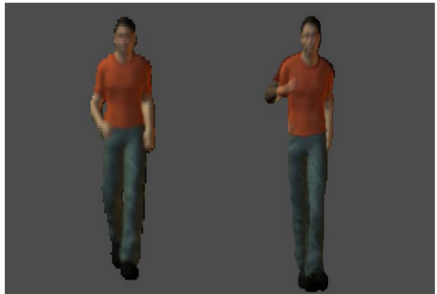
Figure 10. Impostors from different texture maps of equal number of key-frames and memory consumption. The proposed (right) has higher resolution due to re-generated animation frames via image morphing.
