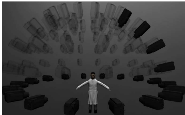
Figure 4. Discrete set of captured 16 by 4 view-points which are uniformly distributed over the surface of a bounding hemisphere.
