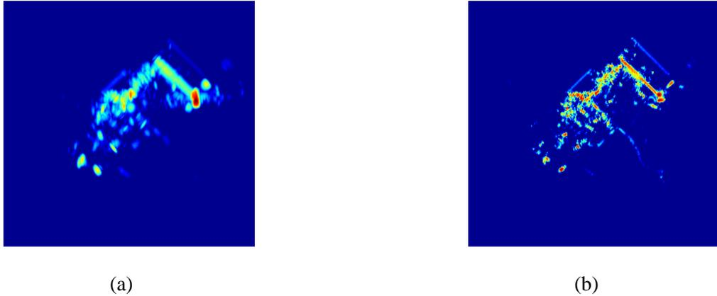
Fig. 7. (a) Conventional imaging from the data without phase error. (b) Sparsity-driven imaging from the data without phase error.
