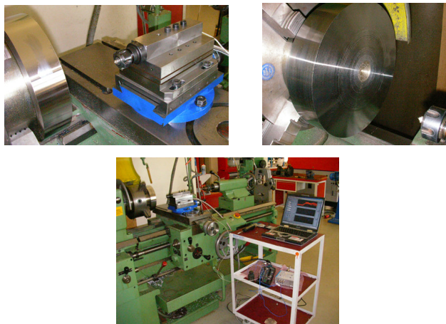
Figure 3.1: The non-cutting test setup.
