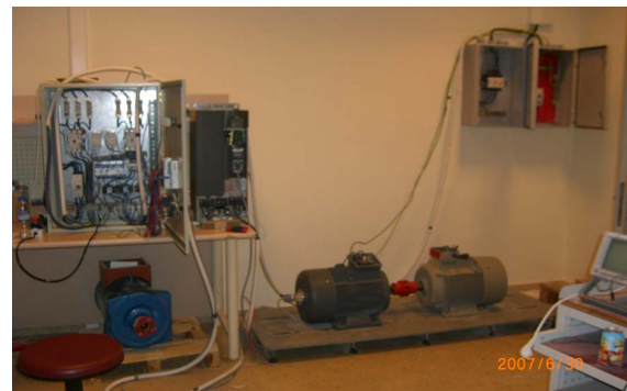
Fig.6. Laboratory test setups, for both generators synchronous (up) and asynchronous (down)
