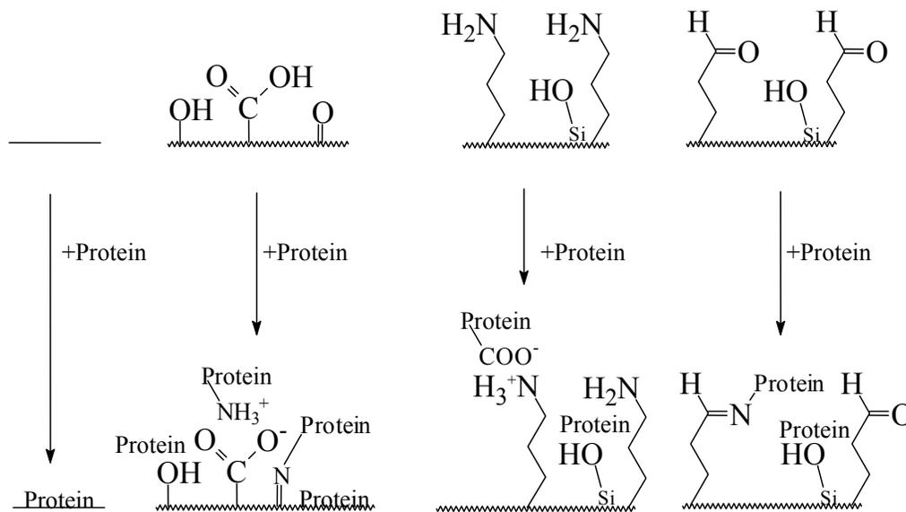
Figure 9. Multiple binding modes for protein retained along engineered surfaces. Surfaces are (A) native polypropylene; (B) oxidized polypropylene; (C) aminopropylsilylated oxidized polypropylene; and (D) aldehyde-transformed oxidized polypropylene.
