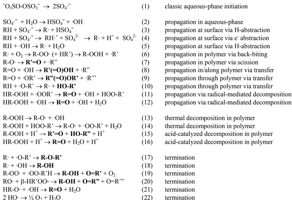
Figure 5. Solution-phase originating oxidation model illustrating alcohol, ketone, carboxylic acid, ester and ether formation in polypropylene (products in bold).
