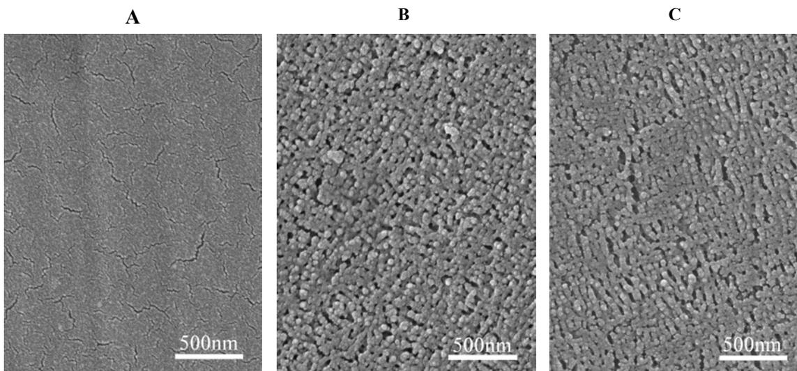
Figure 3. Scanning electron micrographs of gold-coated surfaces of Eppendorf tubes treated 16h with ammonium sulfate (A), persulfate (B) and persulfate followed by the hydrolysis products of aminopropyltriethoxysilane (C).
