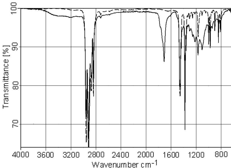
Fig. 2. ATR FT-IR spectrum of vacuum-dried polypropylene samples before (dashed line) and after (solid line) treatment with persulfate solution (1M, 70°C, 16h).
