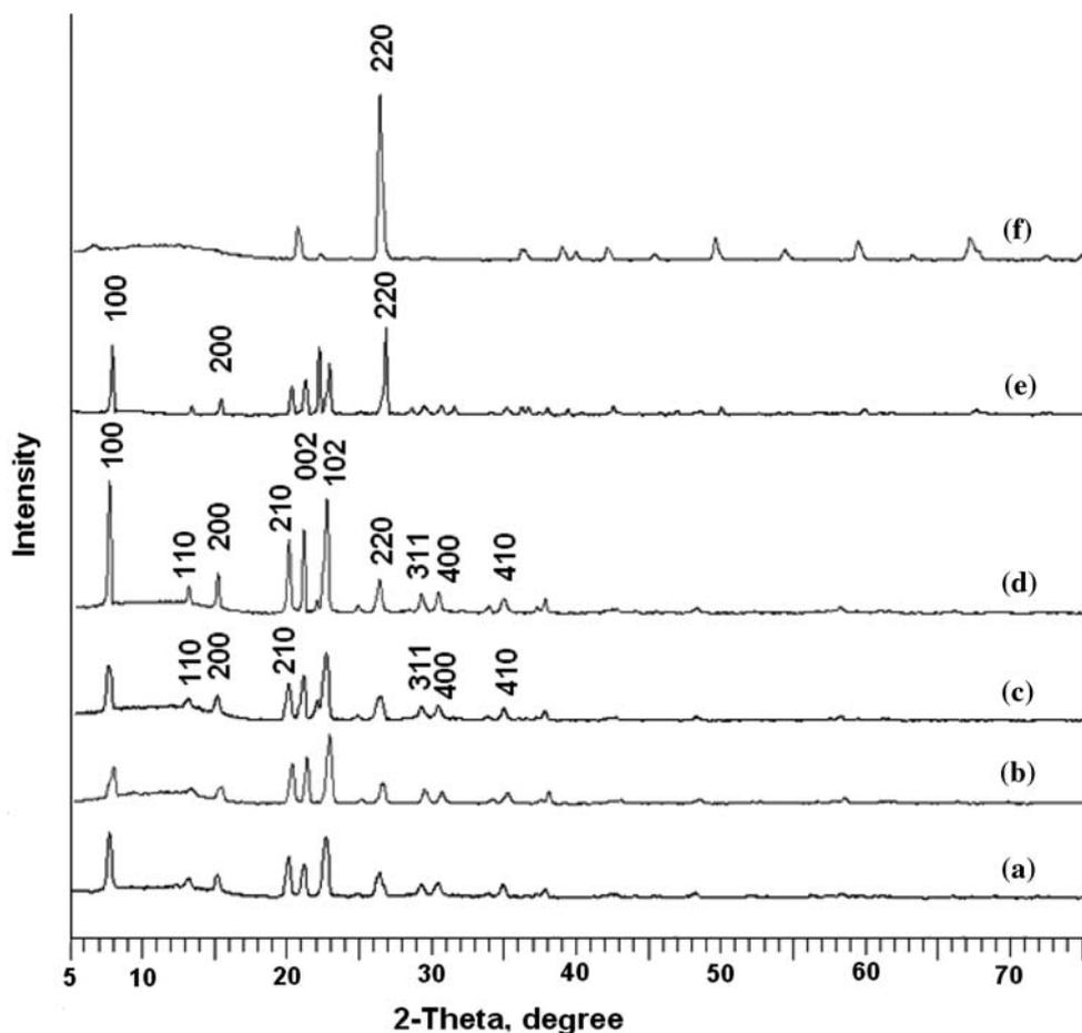
180 to 900 s,  $\text{AlPO}_4\text{-5}$  crystals began to grow longer and aligned in certain angles. XRD patterns of H11, H12 and H13 were shown in Fig. 8, corresponding to the berlinite structure [29].
