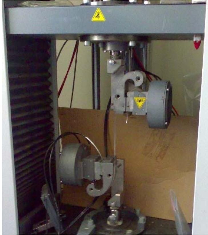
Figure 3.1- Zwick UTM at Cam Elyaf Co. for the testing of fiber bundles
