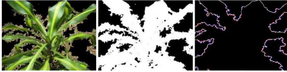
FIGURE 9. Example for a bad (jagged) plant contour caused by inadequate segmentation. Left: Segmented image, Middle: Segmentation map to see the segmentation faults, Right: Traced contour of the image with spurious high-curvature points.
