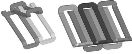
Figure 7. Final coil shape used for the stator.
