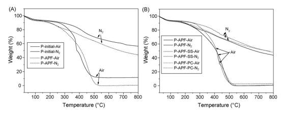
Fig. 3. (A and B) TG curves of "Pirin" coal samples in air and N<sub>2</sub>.
