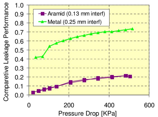
**Fig. 8** Sample Aramid Seal Leakage Data
