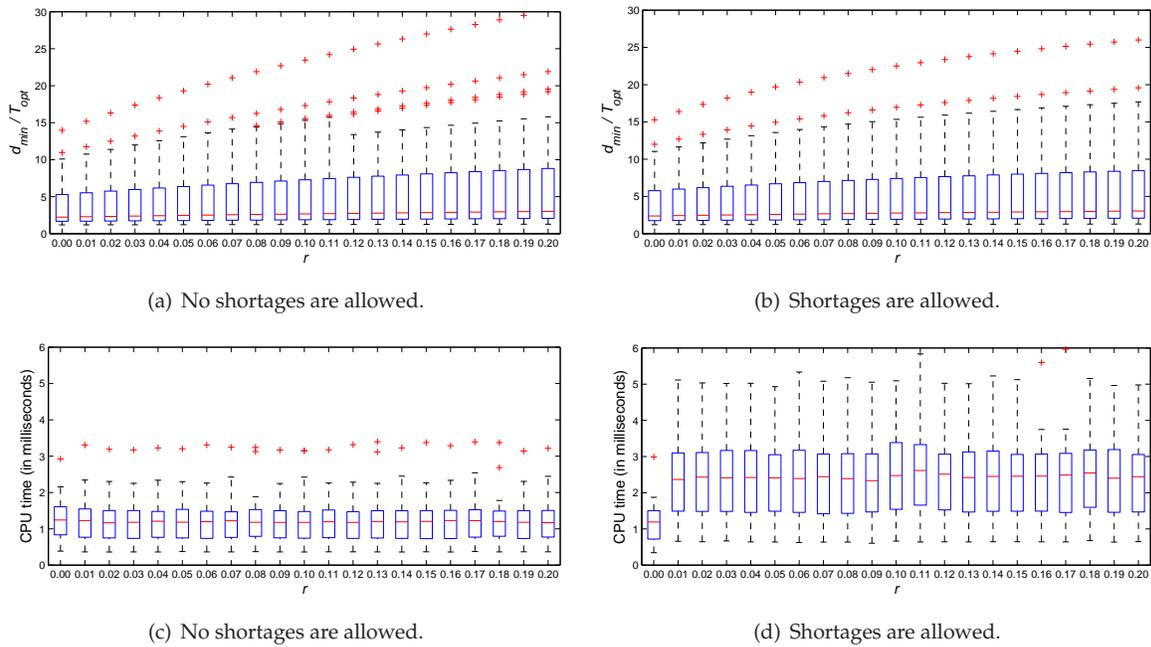
Figure 10: Quality of the upper bound on  $T_{opt}$  for polyhedral concave functions with respect to  $r$  and associated solution times.
