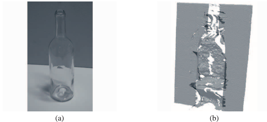
Fig. 1. (a) Transparent glass bottle. (b) 3D reconstruction by Minolta VI-910 Non Contact 3D Digitizer.
