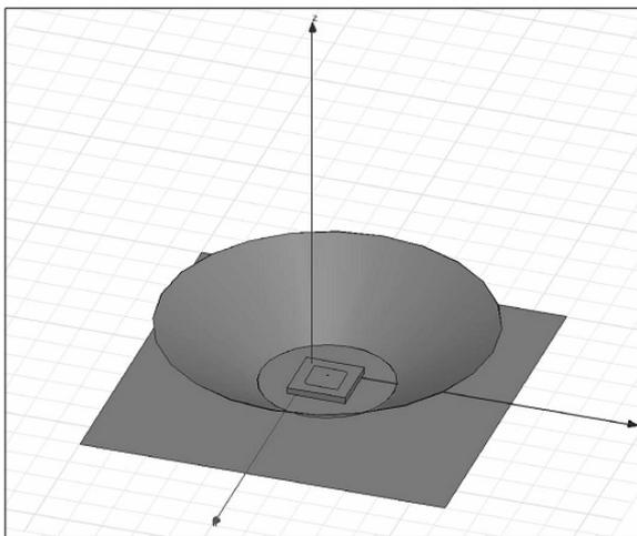
Fig 1 - GPS Patch Antenna with the conical reflector
