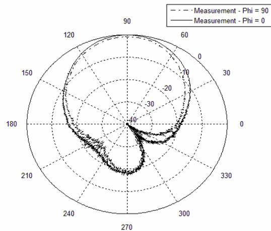
Fig 5 - Measured Radiation Patterns at  $\theta = 0^\circ$  and
