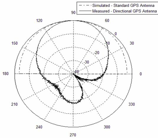
Fig 6 - Measured and Simulated Radiation Patterns
