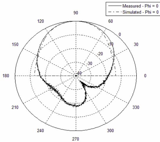
Fig 4 – Measured and Simulated Radiation Patterns
