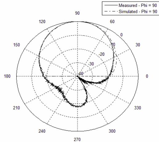
Fig 7 - Measured and Simulated Radiation Patterns
