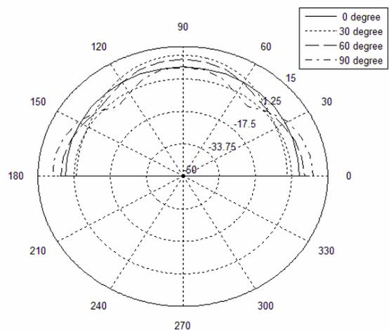
Fig 2 – Radiation Patterns with Different Cone angles
