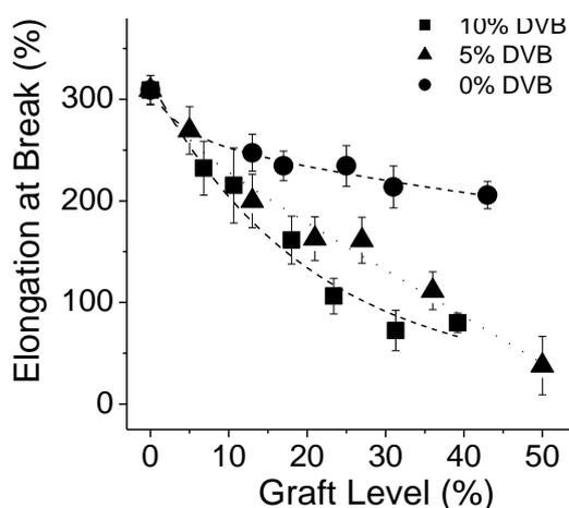
**Figure 8:** Elongation at break of ETFE-g-styrene films (MD) as function of the GL. Grafted films with different DVB concentrations (0, 5, 10 %) in the initial grafting solution.
