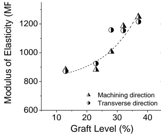
**Figure 9:** Modulus of elasticity of ETFE-*g*-styrene based membranes as function of the GL in the MD and TD.
