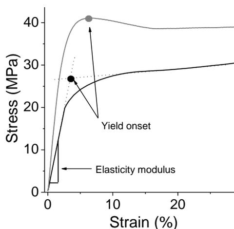
Figure 1: Determination of the modulus of elasticity and the yield onset by the tangents technique.
