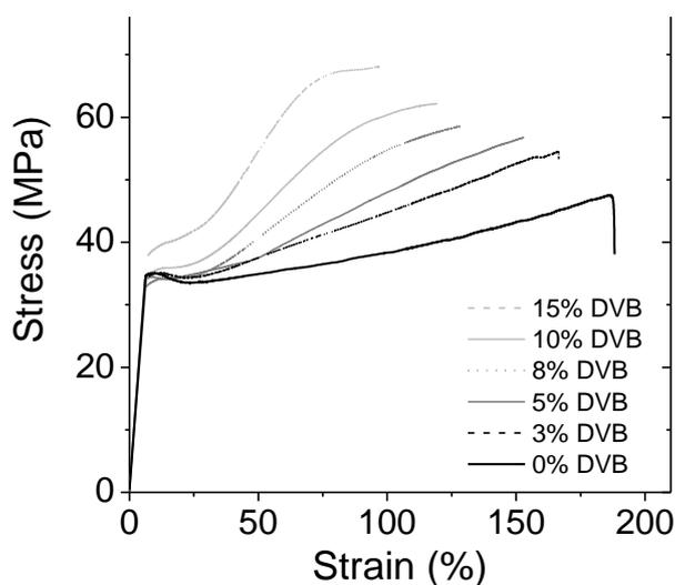
Figure 10: Strain-stress curves of ETFE-g-styrene/DVB films (MD) with different DVB concentration in the initial grafting solution.
