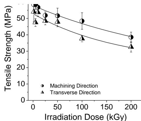
Figure 3: Effect of irradiation dose on tensile strength of the ETFE films in both directions.
