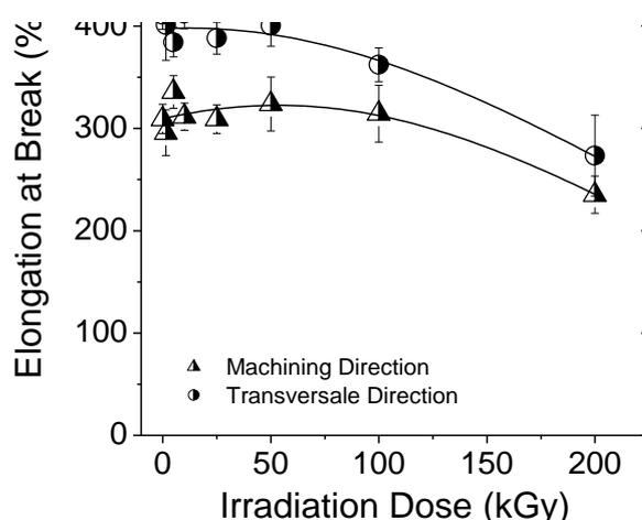
Figure 4: Effect of irradiation dose on elongation at break of ETFE films in both directions.
