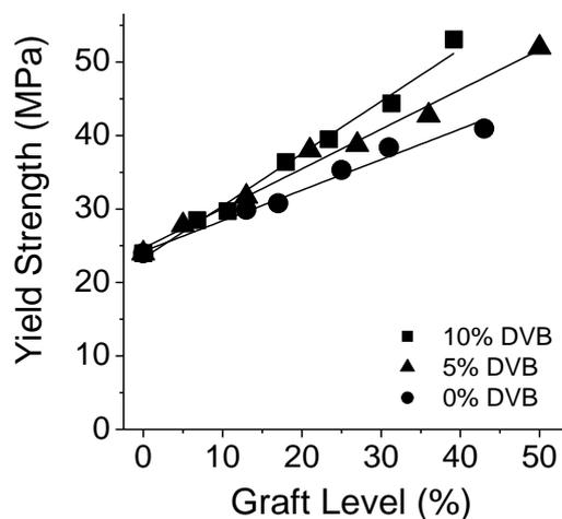
Figure 7: Evolution of the yield strength of ETFE-g-styrene films (MD) as function of the GL. Grafted films with different DVB concentration in the initial grafting solution.
