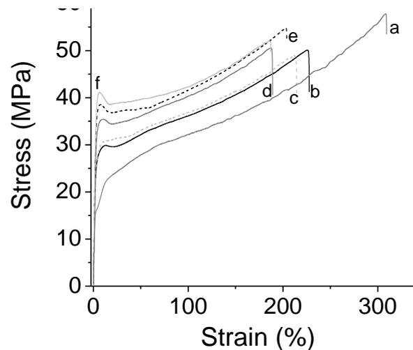
Figure 6: strain-stress curves of ETFE and ETFE-g-styrene films (MD) with different graft levels: (a) ETFE base film, (b) 13%, (c) 17%, (d) 25%, (e) 31%, (f) 44%.
