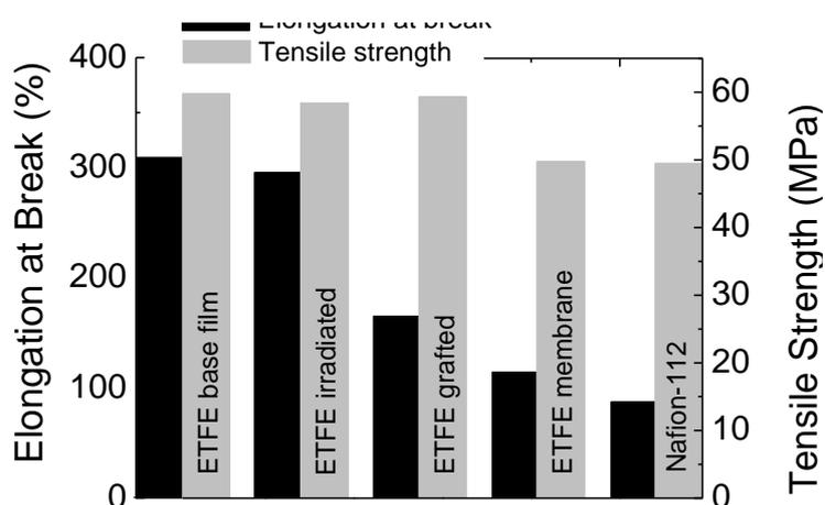
Figure 13: Effect of preparation process (irradiation, grafting and sulfonation) on the elongation at break and tensile strength of ETFE-g-styrene/DVB membrane (5% DVB (v/v) and GL ~ 25 %) in the machining direction. Membranes are exchanged to K<sup>+</sup> form and dried. Nafion®112 membrane is presented for comparison.
