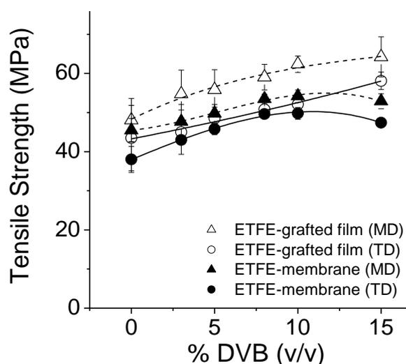
**Figure 11:** Effect of DVB concentration in the initial solution on the tensile strength of ETFE-g-styrene/DVB films and membranes (GL ~ 25%) in both direction (MD and TD).
