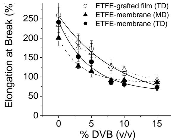
**Figure 12:** Effect of DVB concentration in the initial solution on the elongation at break of ETFE-*g*-styrene/DVB films and membranes in both direction (MD and TD).
