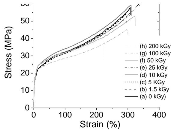
Figure 2: Tensile strain-stress curves of ETFE films for varying irradiation doses in the MD. (a) 0 kGy (unirradiated base film), (b) 1.5 kGy, (c) 5 kGy, (d) 10 kGy, (e) 25 kGy, (f) 50 kGy, (g) 100 kGy, (h) 200 kGy.
