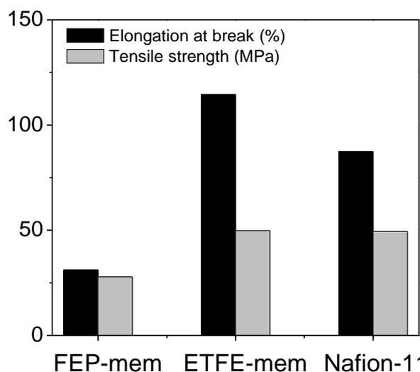
**Figure 14:** Elongation at break and tensile strength of ETFE-*g*-styrene/DVB (5 % DVB (v/v) and GL ~ 25 %), FEP-*g*-styrene/DVB (10 % DVB (v/v) and GL ~ 20 %) and Nafion®112 based membranes in the machining direction. Membranes are exchanged to K<sup>+</sup> form and dried.
