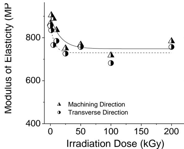
**Figure 5:** Modulus of elasticity of ETFE films as function of the irradiation dose in both directions.
