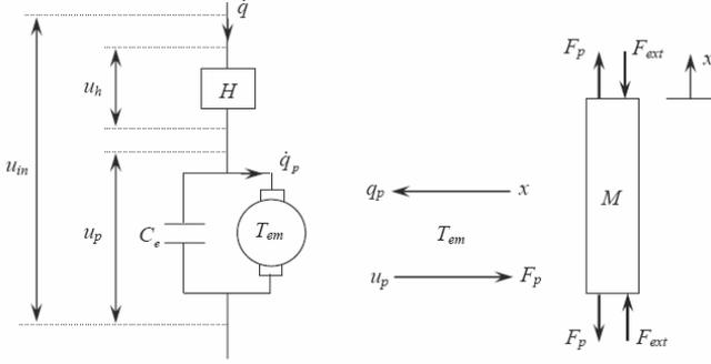
Fig. 1 Electromechanical model of a PZT actuator, [2]
