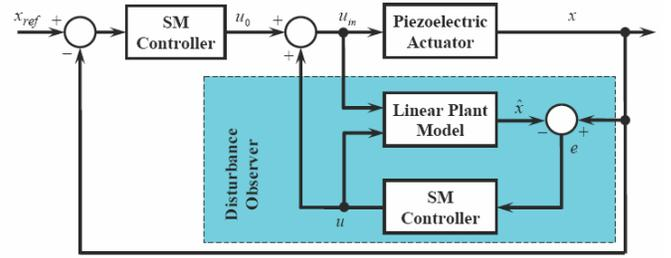
Fig. 3 Simulink Model of the overall system
