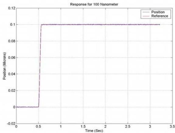
Fig. 7 Step response for 100 Nanometer
