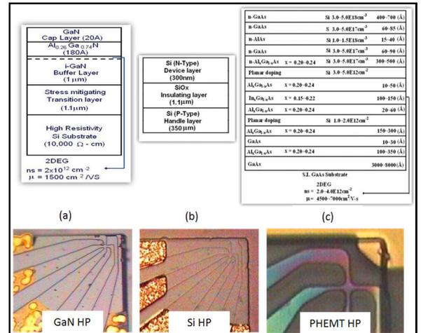
**Fig. 1.** Schematic diagram of the layer configuration of the AlGaIn/GaN heterostructure (a), SOI wafer (b) and PHEMT heterostructure (c) and corresponding photographs of  $1\mu\text{m} \times 1\mu\text{m}$  Hall probes.
