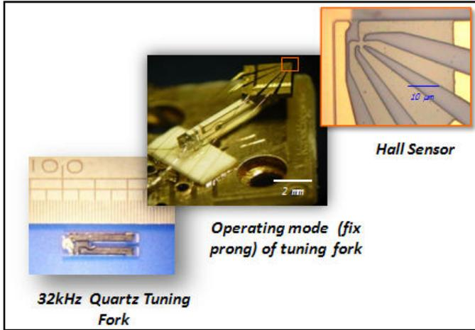
**Fig. 4.** Integration of micro Hall probe with Quartz Tuning fork with Gold wire for electrical contacts. One prong fixed to the base to reduce the noise and improve the resonance properties of the tuning fork [10].
